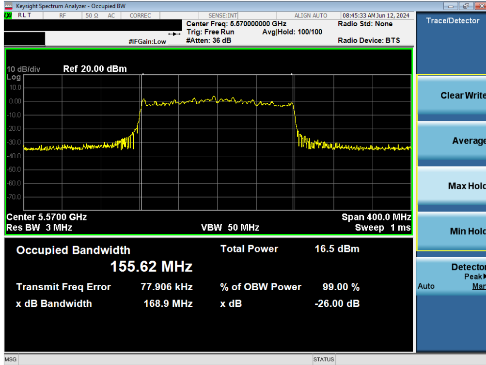
Plot 7-25. 26dB Bandwidth Plot MIMO ANT1 (160MHz BW 802.11ax (UNII Band 2C) – Ch. 114)
