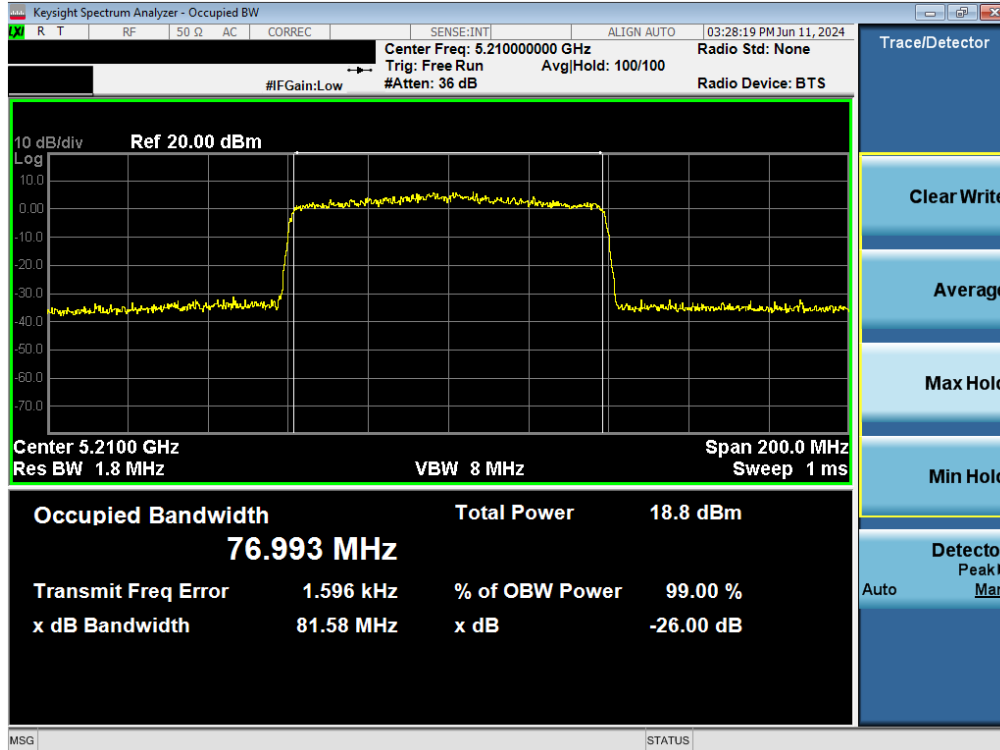
Plot 7-7. 26dB Bandwidth Plot MIMO ANT1 (80MHz BW 802.11ax (UNII Band 1) – Ch. 42)
