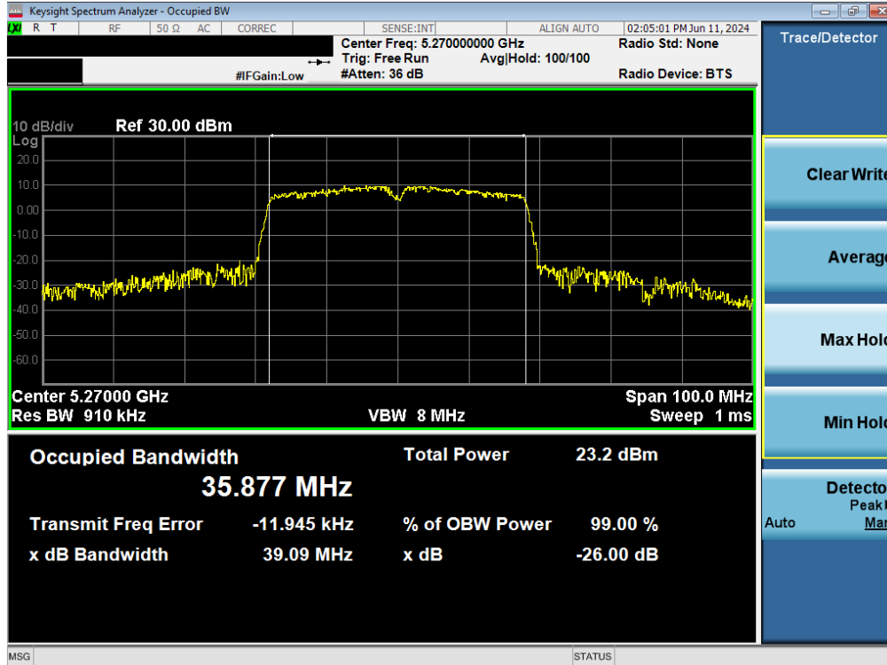
Plot 7-13. 26dB Bandwidth Plot MIMO ANT1 (40MHz BW 802.11n (UNII Band 2A) – Ch. 54)
