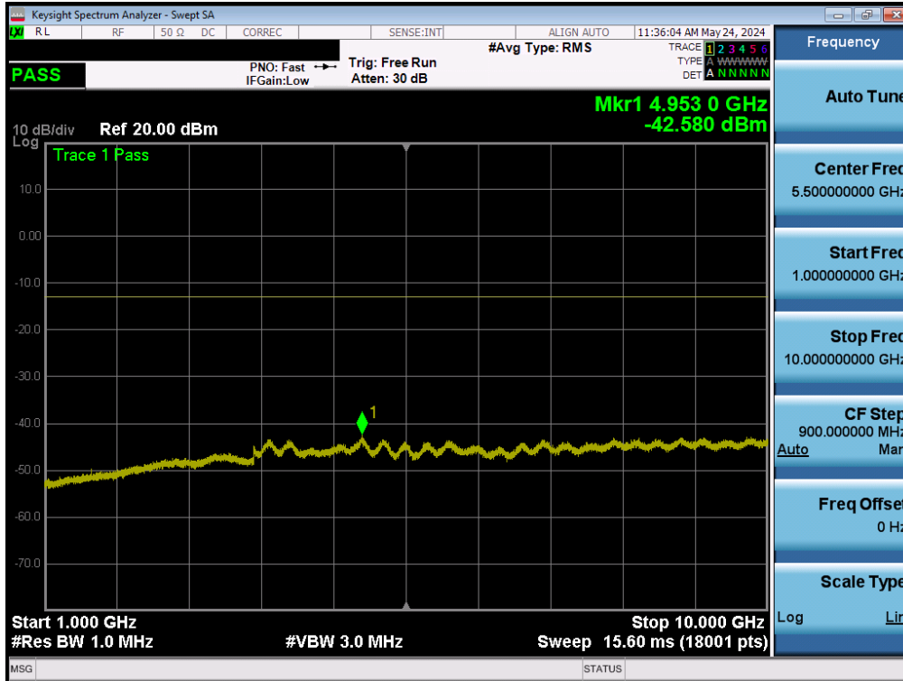
Plot 7-40. Conducted Spurious Plot (LTE Band 14 - 10MHz QPSK - RB Size 1, RB Offset 25)
