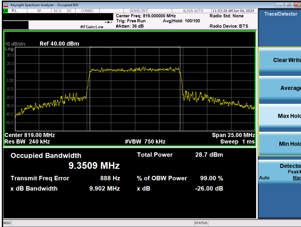
Plot 7-31. Occupied Bandwidth Plot (NR Band n26 - 10MHz 16-QAM - Full RB)
