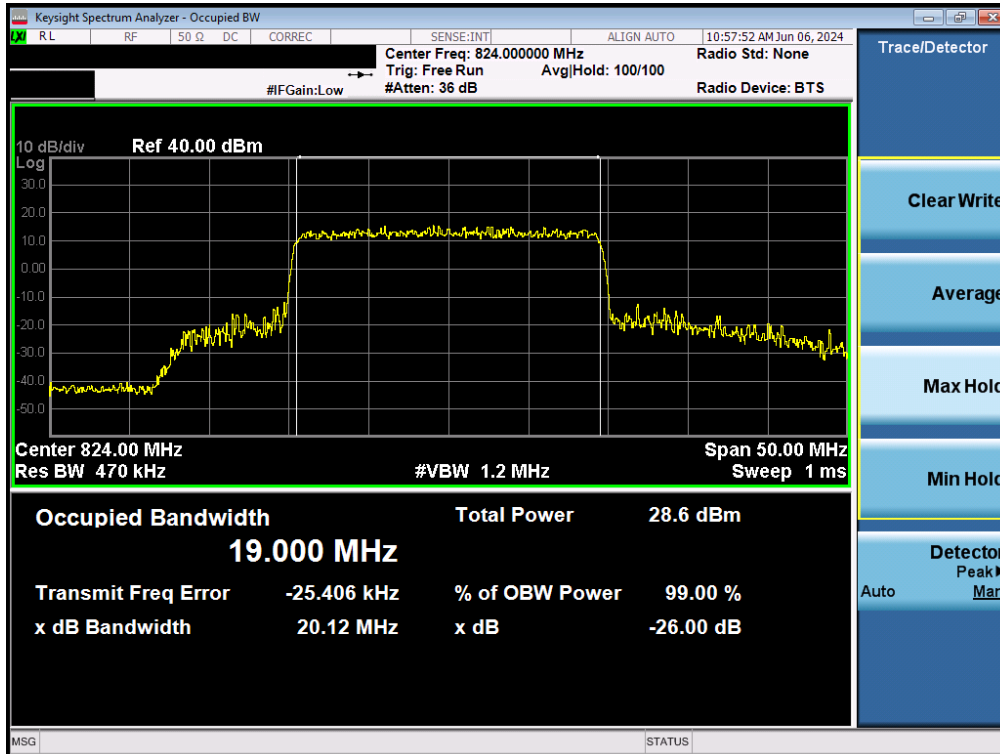
Plot 7-24. Occupied Bandwidth Plot (NR Band n26 - 20MHz QPSK - Full RB)
