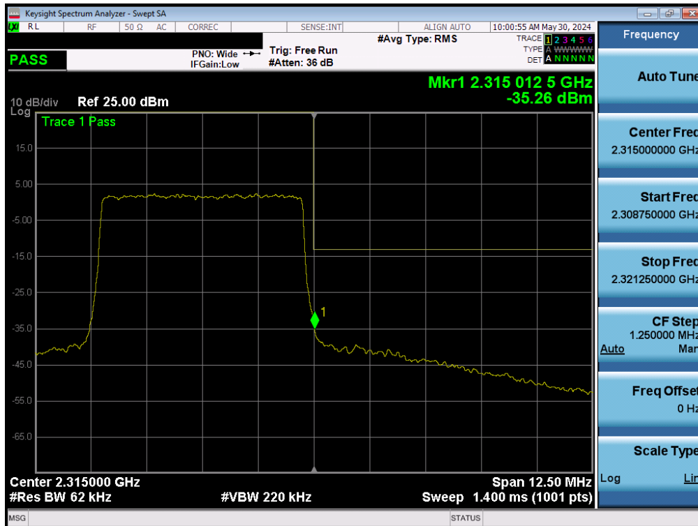
Plot 7-173. Upper Band Edge Plot (NR Band n30 - 5MHz CP-OFDM-QPSK – Full RB)
