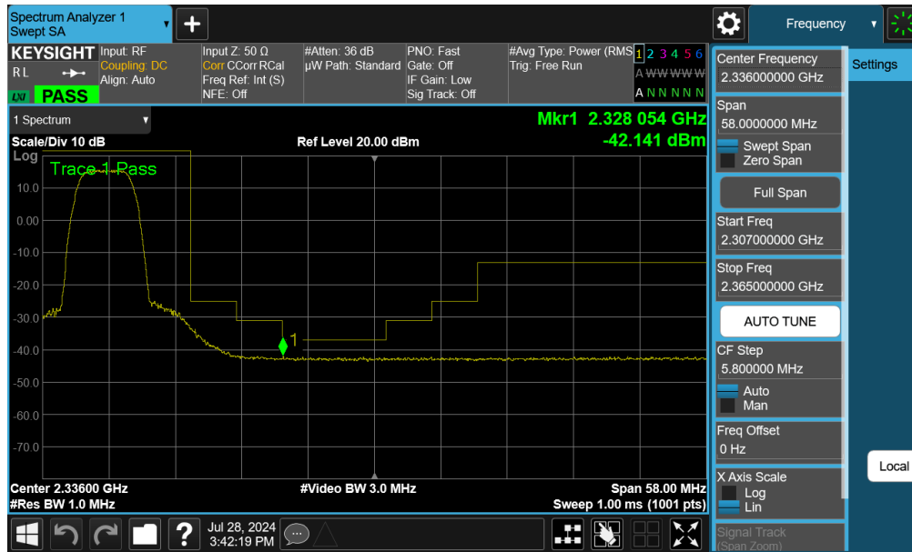
Plot 7-162. Extended Upper Band Edge Plot (LTE Band 30 - 5MHz QPSK – Full RB)
