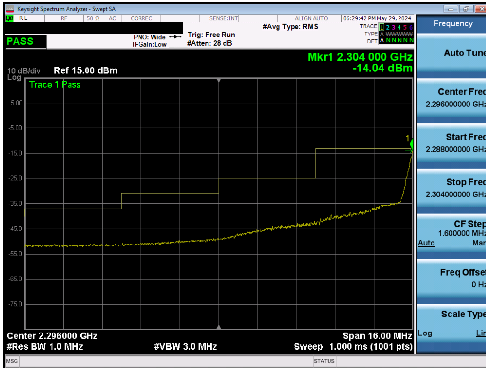
Plot 7-172. Extended Lower Band Edge Plot (NR Band n30 - 5MHz DFT-s-OFDM-BPSK – Full RB)
