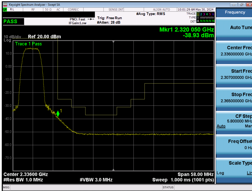
Plot 7-174. Extended Upper Band Edge Plot (NR Band n30 - 5MHz CP-OFDM-QPSK - Full RB)
