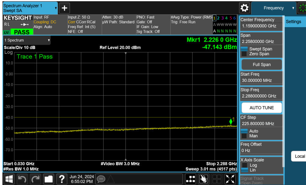
Plot 7-118. Conducted Spurious Plot (LTE Band 30 - 10MHz QPSK - RB Size 1, RB Offset 0)
