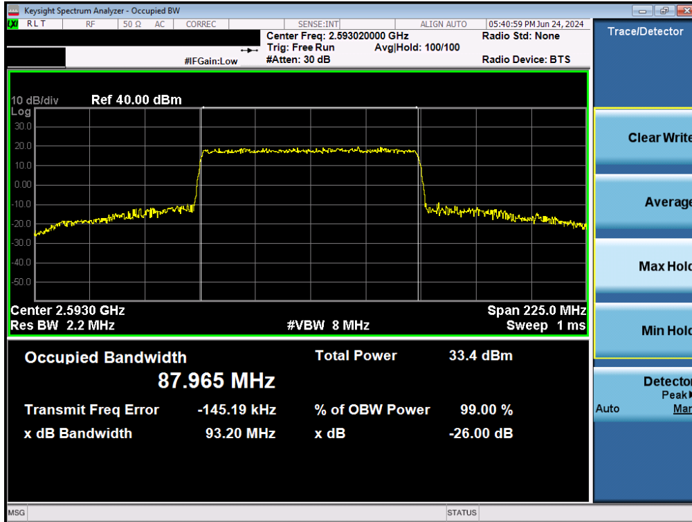
Plot 7-80. Occupied Bandwidth Plot (NR Band n41 - 90MHz QPSK - Full RB)
