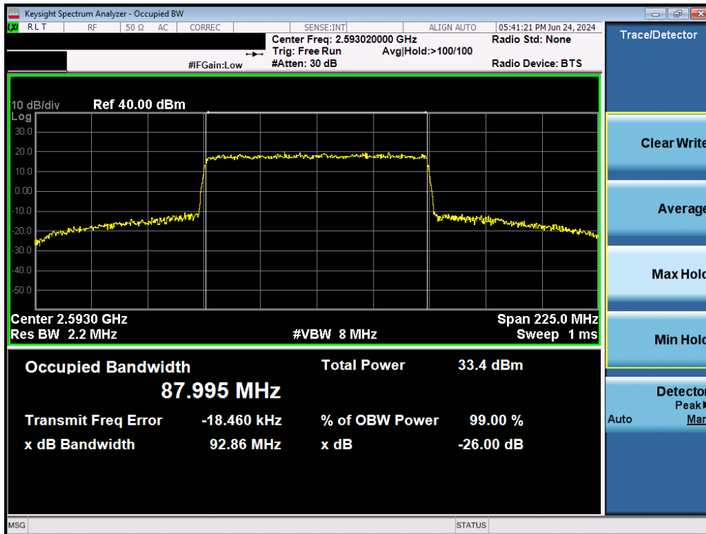
Plot 7-81. Occupied Bandwidth Plot (NR Band n41 - 90MHz 16-QAM - Full RB)
