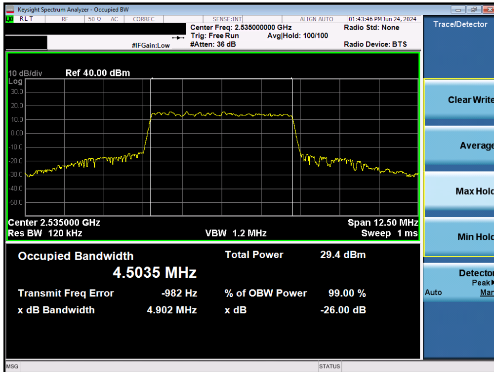
Plot 7-75. Occupied Bandwidth Plot (NR Band n7 - 5MHz 16-QAM - Full RB)
