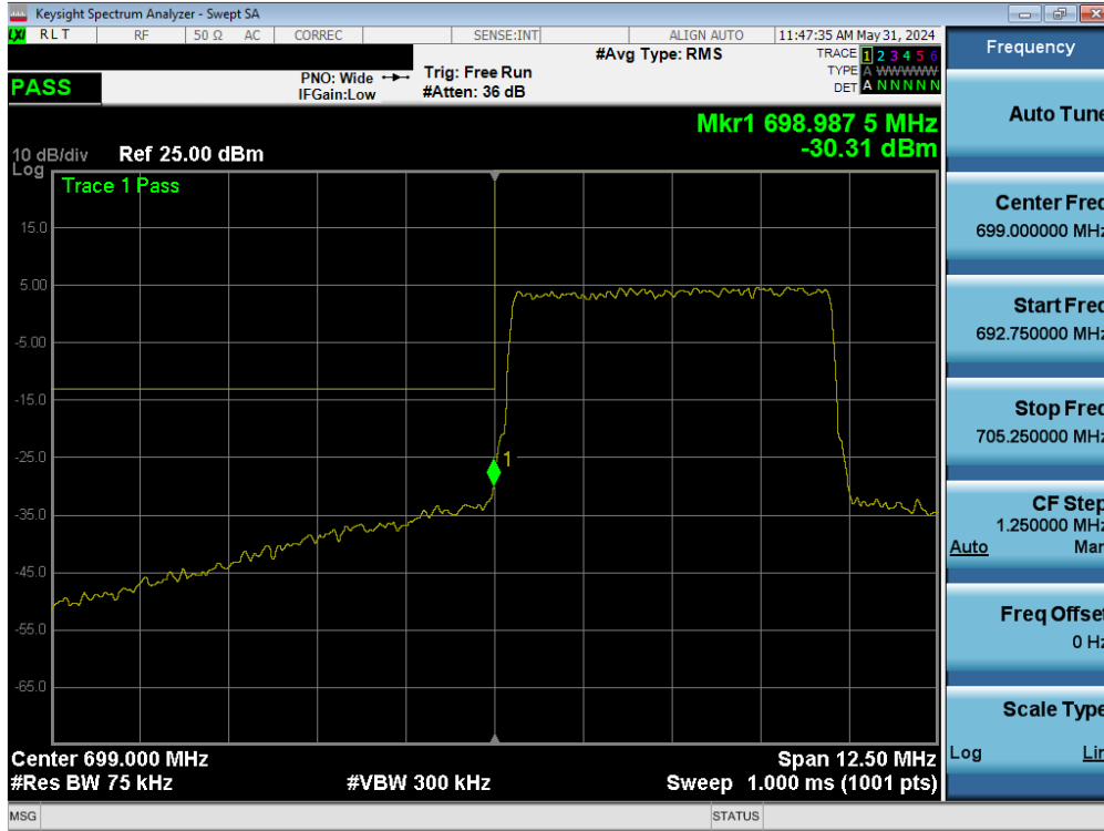
Plot 7-158. Lower Band Edge Plot (NR Band n12 – 5.0MHz - Full RB - ANT1)
