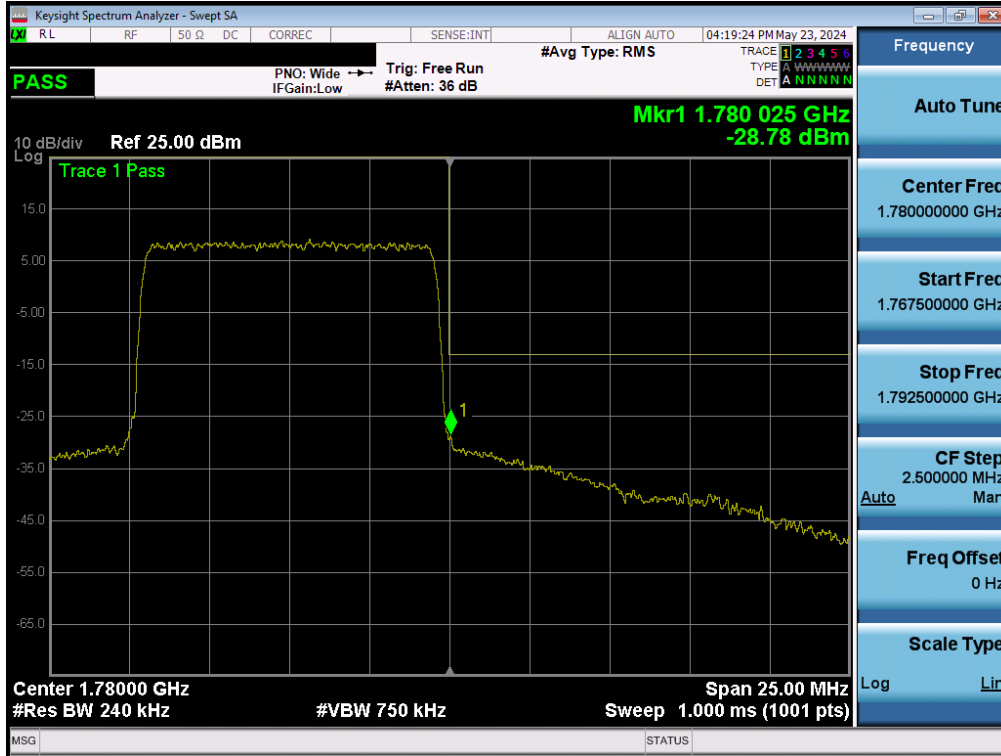
Plot 7-150. Upper Band Edge Plot (LTE Band 66 - 10MHz QPSK - Full RB - ANT1)
