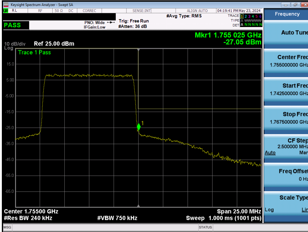
Plot 7-148. Upper Band Edge Plot (LTE Band 4 - 10MHz QPSK – Full RB - ANT1)
