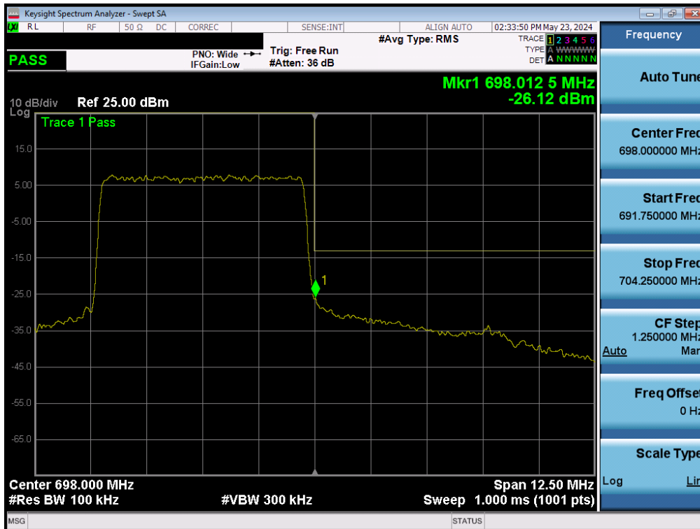
Plot 7-139. Upper Band Edge Plot (LTE Band 71 - 5MHz QPSK – Full RB - ANT1)
