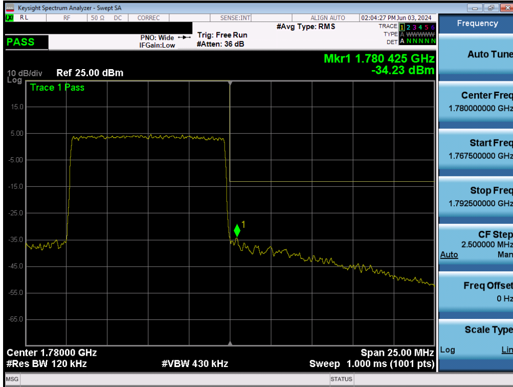
Plot 7-166. Upper Band Edge Plot (NR Band n66 – 10.0MHz - Full RB - ANT1)
