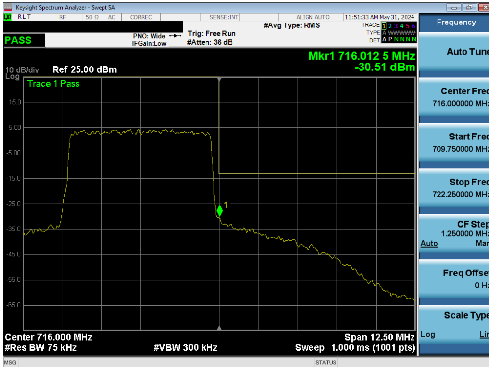
Plot 7-159. Upper Band Edge Plot (NR Band n12 – 5.0MHz - Full RB - ANT1)
