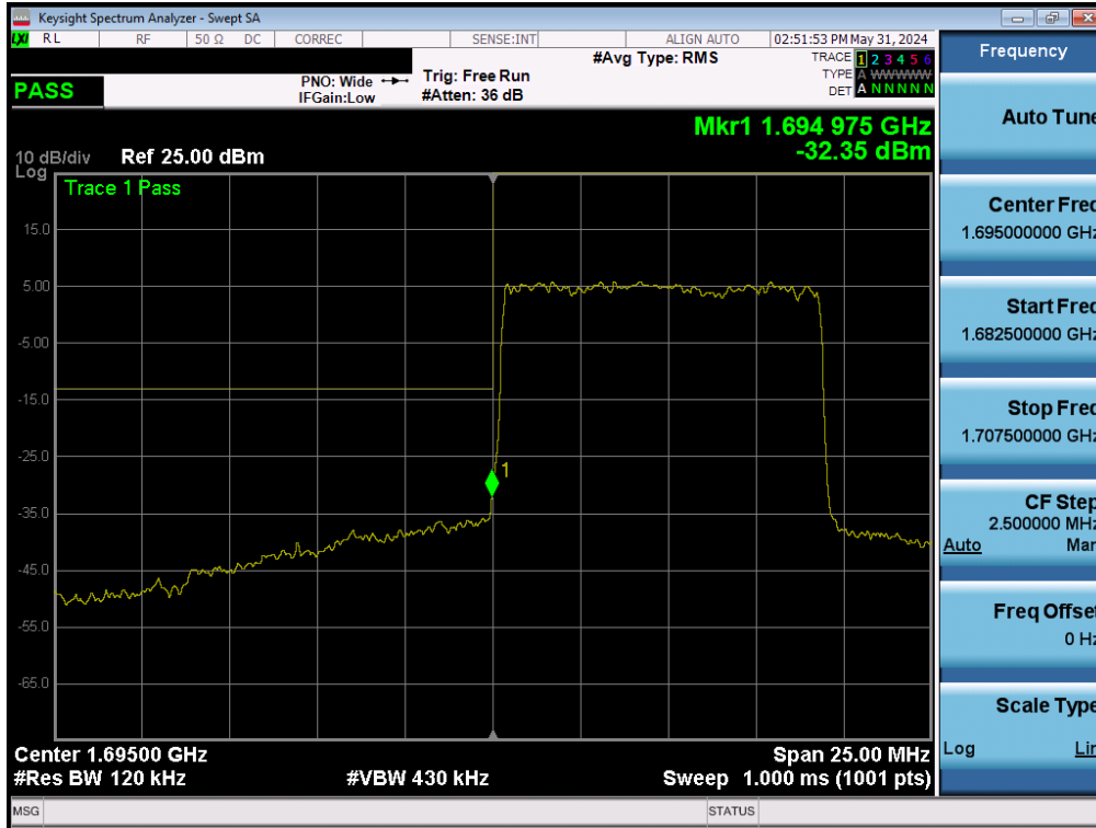
Plot 7-160. Lower Band Edge Plot (NR Band n70 – 10.0MHz - Full RB - ANT1)
