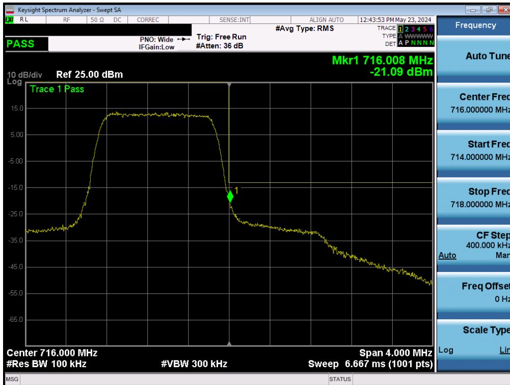
Plot 7-141. Upper Band Edge Plot (LTE Band 12 – 1.4MHz QPSK – Full RB - ANT1)
