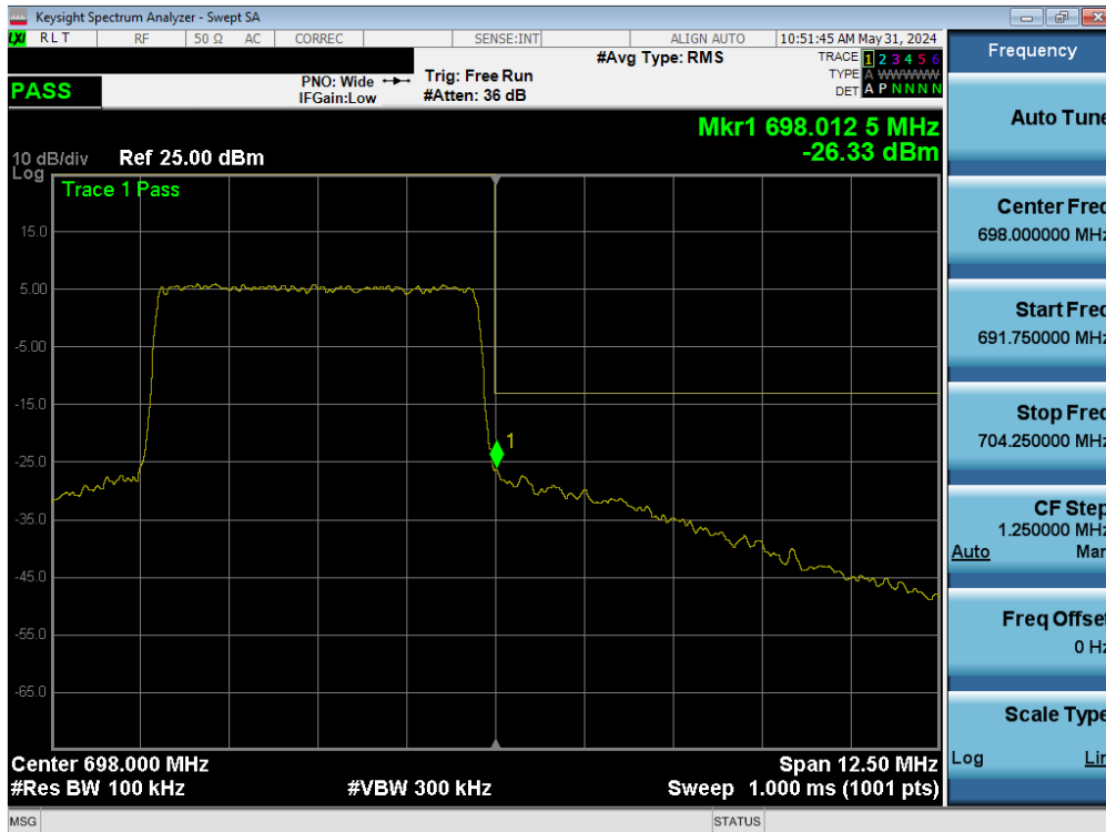
Plot 7-157. Upper Band Edge Plot (NR Band n71 – 5.0MHz - Full RB - ANT1)
