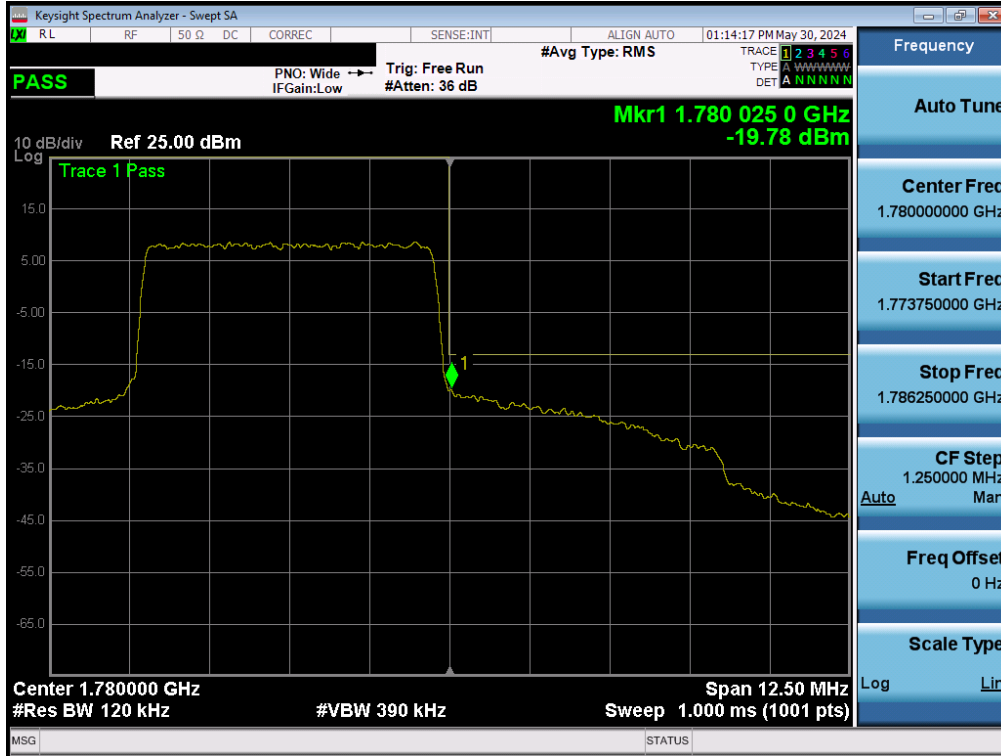
Plot 7-172. Upper Band Edge Plot (LTE Band 66 - 5MHz QPSK – Full RB - ANT2)
