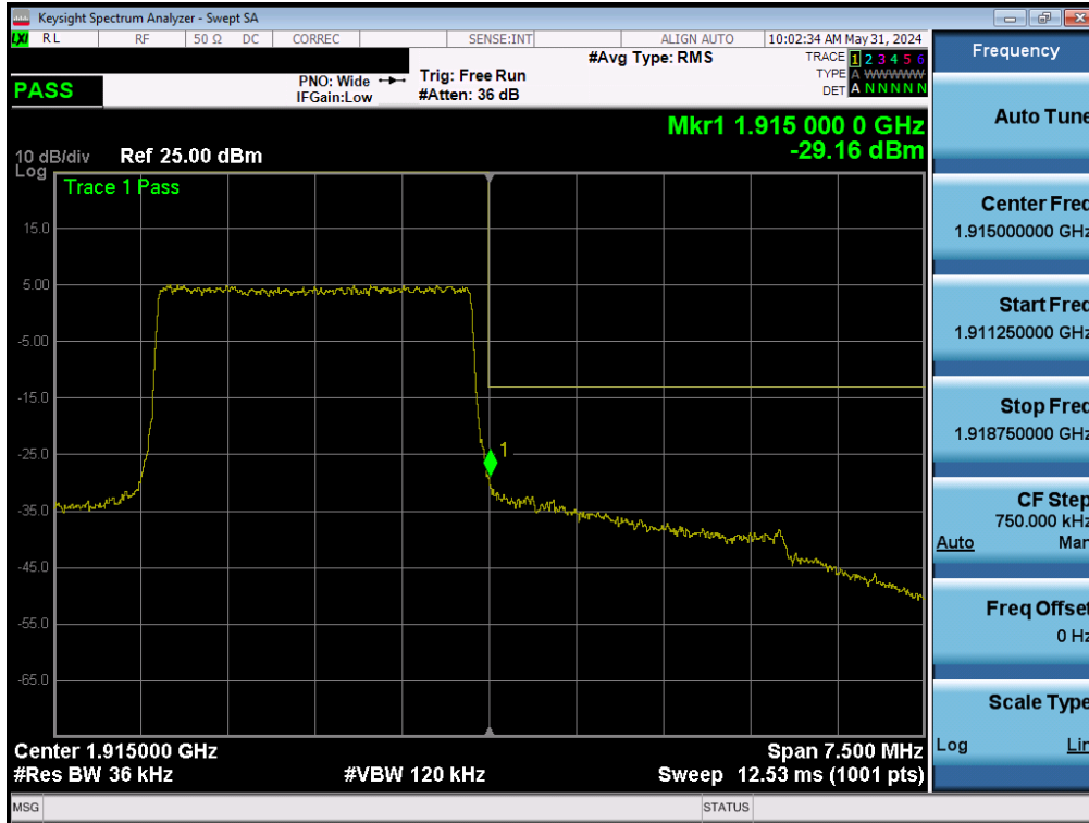
Plot 7-76. Upper Band Edge Plot (LTE Band 25 - 3MHz QPSK – Full RB - Ant2)
