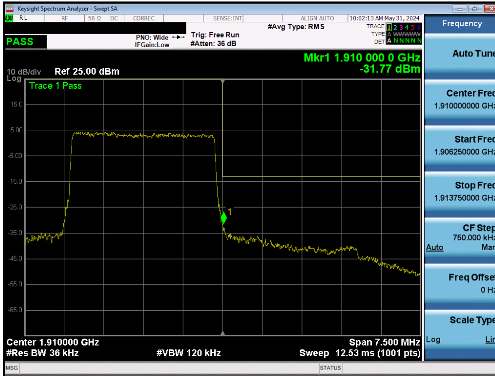
Plot 7-74. Upper Band Edge Plot (LTE Band 2 - 3MHz QPSK – Full RB - Ant2)
