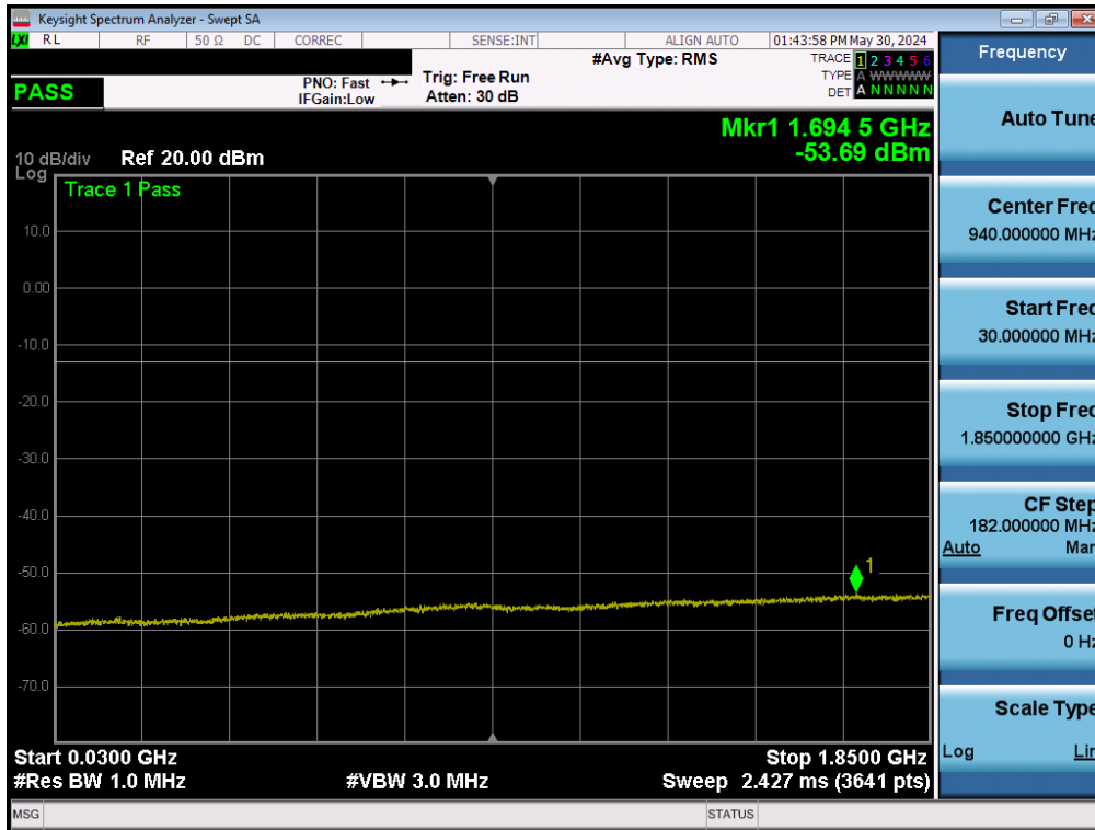
Plot 7-56. Conducted Spurious Plot (LTE Band 25/2 - 20MHz QPSK - 1RB - High Channel - Ant2)
