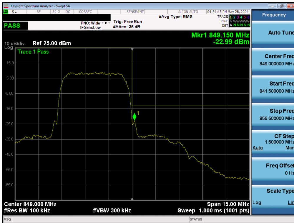
Plot 7-34. Upper Band Edge Plot (WCDMA Cell – Ch. 4233)
