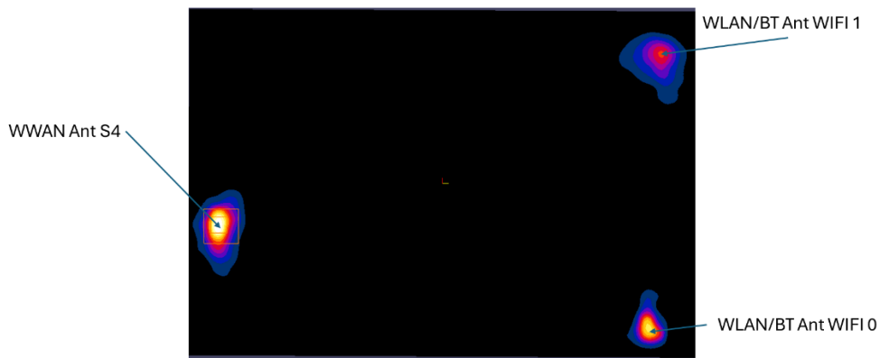
Figure E-2 Tablet Back Side Antenna S4 SAR to Peak Location Separation Ratio Plot
