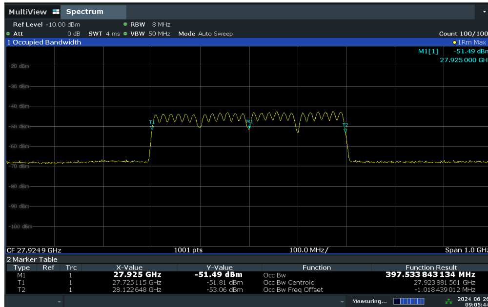
Plot 7-87. Occupied Bandwidth Plot (100MHz-4CC – CP-OFDM 16QAM – Mid Channel)
