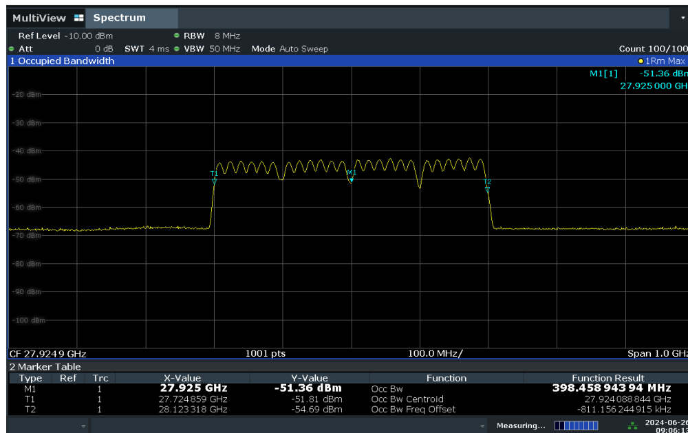
Plot 7-88. Occupied Bandwidth Plot (100MHz-4CC – CP-OFDM 64QAM – Mid Channel)
