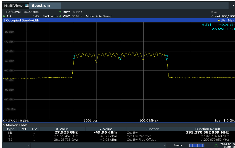
Plot 7-85. Occupied Bandwidth Plot (100MHz-4CC – CP-OFDM QPSK – Mid Channel)
