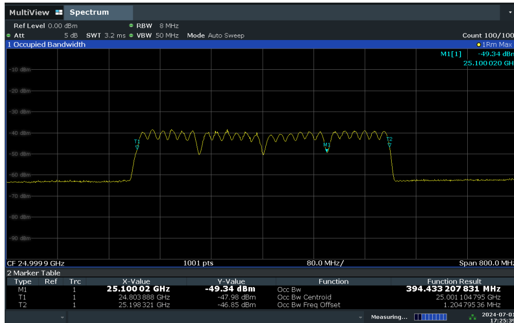
Plot 7-53. Occupied Bandwidth Plot (100MHz-4CC – CP-OFDM QPSK – Mid Channel)
