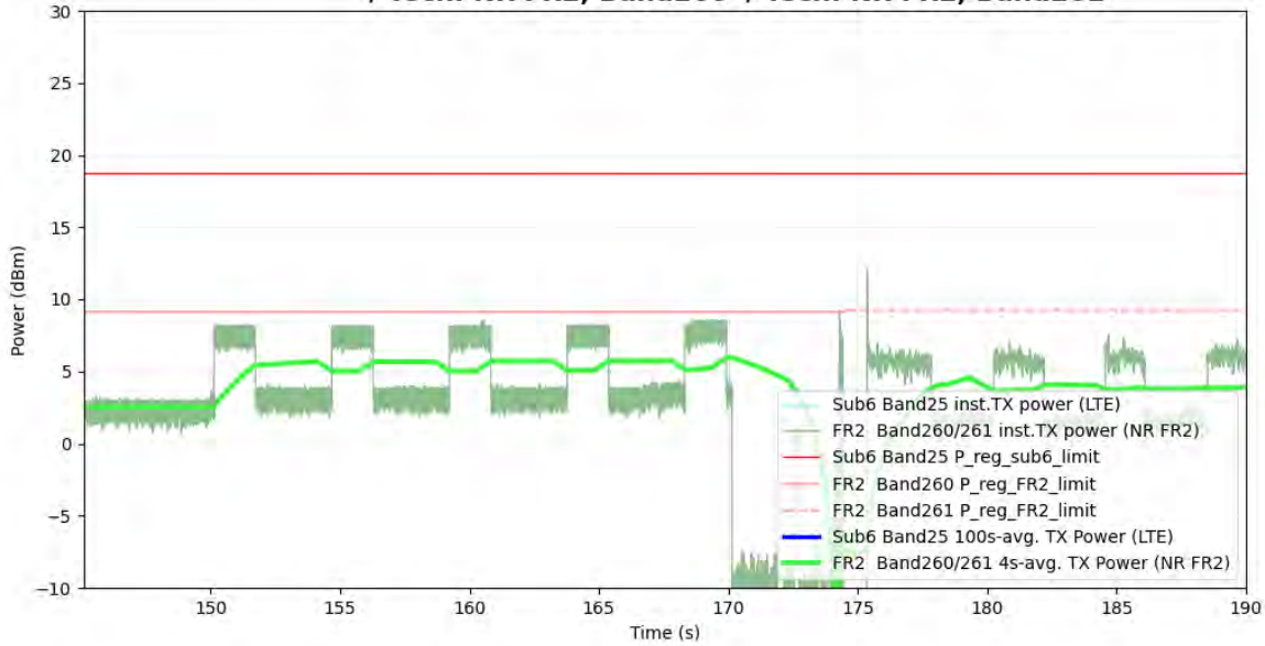
Figure 6-14 LTE, mmW inst. Pwr and Time-averaged Tx Pwr (case 4.1)
