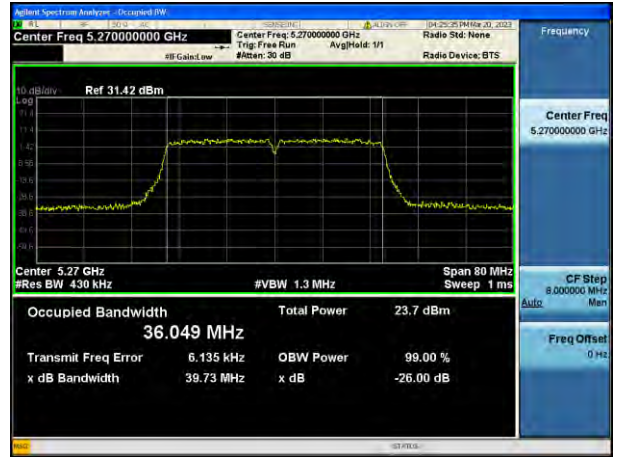
802.11n_HT40 UNII 3 BAND 26 dB Bandwidth (CH 159)
