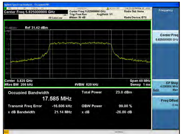
802.11n_HT20 UNII 3 BAND 26 dB Bandwidth(CH 165)
