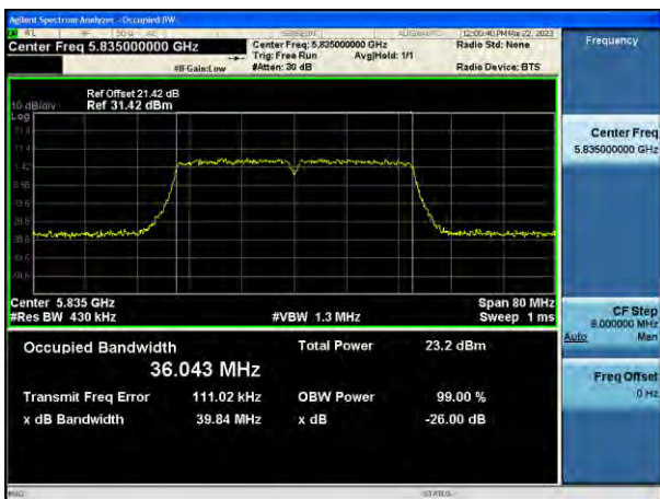
802.11ac_VHT40 UNII 4 BAND 26 dB Bandwidth (CH 167)
