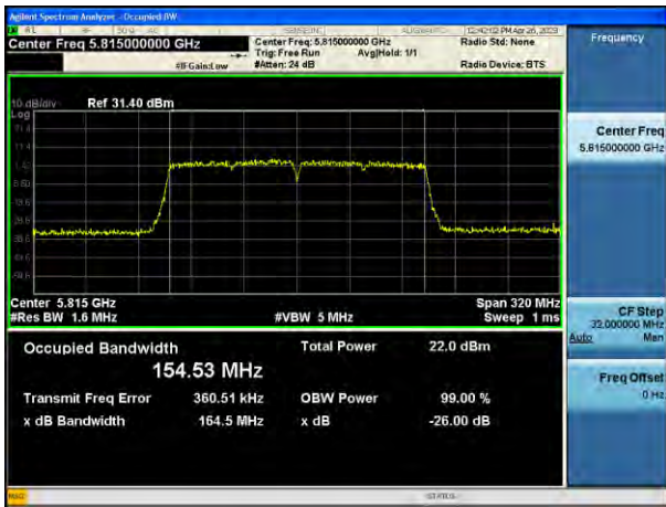
802.11ac_VHT160 UNII 4 BAND 26 dB Bandwidth(CH 163)
