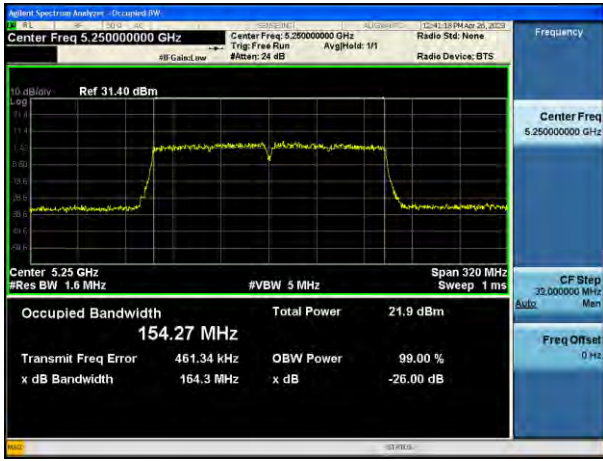
802.11ac_VHT160 UNII 4 BAND 26 dB Bandwidth(CH 163)
