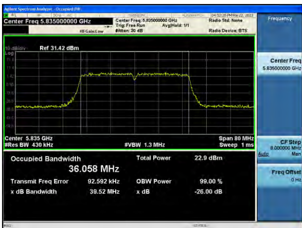
802.11n_HT40 UNII 4 BAND 26 dB Bandwidth (CH 167)
