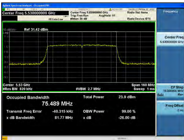
802.11ac_VHT80 UNII 4 BAND 26 dB Bandwidth (CH 171)
