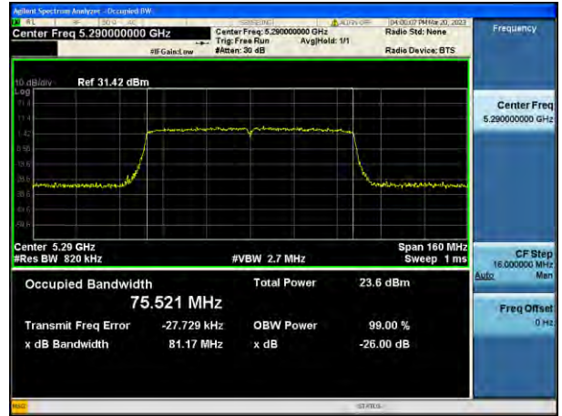
802.11ac_VHT80 UNII 3 BAND 26 dB Bandwidth (CH 155)
