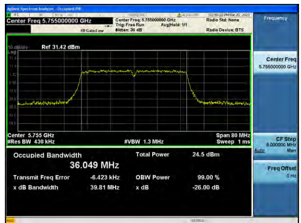
802.11ac_VHT40 UNII 3 BAND 26 dB Bandwidth (CH 151)
