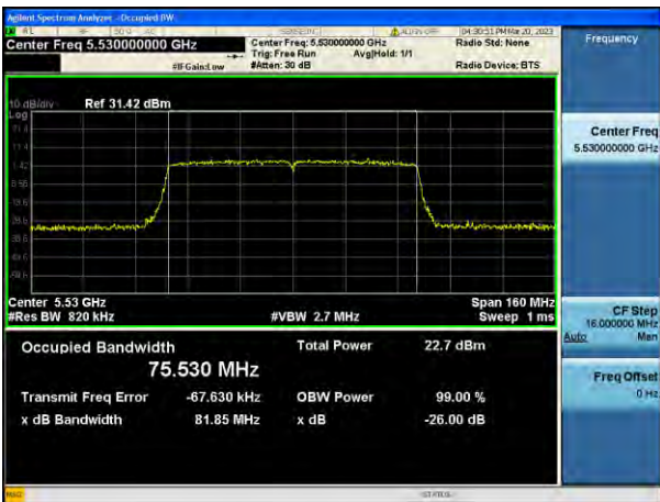
802.11ac_VHT80 UNII 4 BAND 26 dB Bandwidth (CH 171)
