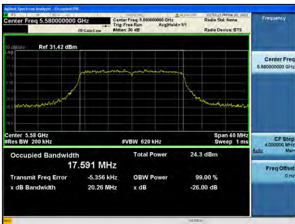
802.11ac_VHT20 UNII 4 BAND 26 dB Bandwidth(CH 173)
