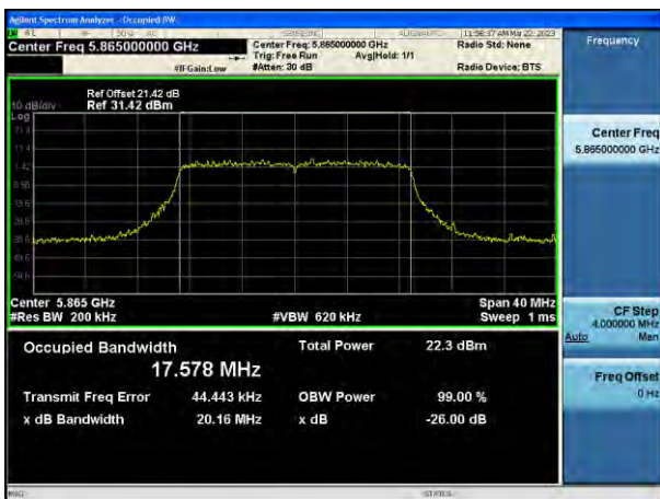
802.11n_HT20 UNII 4 BAND 26 dB Bandwidth(CH 173)
