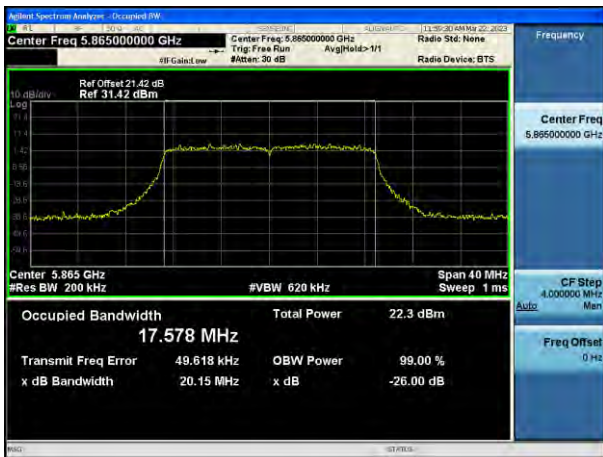
802.11ac_VHT20 UNII 4 BAND 26 dB Bandwidth(CH 173)
