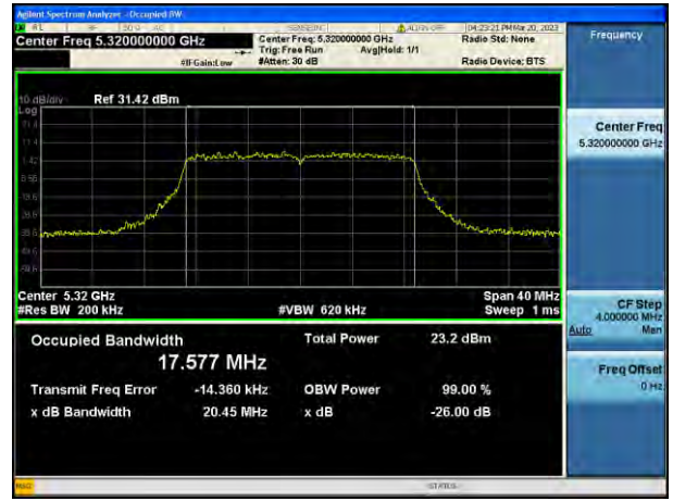
802.11ac_VHT20 UNII 3 BAND 26 dB Bandwidth(CH 165)
