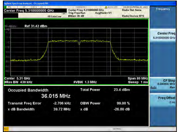
802.11ac_VHT40 UNII 3 BAND 26 dB Bandwidth (CH 159)
