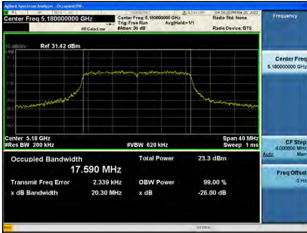
802.11n_HT20 UNII 2C BAND 26 dB Bandwidth(CH 144)
