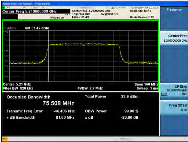
802.11ac_VHT80 UNII 2C BAND 26 dB Bandwidth(CH 106)
