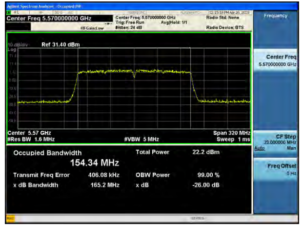
802.11ac_VHT160 UNII 2A BAND 26 dB Bandwidth (CH 114)
