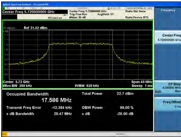
802.11ac_VHT20 UNII 4 BAND 26 dB Bandwidth(CH 169)
