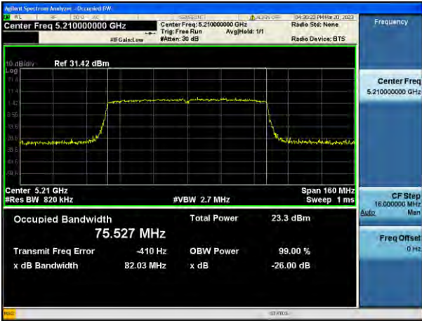
802.11ac_VHT80 UNII 2C BAND 26 dB Bandwidth(CH 106)
