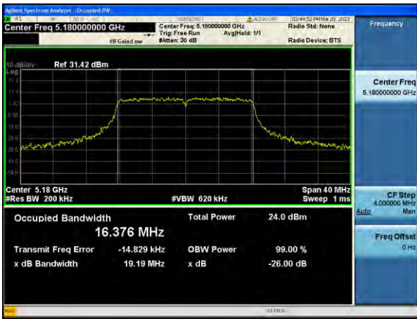
802.11a UNII 2C BAND 26 dB Bandwidth (CH 116)
