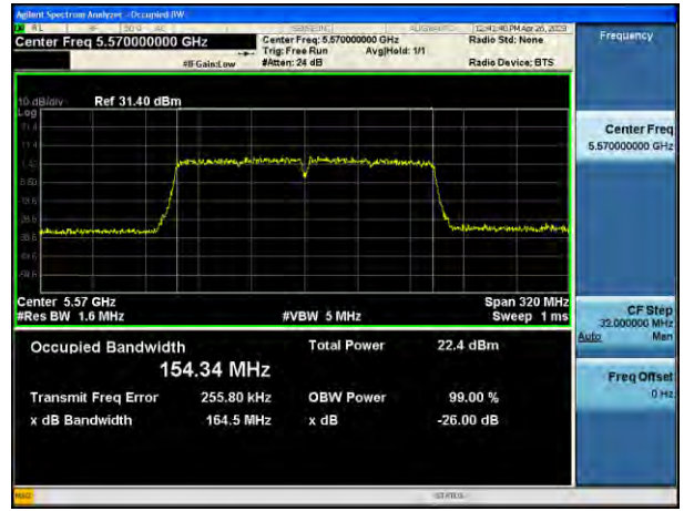
802.11ac_VHT160 UNII 2A BAND 26 dB Bandwidth (CH 114)
