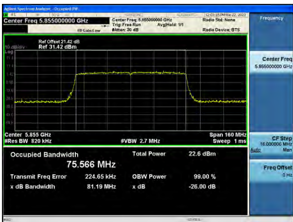
802.11ac_VHT80 UNII 4 BAND 26 dB Bandwidth (CH 171)
