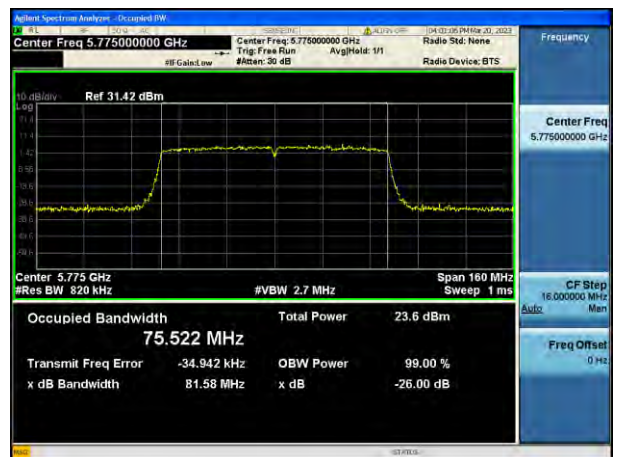
802.11ac_VHT80 UNII 3 BAND 26 dB Bandwidth (CH 155)
