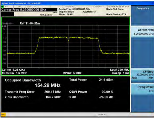
802.11ac_VHT160 UNII 4 BAND 26 dB Bandwidth(CH 163)
