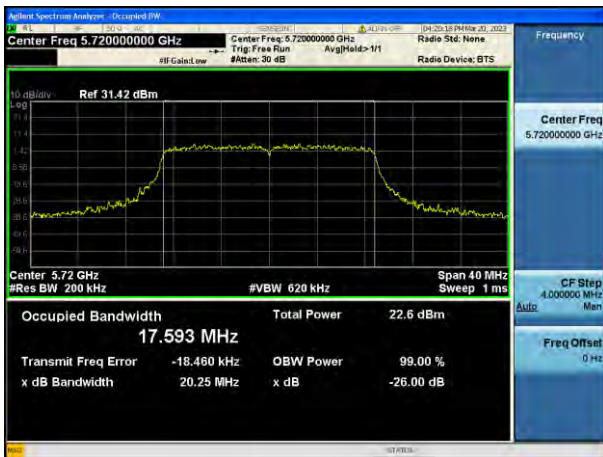
802.11n_HT20 UNII 4 BAND 26 dB Bandwidth(CH 177)
