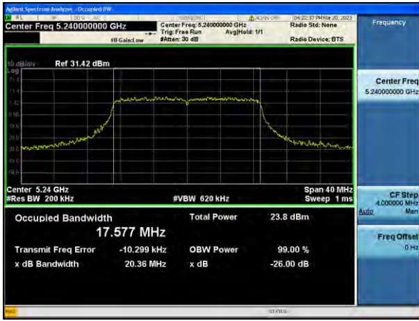
802.11ac_VHT20 UNII 2C BAND 26 dB Bandwidth(CH 144)
