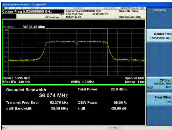
802.11ac_VHT40 UNII 4 BAND 26 dB Bandwidth (CH 167)
