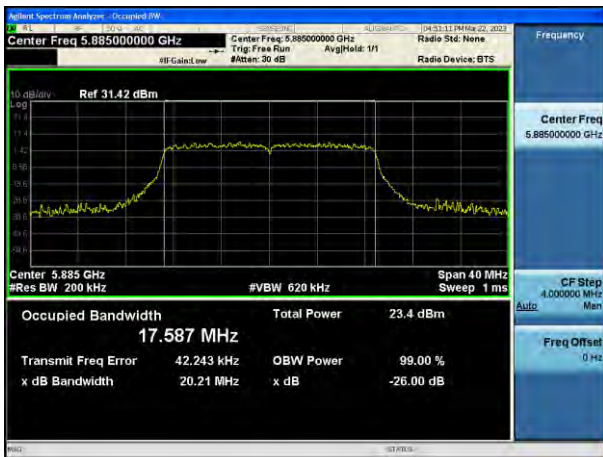
802.11n_HT20 UNII 4 BAND 26 dB Bandwidth(CH 177)
