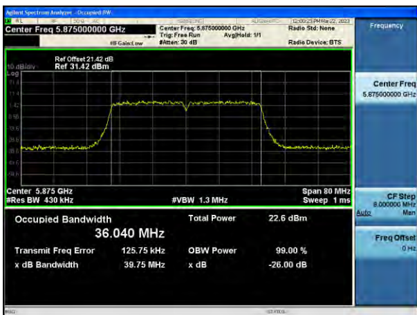
802.11n_HT40 UNII 4 BAND 26 dB Bandwidth (CH 175)
