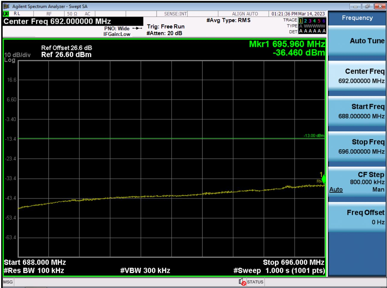
BAND 12. Upper Band Edge Plot (1.4 M BW Ch.23173 QPSK\_RB1\_Offset 5)\_1
