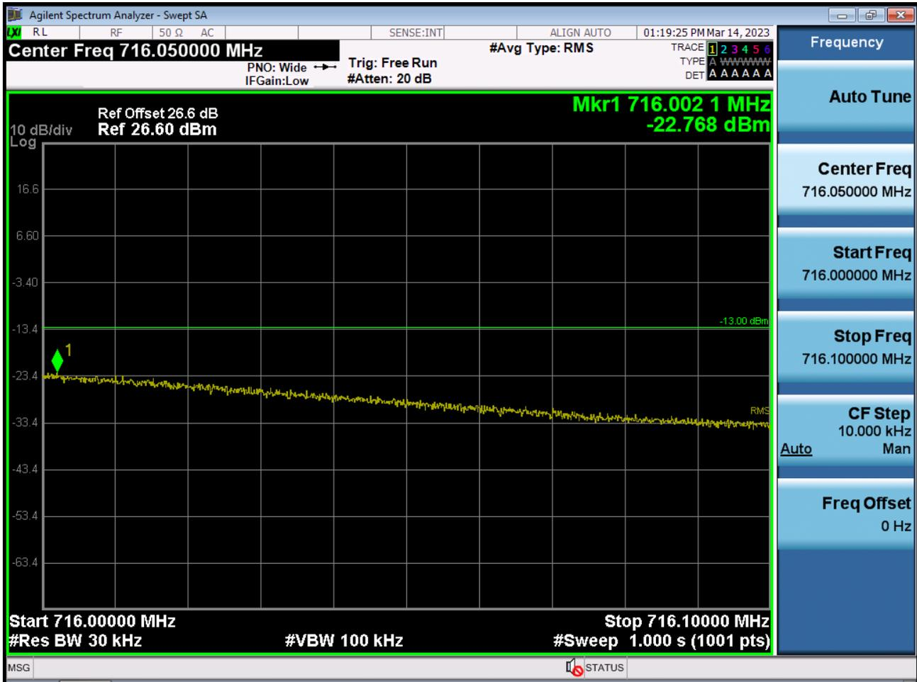
BAND 12. Upper Band Edge Plot (5 M BW Ch.23155 QPSK\_RB1\_Offset 24)\_2
