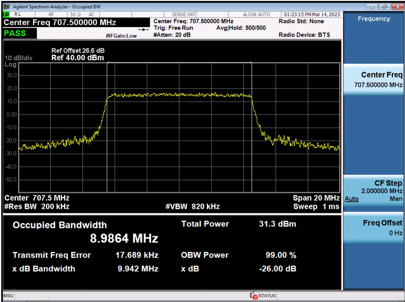
BAND 12. Occupied Bandwidth Plot (10 M BW Ch.23095 64QAM\_RB50\_0)
