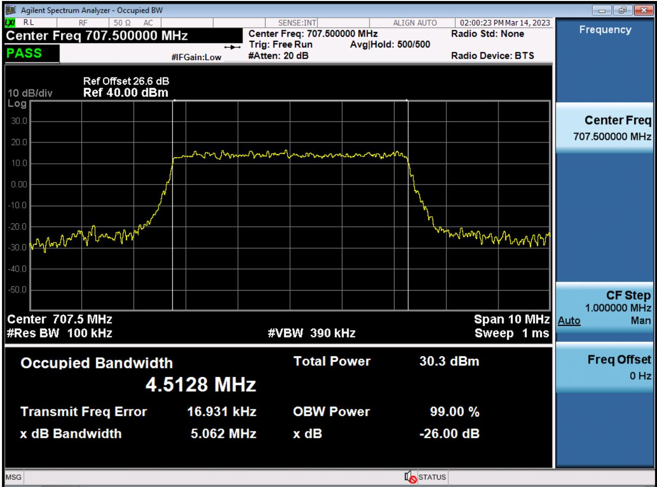
BAND 12. Occupied Bandwidth Plot (5 M BW Ch.23095 256QAM\_RB25\_0)
