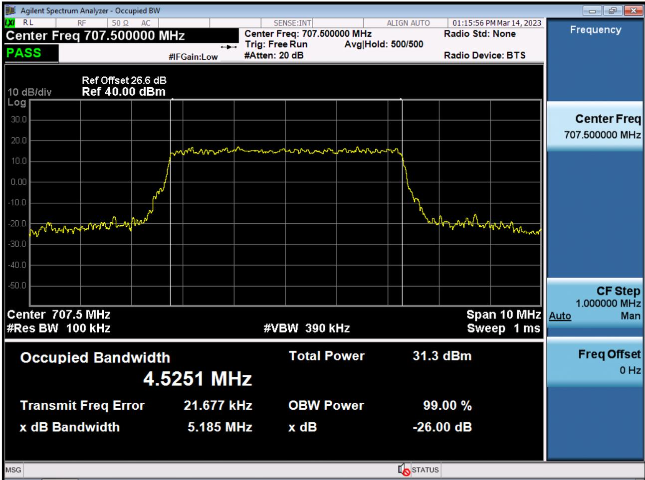
BAND 12. Occupied Bandwidth Plot (5 M BW Ch.23095 64QAM\_RB25\_0)
