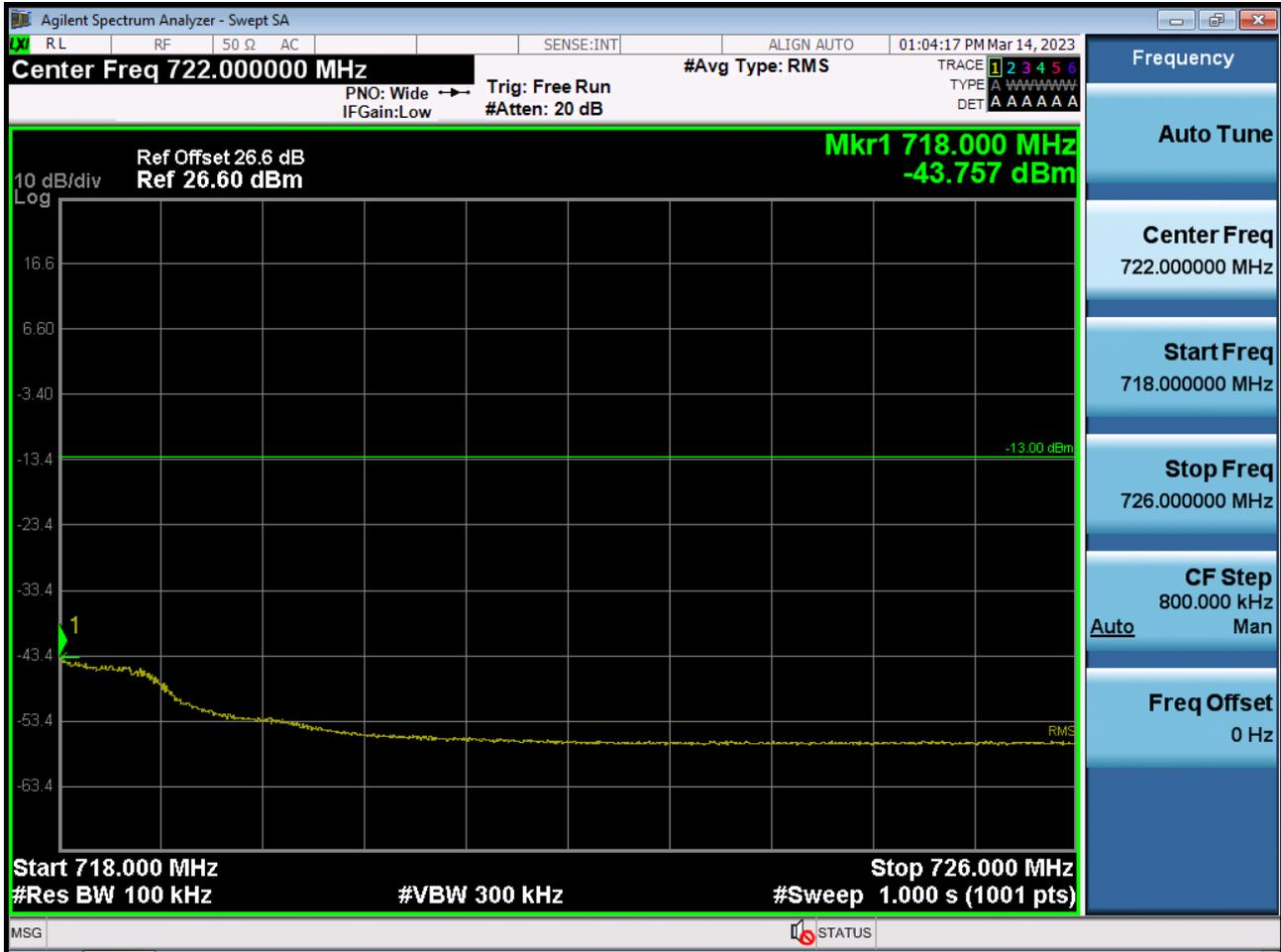
BAND 12. Upper Band Edge Plot (3 M BW Ch.23165 QPSK\_RB1\_Offset 14)-1
