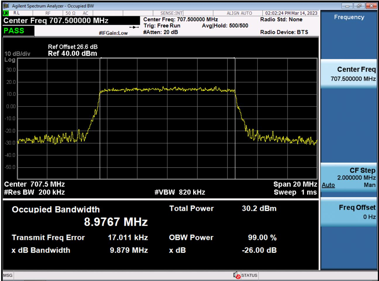
BAND 12. Occupied Bandwidth Plot (10 M BW Ch.23095 256QAM\_RB50\_0)
