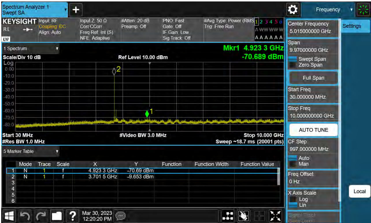
Sub6 n77. Conducted Spurious Plot_1 (649000ch_70 MHz_BPSK)
