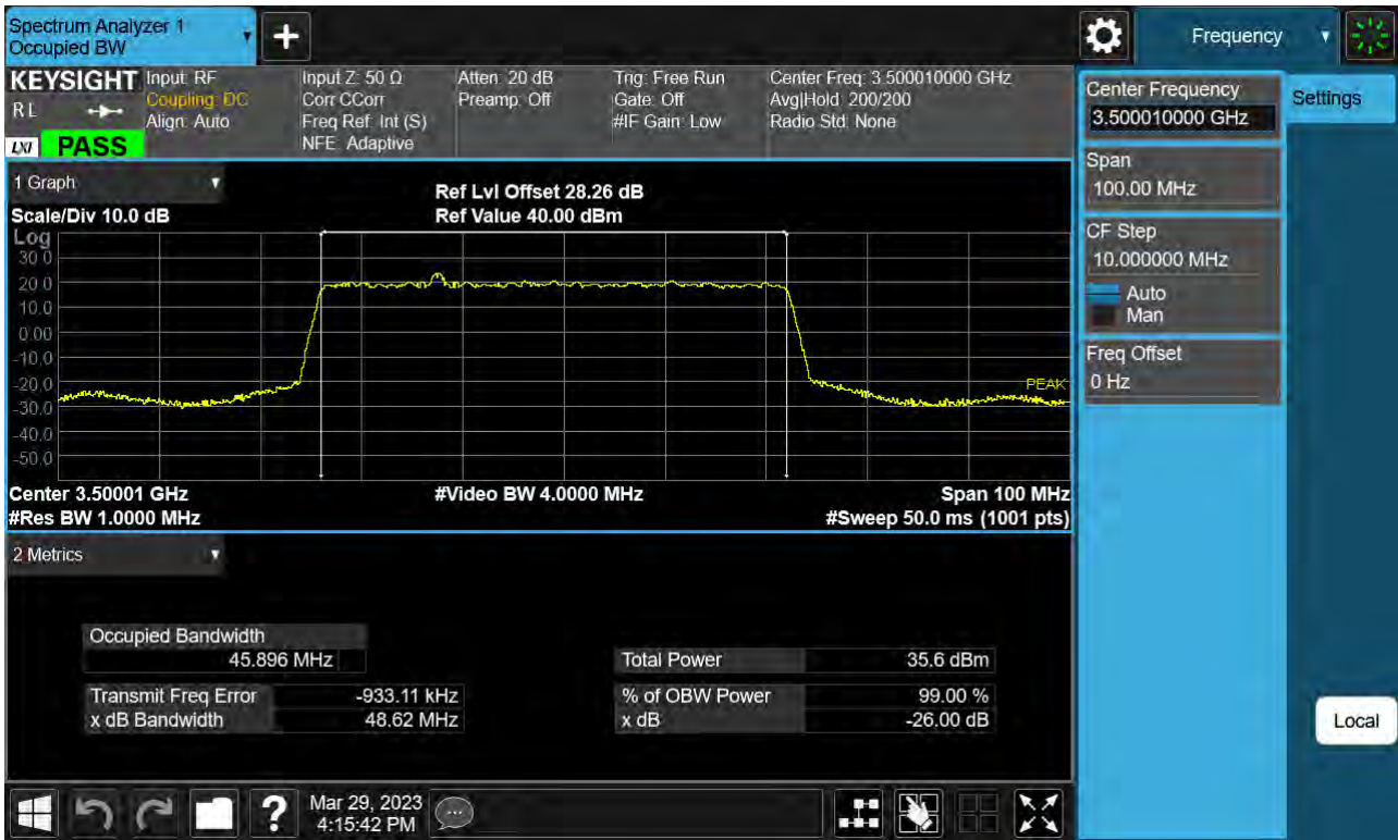
Sub6 n77. Occupied Bandwidth Plot (50 M BW Ch.633334 BPSK )
