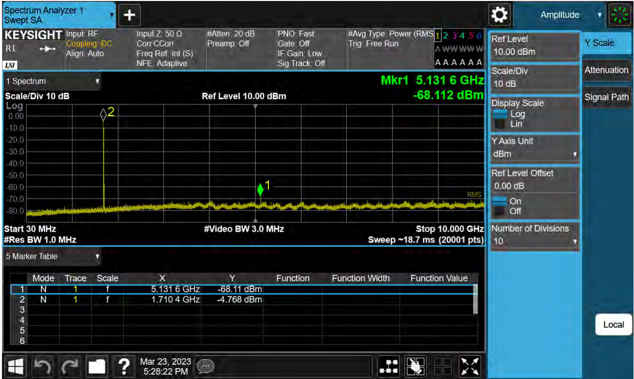
Sub6 n66. Conducted Spurious Plot_1 (343500ch_15 MHz_BPSK_RB 1_1)
