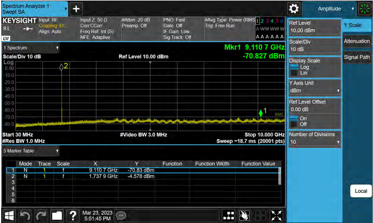
Sub6 n66. Conducted Spurious Plot_1 (349000ch_15 MHz_BPSK_RB 1_1)
