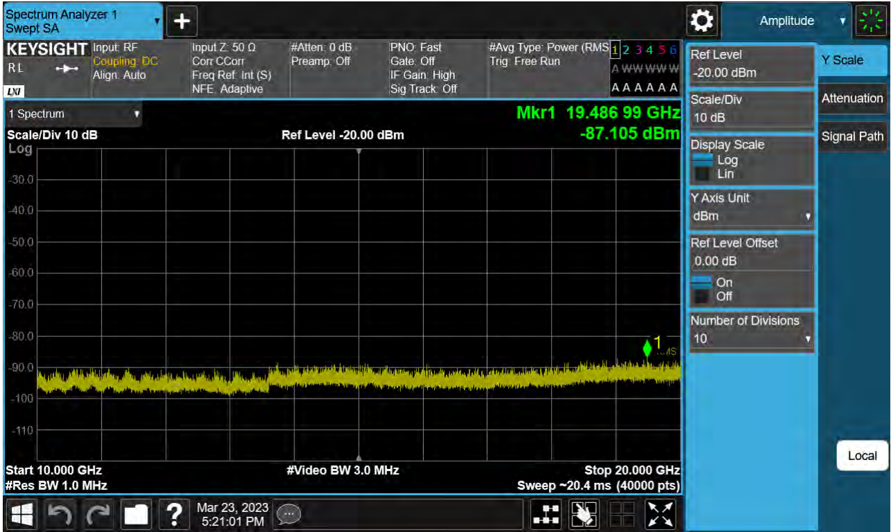
Sub6 n66. Conducted Spurious Plot_2 (343000ch_10 MHz_BPSK_RB 1_1)
