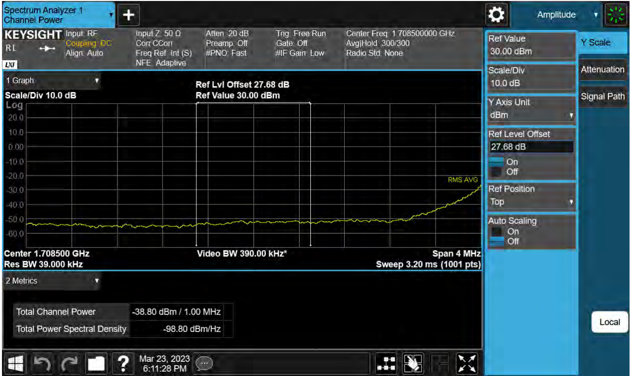
Sub6 n66. Lower Extended Band Edge Plot (40 M BW Ch.346000 BPSK_ Full RB) -3
