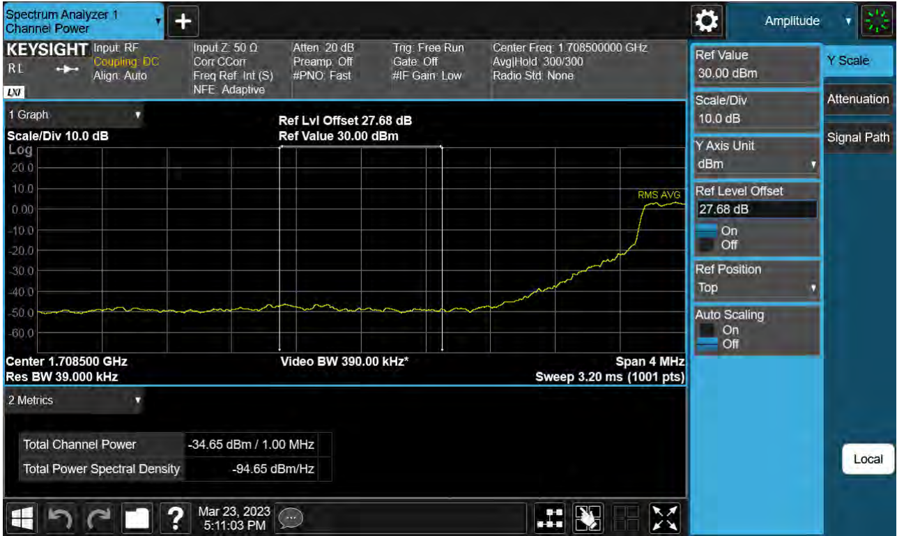
Sub6 n66. Lower Extended Band Edge Plot (5 M BW Ch.342500 BPSK_ Full RB) -3
