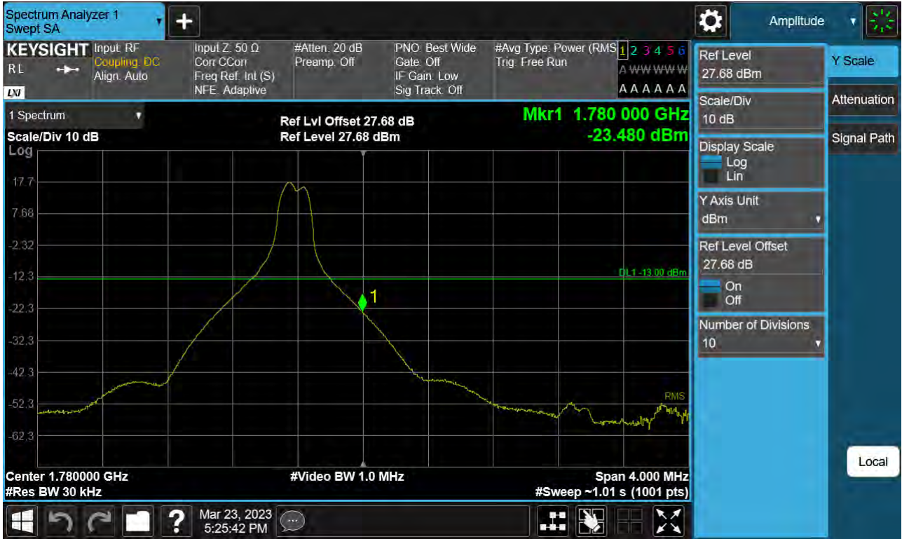
Sub6 n66. Upper Band Edge Plot (10 M BW Ch.355000 BPSK_RB1_Offset 51) -1
