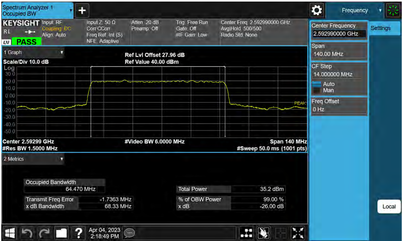
Sub6 n41. Occupied Bandwidth Plot (70 MHz Ch.518598 BPSK )
