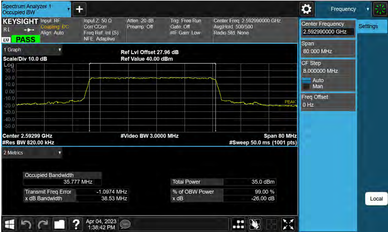
Sub6 n41. Occupied Bandwidth Plot (40 MHz Ch.518598 QPSK )
