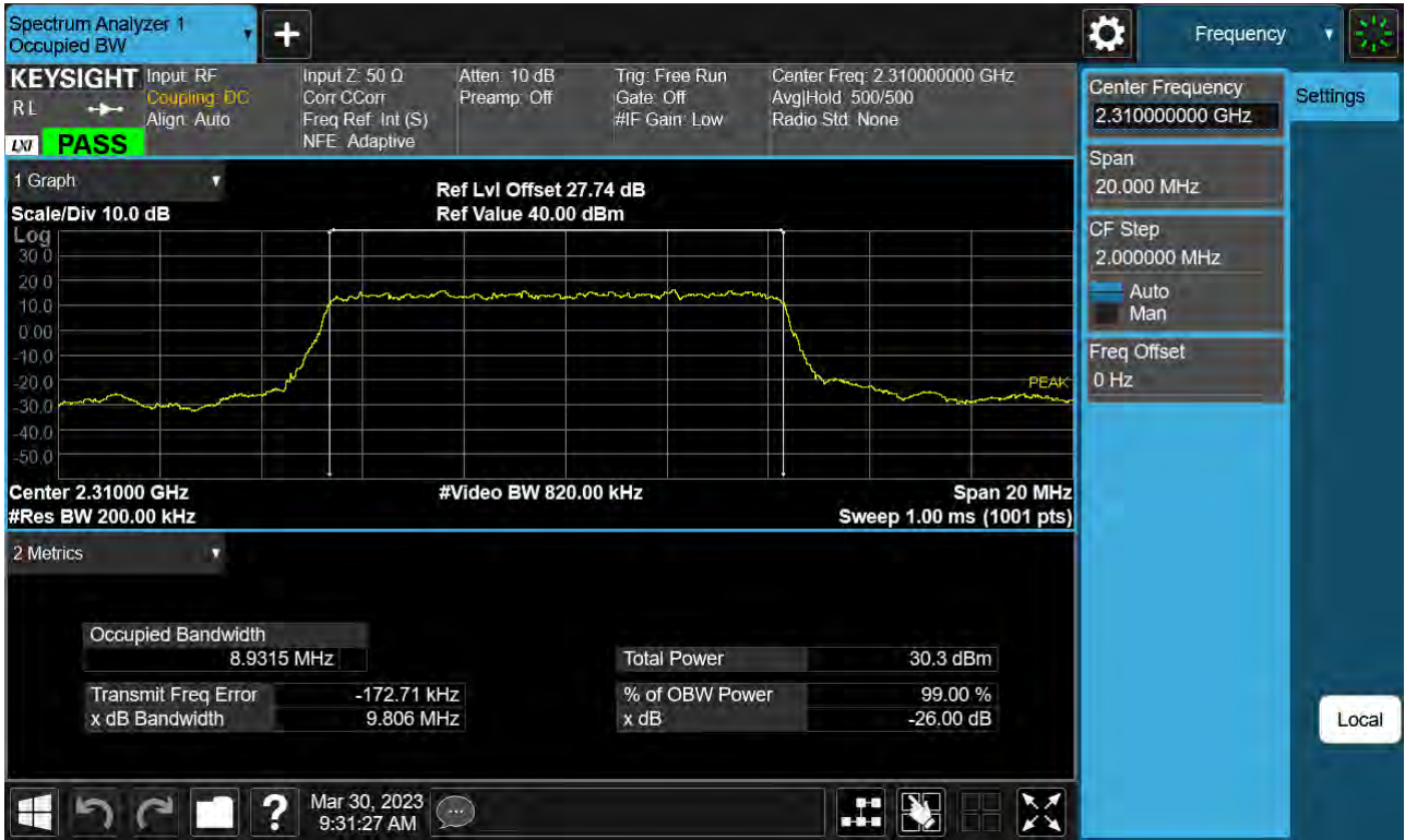
Sub6 n30. Occupied Bandwidth Plot (10 MHz Ch.462000 BPSK RB 50)
