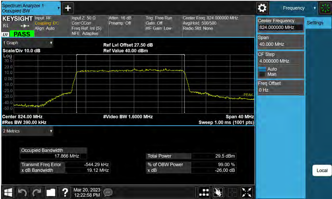
Sub6 n26. Occupied Bandwidth Plot (20 M BW Ch.164800 64QAM RB 100_0)
