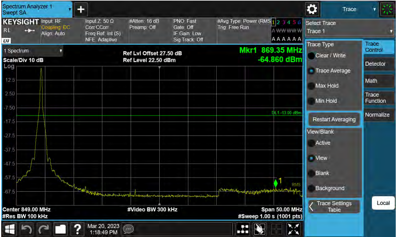
Sub6 n26. Lower Band Edge Plot (15 M BW Ch.164300 BPSK_RB1_Offset 0)
