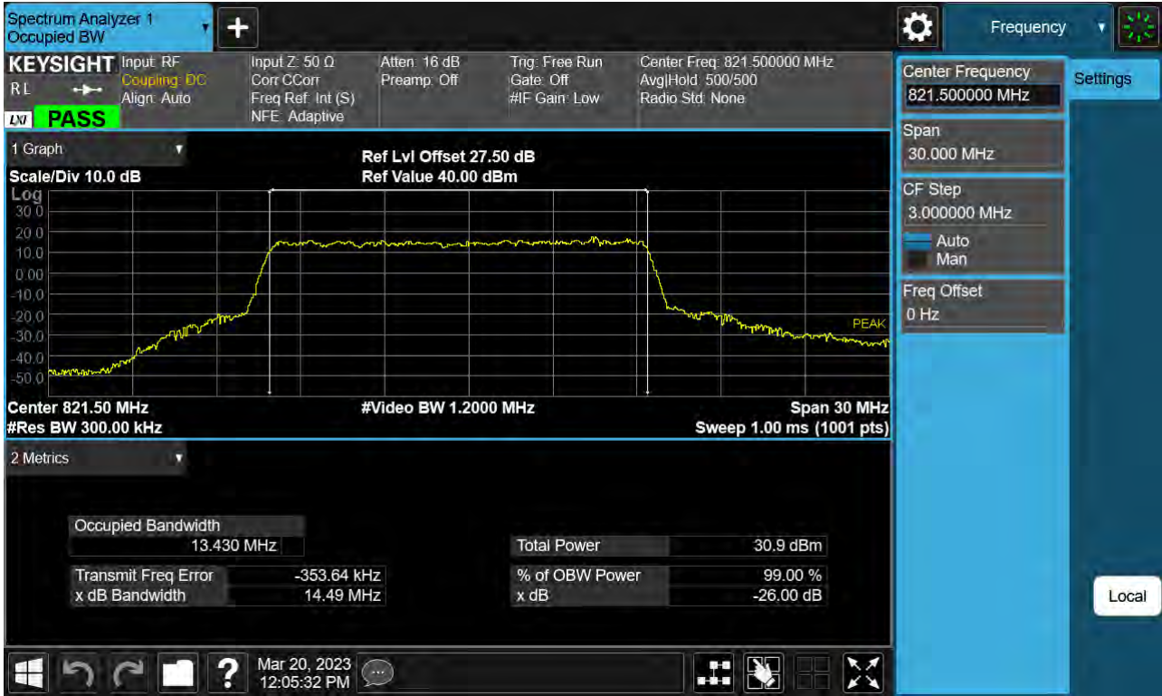
Sub6 n26. Occupied Bandwidth Plot (15 M BW Ch.164300 QPSK RB 75_0)
