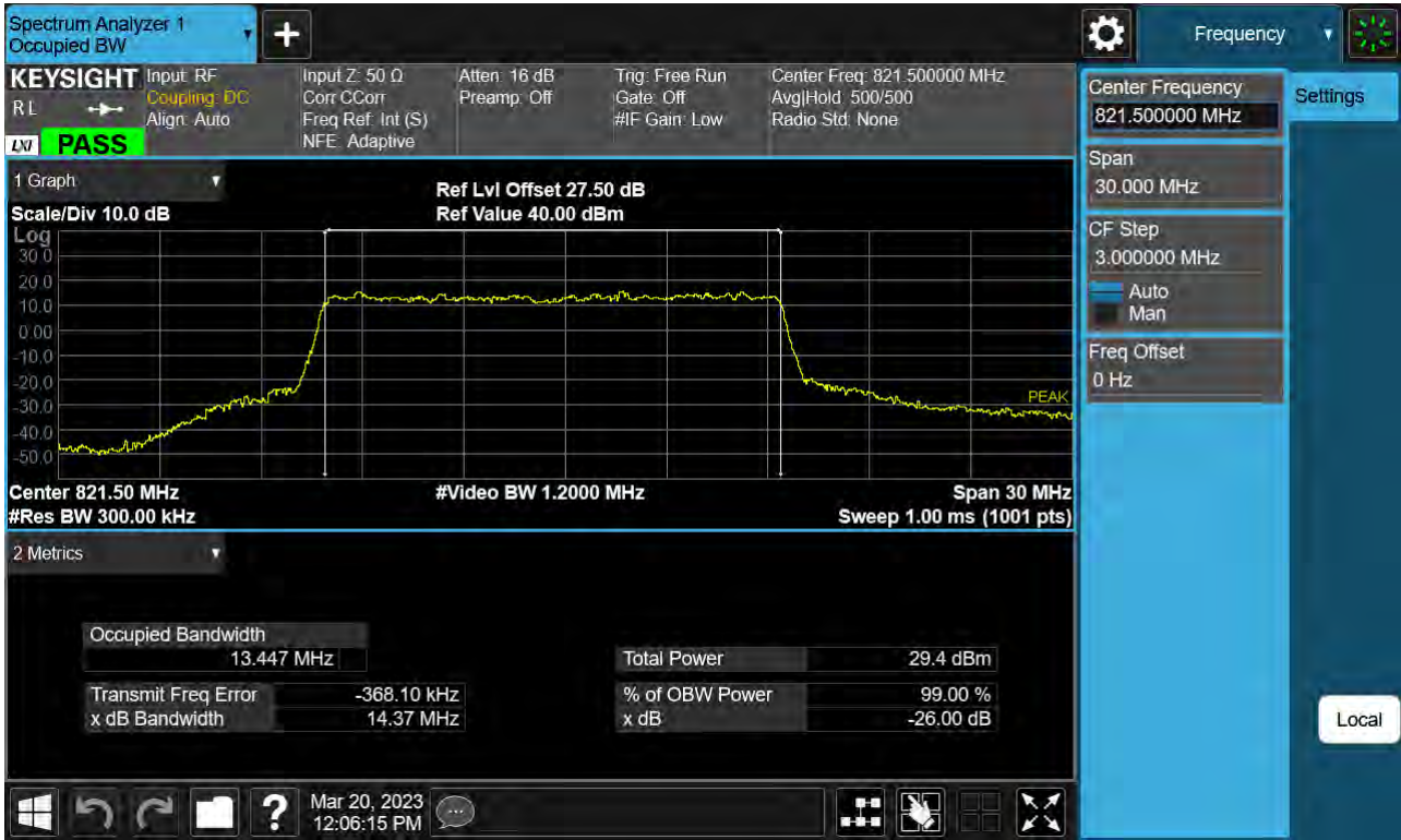
Sub6 n26. Occupied Bandwidth Plot (15 M BW Ch.164300 64QAM RB 75_0)
