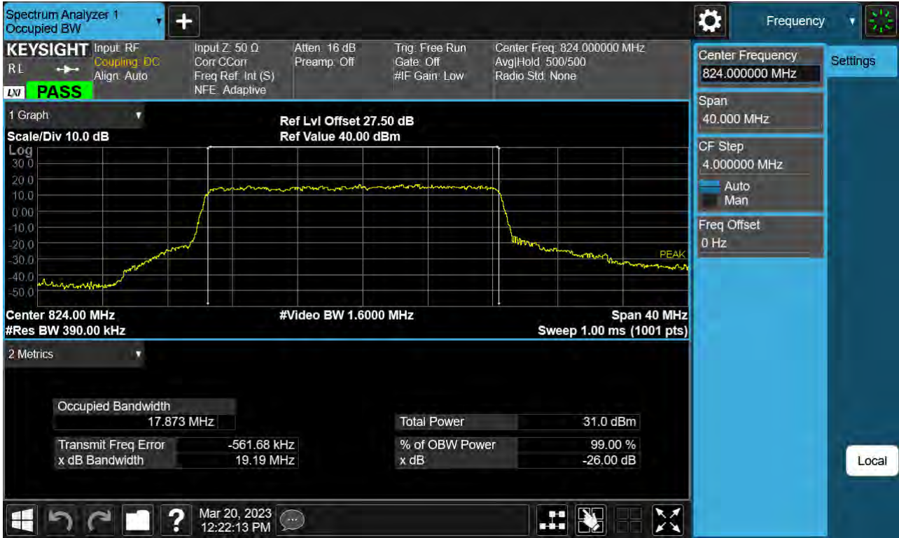
Sub6 n26. Occupied Bandwidth Plot (20 M BW Ch.164800 QPSK RB 100_0)
