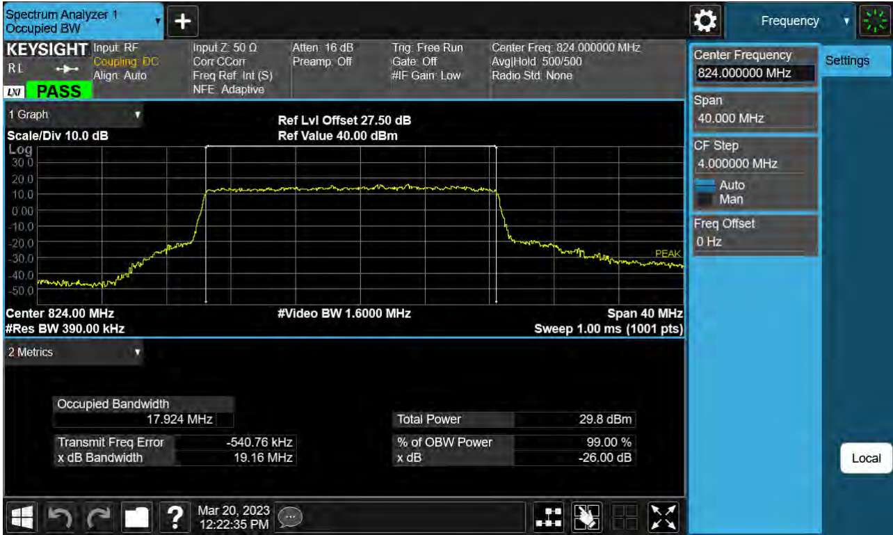
Sub6 n26. Occupied Bandwidth Plot (20 M BW Ch.164800 16QAM RB 100_0)
