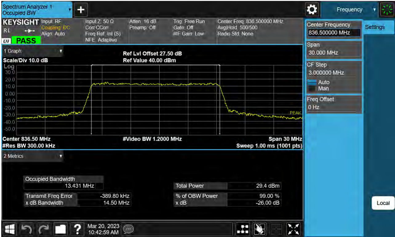
Sub6 n26. Occupied Bandwidth Plot (15 M BW Ch.167300 64QAM RB 75_0)
