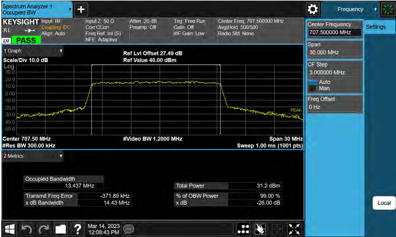
Sub6 n12. Occupied Bandwidth Plot (15M BW Ch.141500 16QAM_RB75_0)
