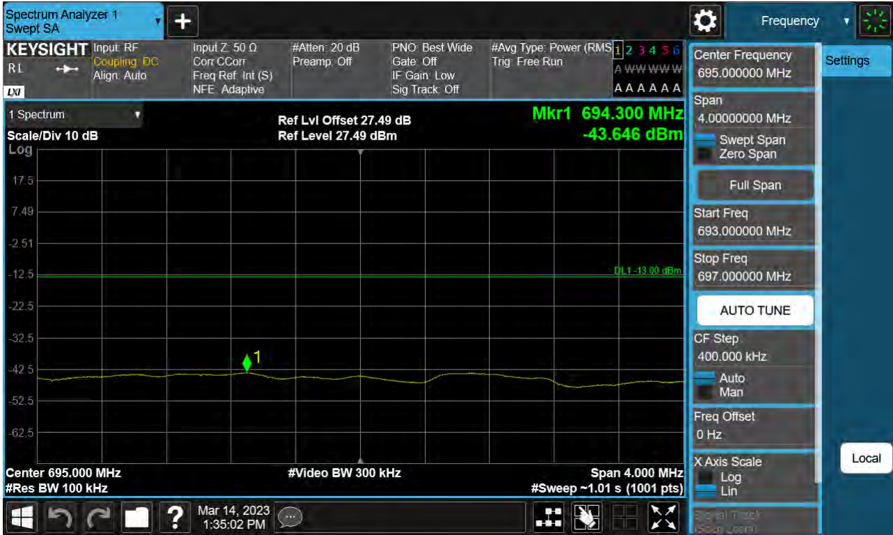
Sub6 n12. Lower Extended Band Edge Plot (15M BW Ch.141300 BPSK_RB75_0)
