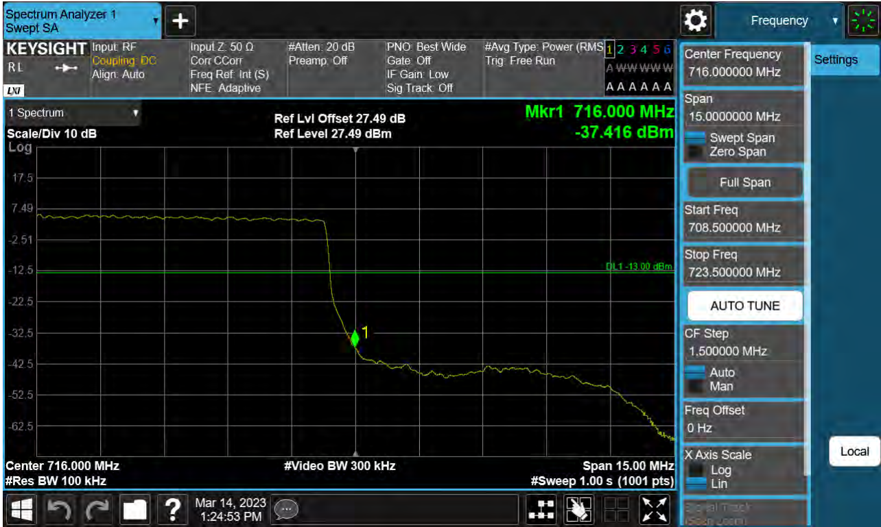
Sub6 n12. Upper Band Edge Plot (10M BW Ch.142200 BPSK_RB50_Offset 0)
