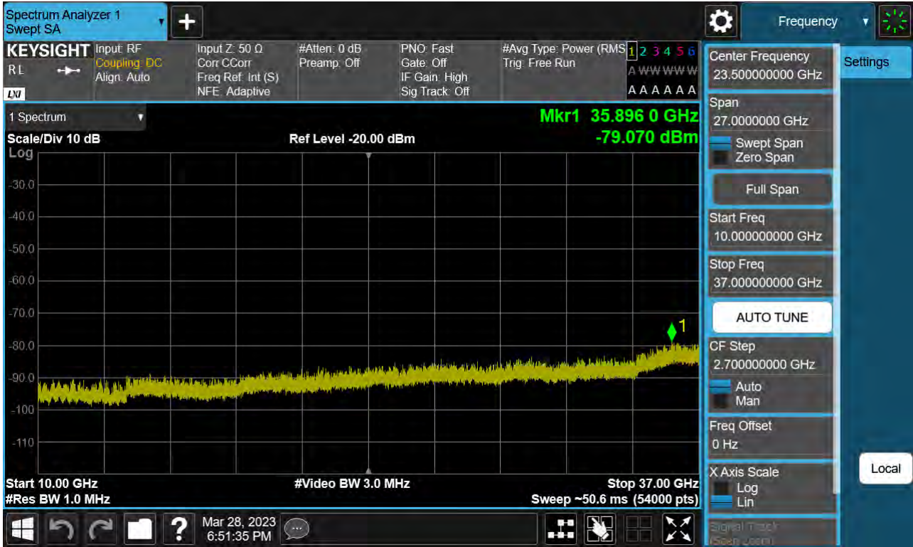
Sub6 n48. Conducted Spurious Plot 2 (15 MHz Ch. 646166 BPSK RB 1, Offset 1)
