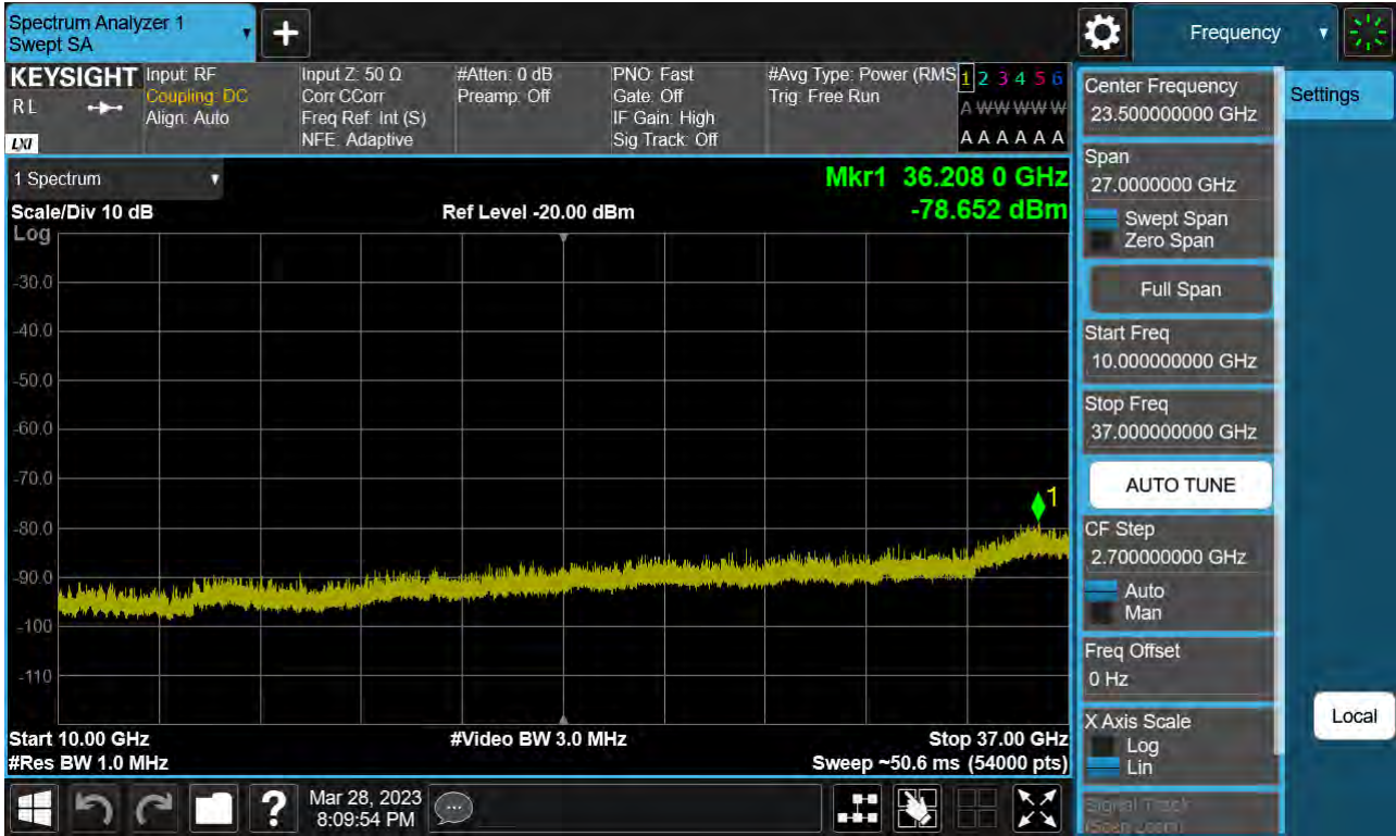
Sub6 n48. Conducted Spurious Plot 2 (30 MHz Ch. 641666 BPSK RB 1, Offset 1)
