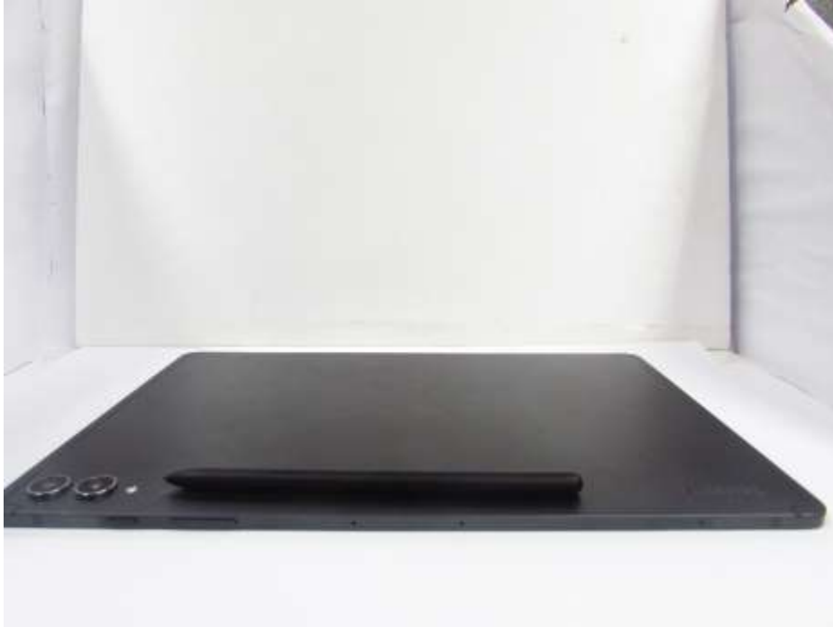
Positions of SPEN and DUT during charging.
