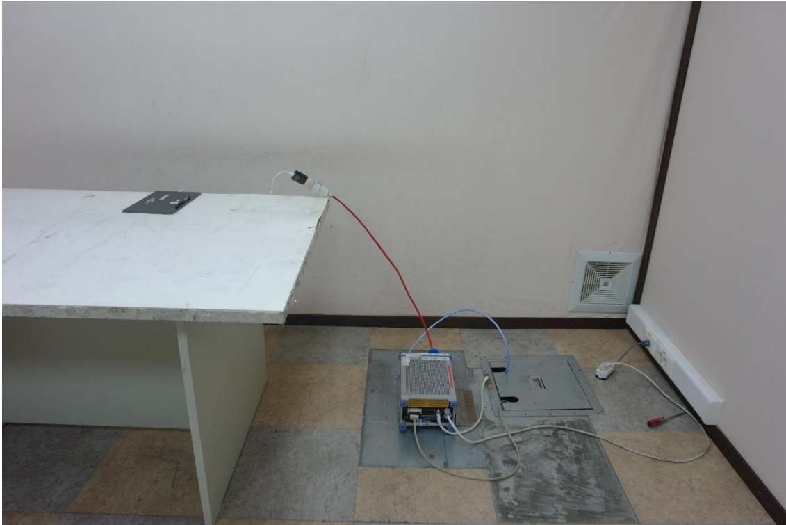
AC PowerLine Conducted Test WPS(S-pen) Setup Photo
