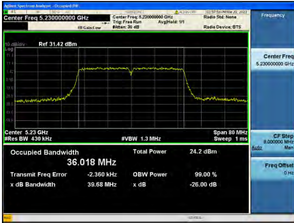
802.11ac_VHT40 UNII 2C BAND 26 dB Bandwidth(CH 142)
