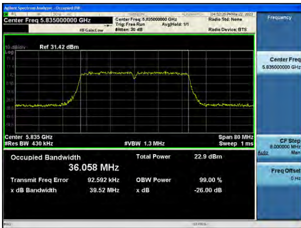
802.11n_HT40 UNII 4 BAND 26 dB Bandwidth (CH 167)
