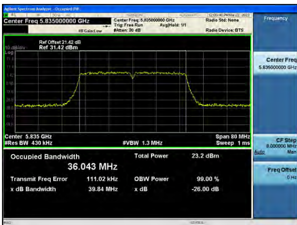
802.11ac_VHT40 UNII 4 BAND 26 dB Bandwidth (CH 167)
