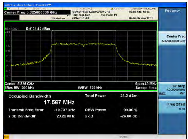
802.11n_HT20 UNII 3 BAND 26 dB Bandwidth(CH 165)
