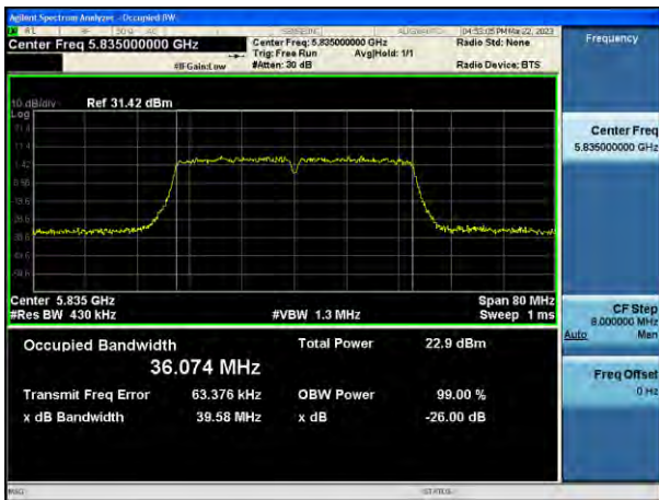
802.11ac_VHT40 UNII 4 BAND 26 dB Bandwidth (CH 167)
