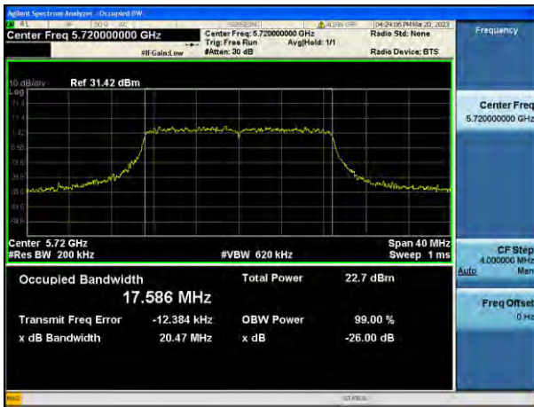
802.11ac_VHT20 UNII 4 BAND 26 dB Bandwidth(CH 169)
