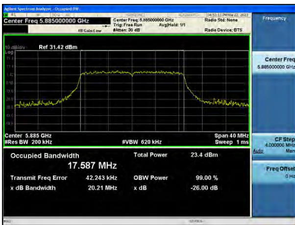
802.11n_HT20 UNII 4 BAND 26 dB Bandwidth(CH 177)
