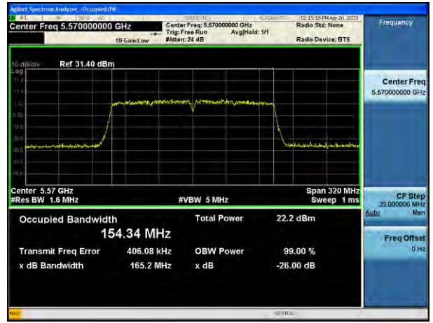
802.11ac_VHT160 UNII 2A BAND 26 dB Bandwidth (CH 114)
