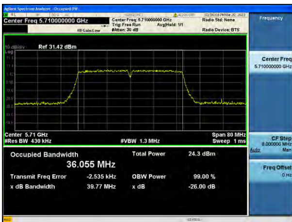
802.11n_HT40 UNII 4 BAND 26 dB Bandwidth (CH 175)
