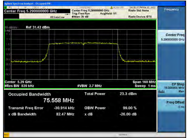
802.11ac_VHT80 UNII 3 BAND 26 dB Bandwidth (CH 155)
