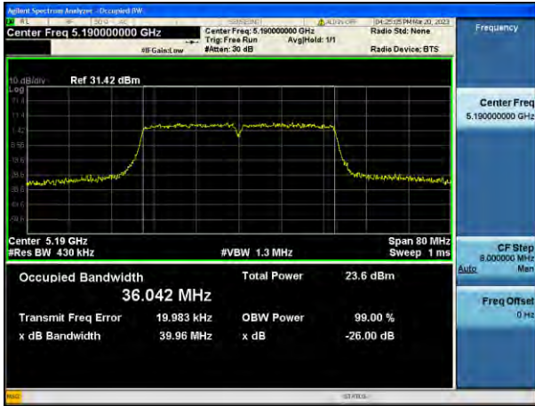
802.11n_HT40 UNII 2C BAND 26 dB Bandwidth(CH 142)
