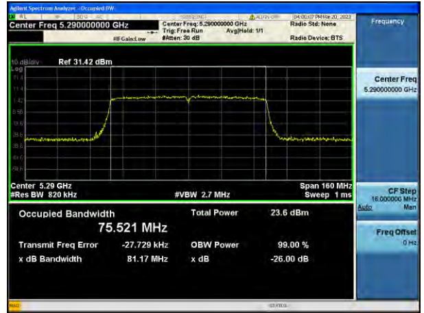
802.11ac_VHT80 UNII 3 BAND 26 dB Bandwidth (CH 155)
