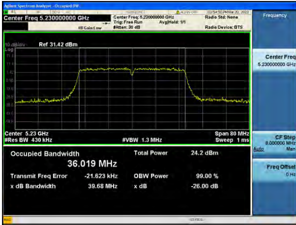
802.11n_HT40 UNII 2C BAND 26 dB Bandwidth(CH 142)
