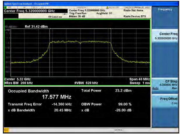
802.11ac_VHT20 UNII 3 BAND 26 dB Bandwidth(CH 165)
