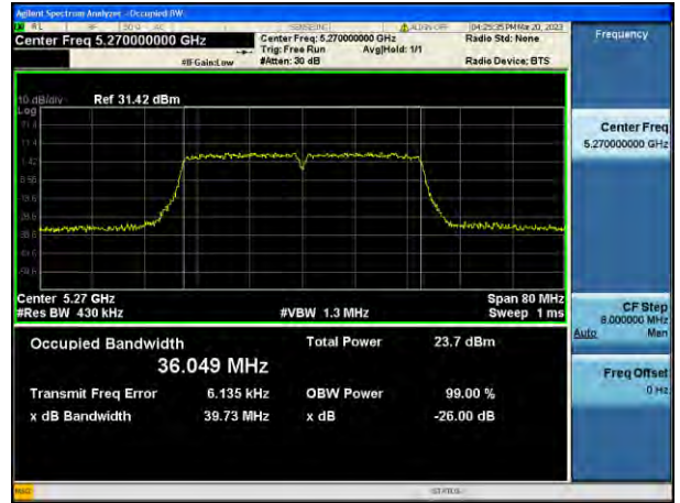
802.11n_HT40 UNII 3 BAND 26 dB Bandwidth (CH 159)
