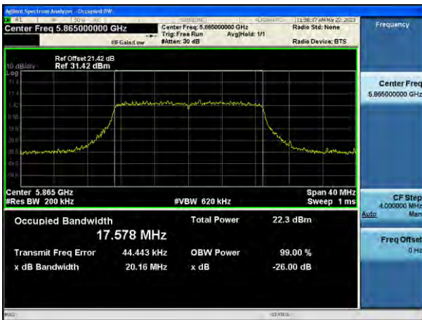
802.11n_HT20 UNII 4 BAND 26 dB Bandwidth(CH 173)
