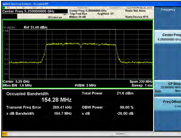
802.11ac_VHT160 UNII 4 BAND 26 dB Bandwidth(CH 163)
