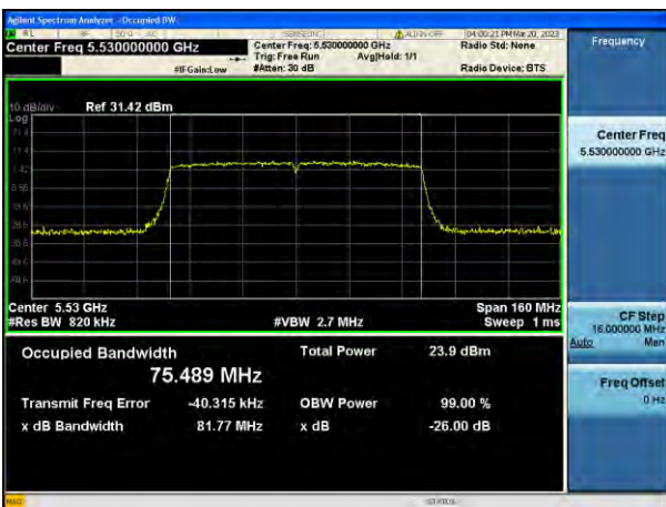
802.11ac_VHT80 UNII 4 BAND 26 dB Bandwidth (CH 171)
