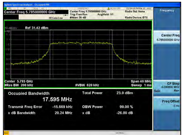
802.11ac_VHT20 UNII 3 BAND 26 dB Bandwidth(CH 157)
