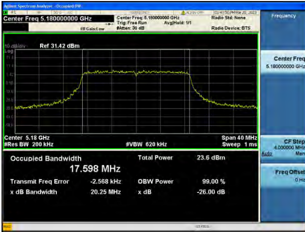
802.11n_HT20 UNII 2C BAND 26 dB Bandwidth(CH 144)
