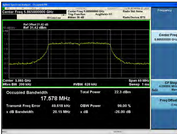
802.11ac_VHT20 UNII 4 BAND 26 dB Bandwidth(CH 173)
