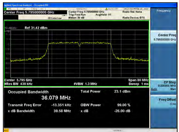
802.11n_HT40 UNII 3 BAND 26 dB Bandwidth (CH 159)
