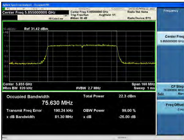
802.11ac_VHT80 UNII 4 BAND 26 dB Bandwidth (CH 171)
