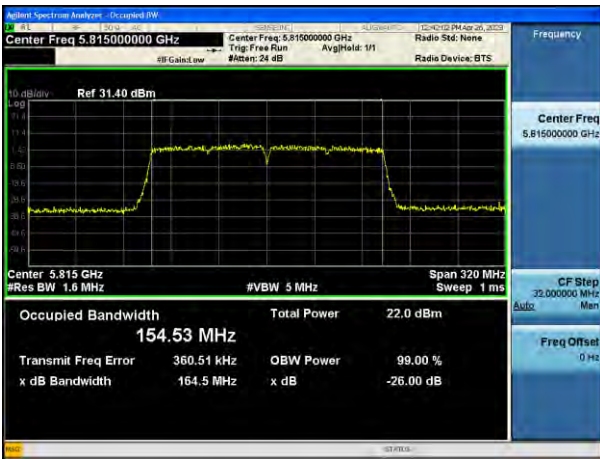
802.11ac_VHT160 UNII 4 BAND 26 dB Bandwidth(CH 163)
