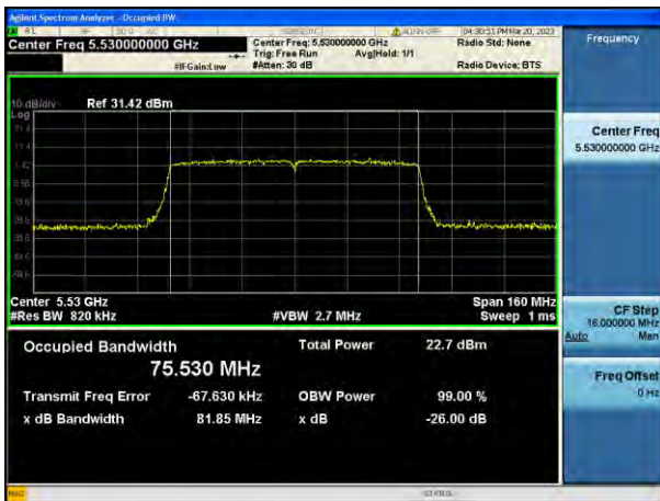
802.11ac_VHT80 UNII 4 BAND 26 dB Bandwidth (CH 171)
