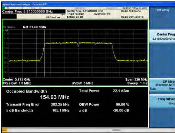
802.11ac_VHT160 UNII 4 BAND 26 dB Bandwidth(CH 163)
