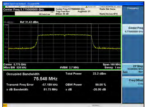
802.11ac_VHT80 UNII 3 BAND 26 dB Bandwidth (CH 155)
