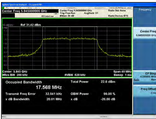
802.11ac_VHT20 UNII 4 BAND 26 dB Bandwidth(CH 169)
