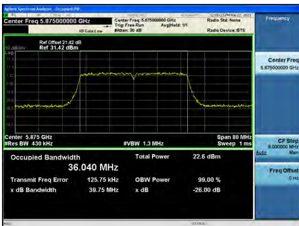
802.11n_HT40 UNII 4 BAND 26 dB Bandwidth (CH 175)
