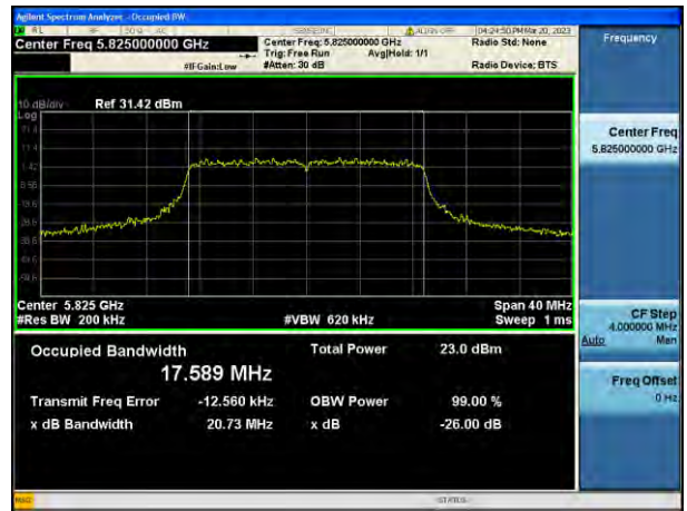
802.11ac_VHT20 UNII 3 BAND 26 dB Bandwidth(CH 165)
