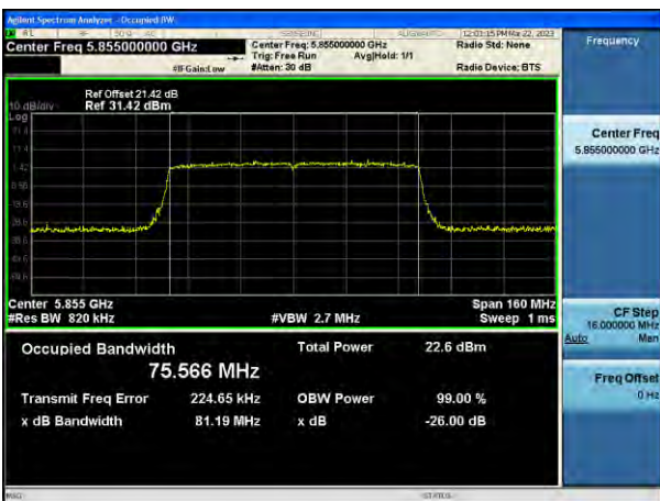
802.11ac_VHT80 UNII 4 BAND 26 dB Bandwidth (CH 171)
