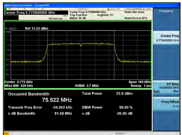
802.11ac_VHT80 UNII 3 BAND 26 dB Bandwidth (CH 155)
