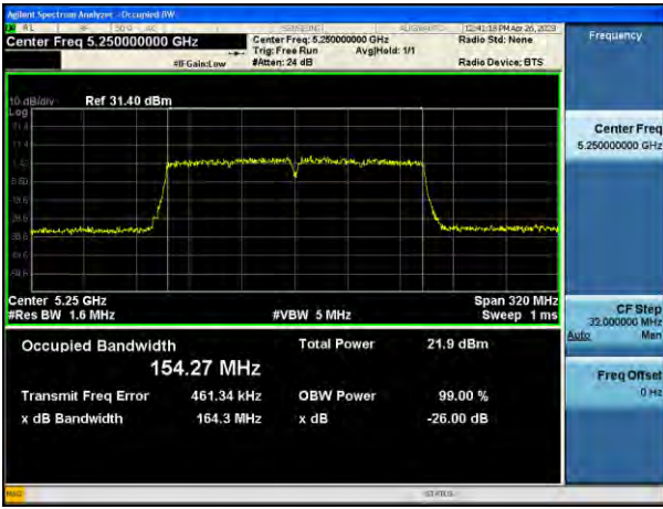
802.11ac_VHT160 UNII 4 BAND 26 dB Bandwidth(CH 163)
