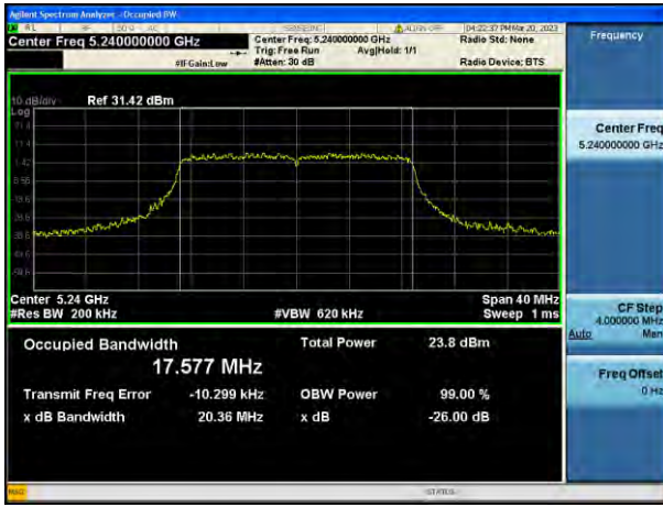
802.11ac_VHT20 UNII 2C BAND 26 dB Bandwidth(CH 144)
