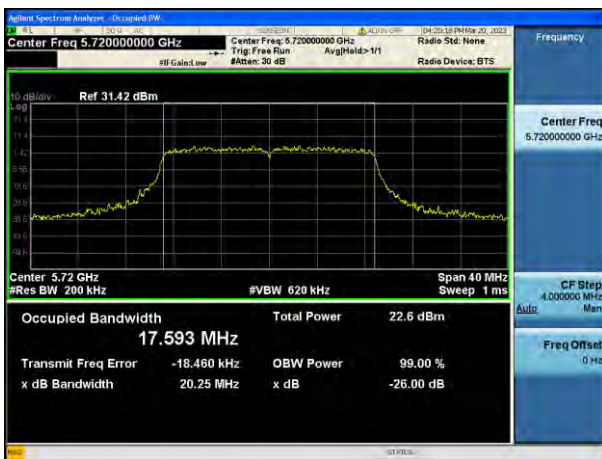
802.11n_HT20 UNII 4 BAND 26 dB Bandwidth(CH 177)
