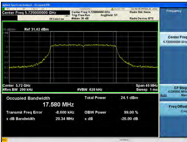
802.11n_HT20 UNII 4 BAND 26 dB Bandwidth(CH 173)
