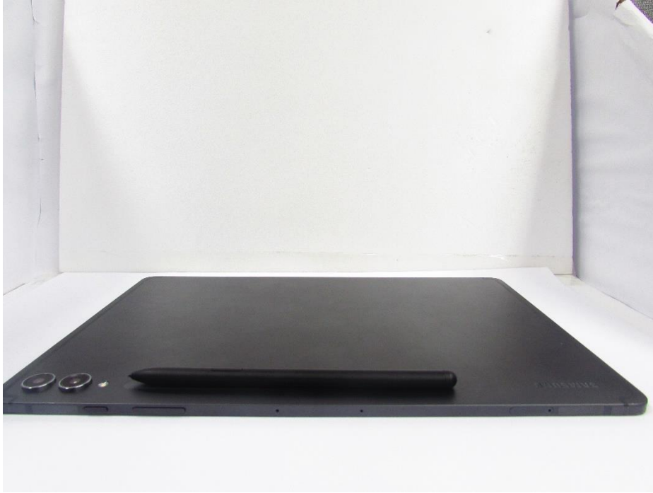
Positions of SPEN and DUT during charging.
