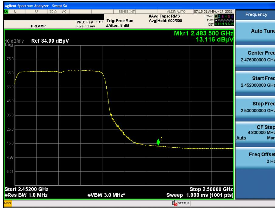
Radiated Restricted Band Edges plot – Peak result (802.11ax(HE20) Ch.11)
