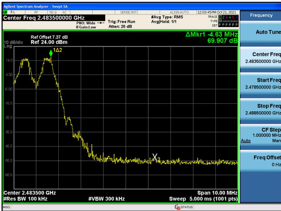
Test Plots with hopping (8DPSK)
