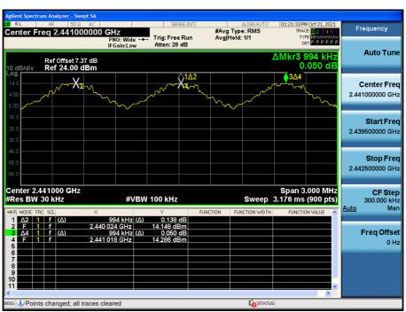
Test Plots (8DPSK) Channel Separation
