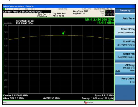
Test Plots (8DPSK) Peak Power (CH.0)
