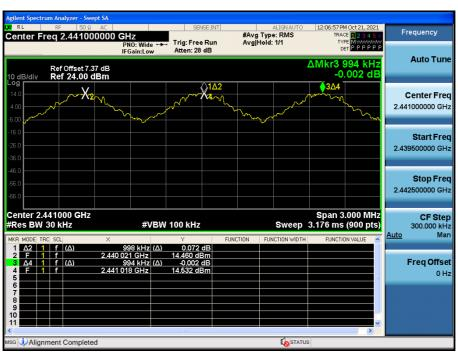
Test Plots (8DPSK) Channel Separation
