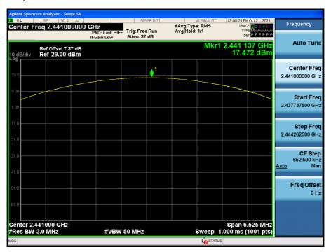
Test Plots (8DPSK) Peak Power (CH.78)
