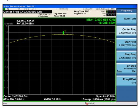
Test Plots (π/4DQPSK) Peak Power (CH.39)
