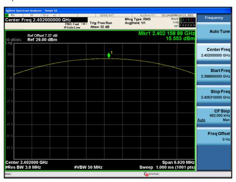
Test Plots (π/4DQPSK) Peak Power (CH.39)
