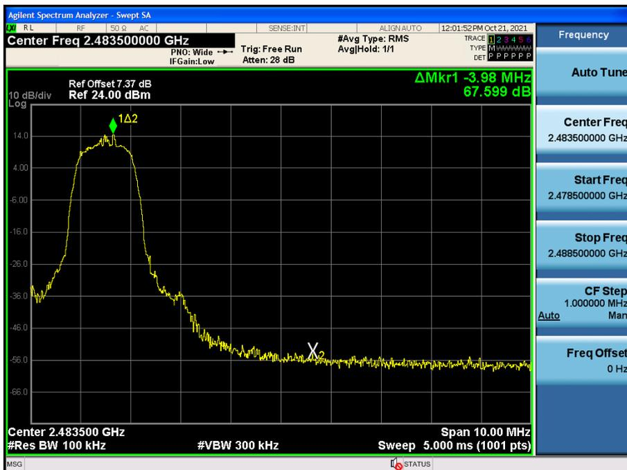
Test Plots with hopping (GFSK)
