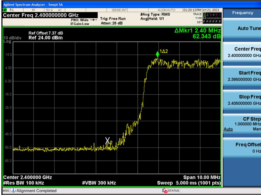
Test Plots with hopping (8DPSK)
