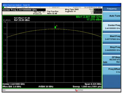
Test Plots (8DPSK) Peak Power (CH.78)
