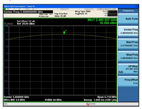
Test Plots (8DPSK) Peak Power (CH.0)
