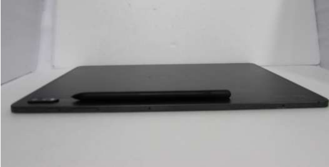
Positions of SPEN and DUT during charging.
