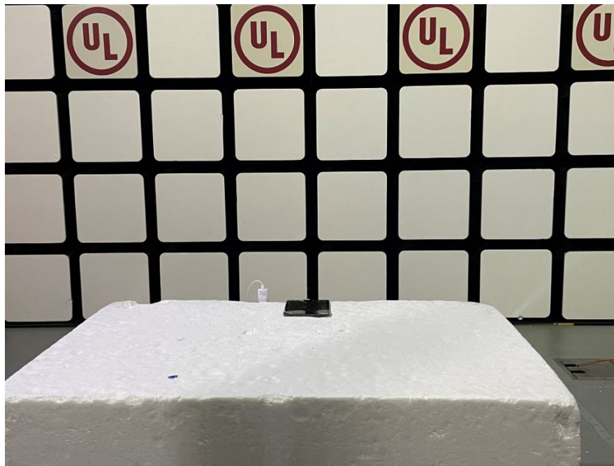
Photo of test setup for Radiated Emissions: >1GHz
