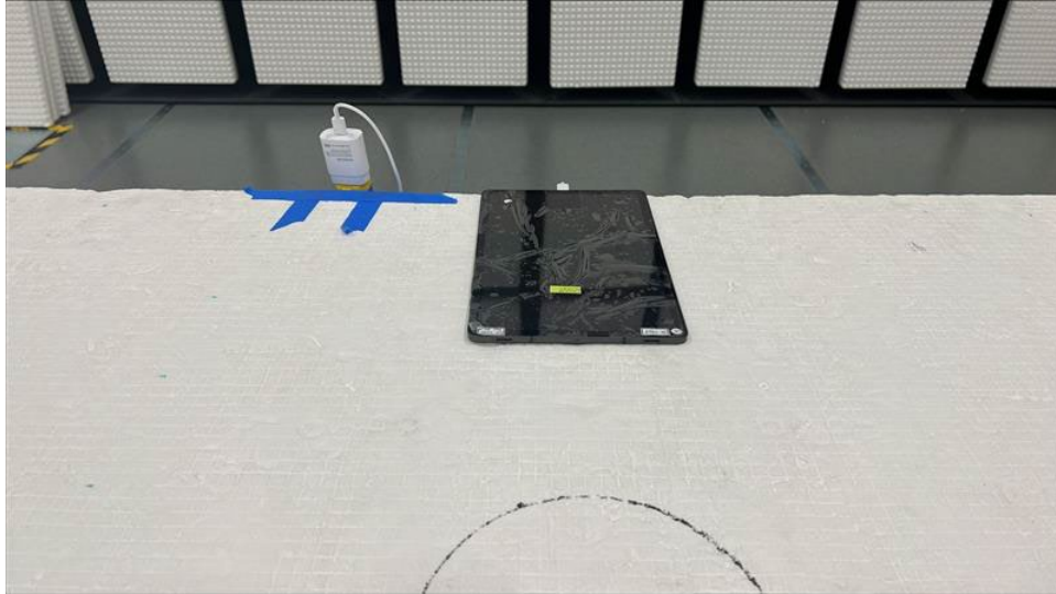
Photo of test setup for Radiated Emissions: 30-1000 MHz
