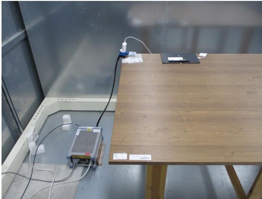
AC LINE CONDUCTED FRONT TEST PHOTO Test Case 2_Charging from EUT(Charging from TA) to S-Pen Position
