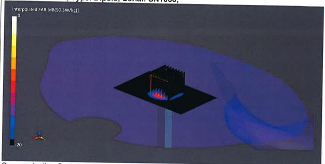
Communication System: CW UID: 0; Frequency: 6500.0 MHz; Duty Cycle: 1; Medium: HSL; Site63\_01Dec2022\_103835\_Head - 2600 5% 1950 10%; Medium parameters used: f = 6500.0 MHz;  $\sigma$  = 6.37 S/m;  $\epsilon_r$  = 33.3;  $\rho$  = 1000 kg/m3;  $\Delta\epsilon_r$  = -3.47 %;  $\Delta\sigma$  = 4.96 %; No correction
