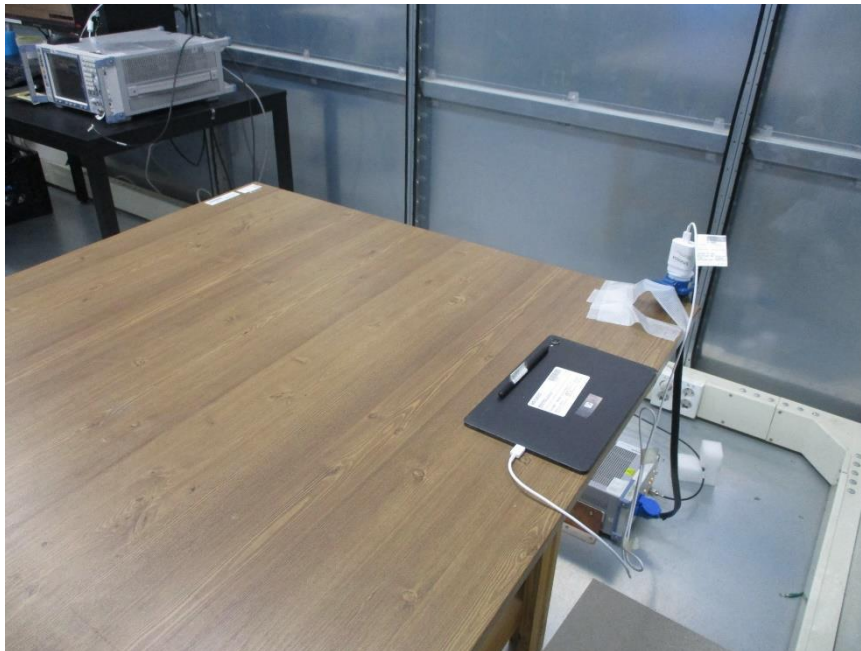
AC LINE CONDUCTED REAR TEST PHOTO Test Case 2_ Charging from EUT(Charging from TA) to S-Pen Position
