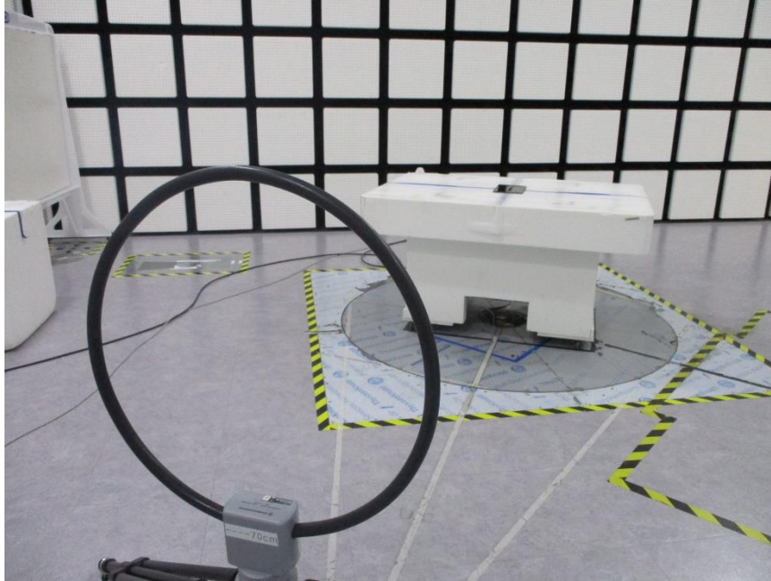
FACE ON FRONT TEST PHOTO Test Case 5_ Charging from EUT to S-Pen through Display Scan
