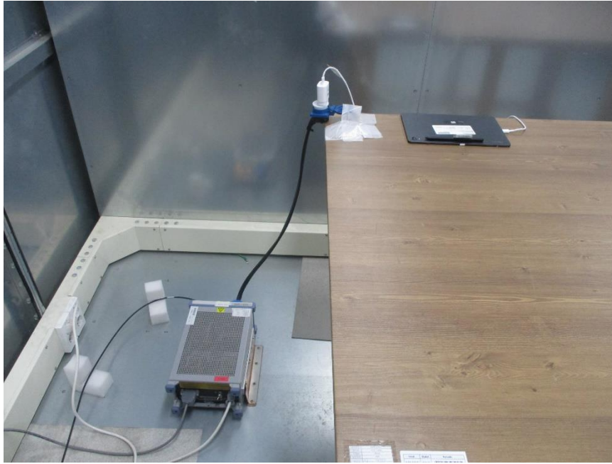
AC LINE CONDUCTED FRONT TEST PHOTO Test Case 2_ Charging from EUT(Charging from TA) to S-Pen Position
