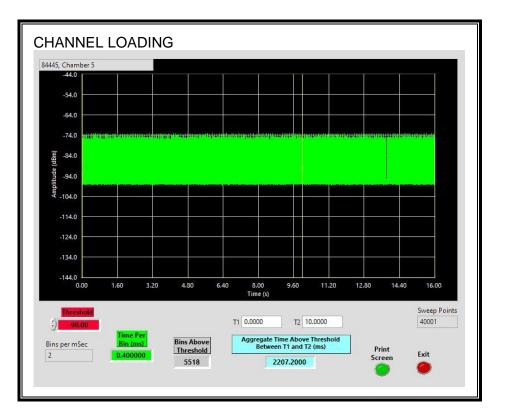
The level of traffic loading on the channel by the EUT is 22.072%
