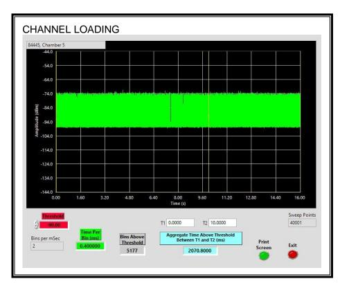
The level of traffic loading on the channel by the EUT is 20.708%
