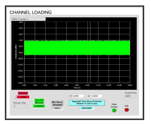
The level of traffic loading on the channel by the EUT is 22.044%
