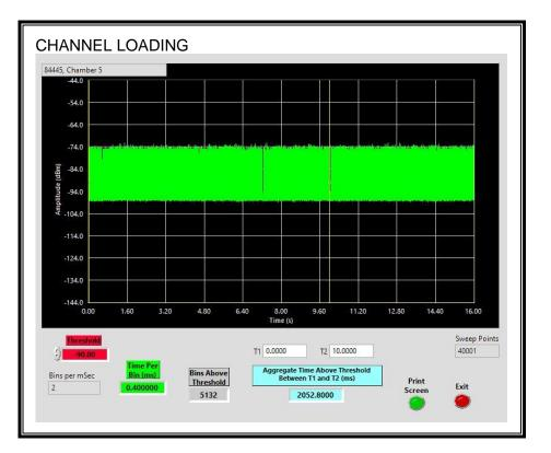
The level of traffic loading on the channel by the EUT is 20.528%
