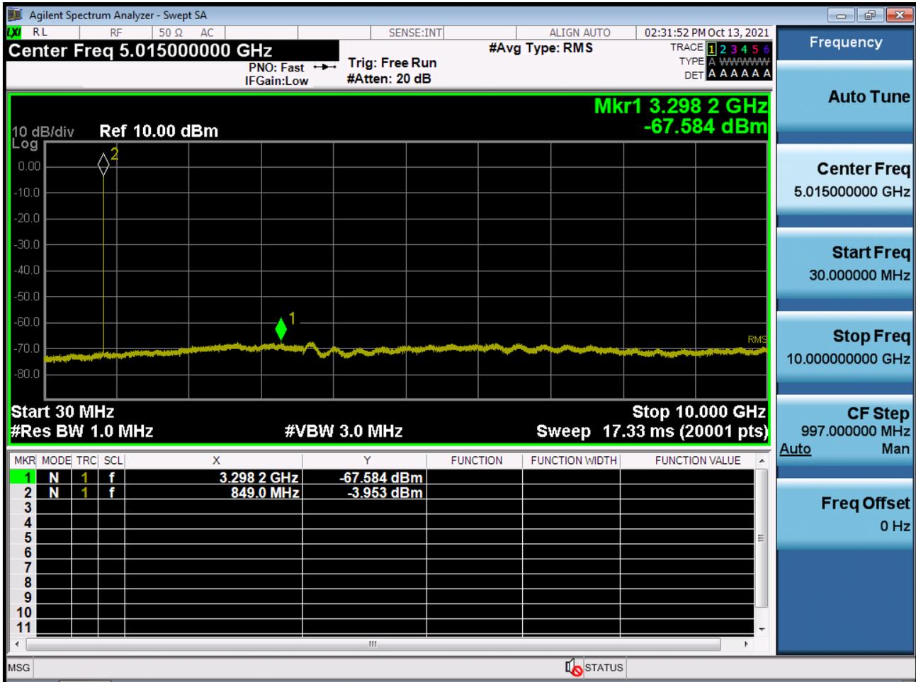
BAND 26. Conducted Spurious (26865ch\_15 MHz\_QPSK\_RB 1\_0)
