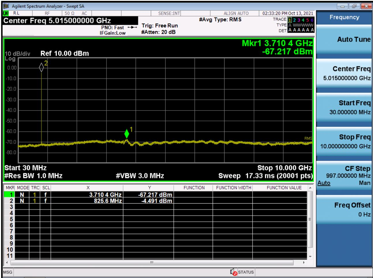
BAND 26. Conducted Spurious (26915ch\_15 MHz\_QPSK\_RB 1\_0)
