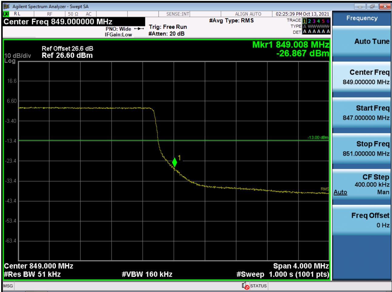
BAND26. Upper Band Edge Plot (10 M BW Ch.26990 QPSK\_RB50\_Offset 0)
