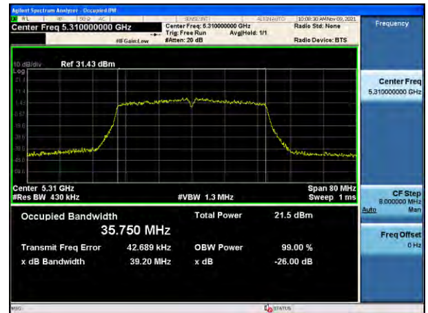
802.11ac_VHT40 UNII 3 BAND 26 dB Bandwidth (CH 151)
