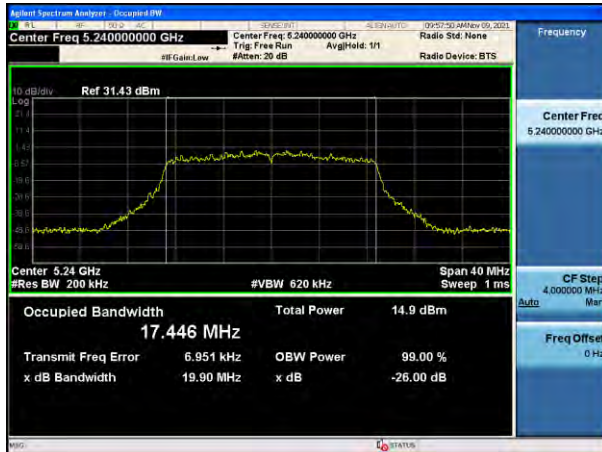
802.11n_HT20 UNII 2C BAND 26 dB Bandwidth(CH 116)
