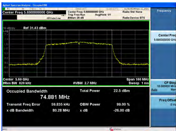
802.11ac_VHT80 UNII 4 BAND 26 dB Bandwidth (CH 171)
