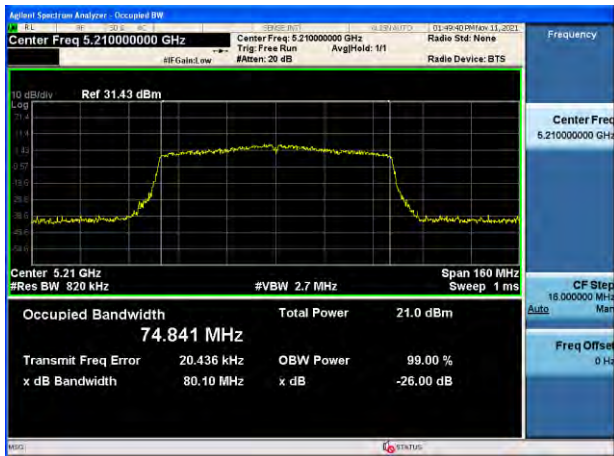
802.11ac_VHT80 UNII 2C BAND 26 dB Bandwidth(CH 138)
