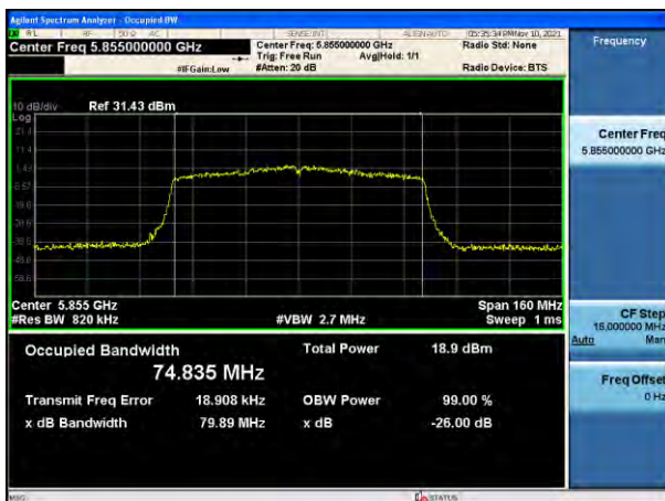
802.11ac_VHT80 UNII 4 BAND 26 dB Bandwidth (CH 171)
