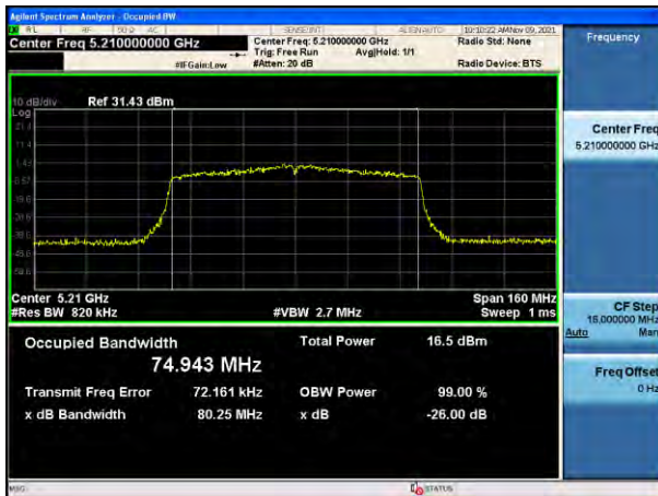
802.11ac_VHT80 UNII 2C BAND 26 dB Bandwidth(CH 106)
