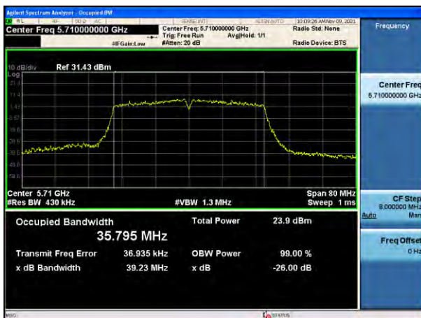
802.11ac_VHT40 UNII 4 BAND 26 dB Bandwidth (CH 167)
