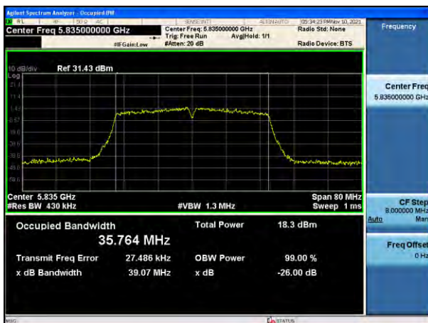
802.11n_HT40 UNII 4 BAND 26 dB Bandwidth (CH 167)
