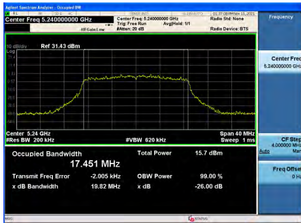
802.11n_HT20 UNII 2C BAND 26 dB Bandwidth(CH 116)
