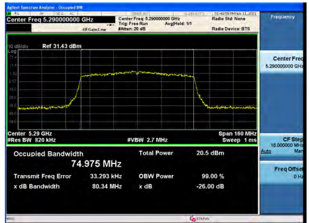
802.11ac_VHT80 UNII 3 BAND 26 dB Bandwidth (CH 155)
