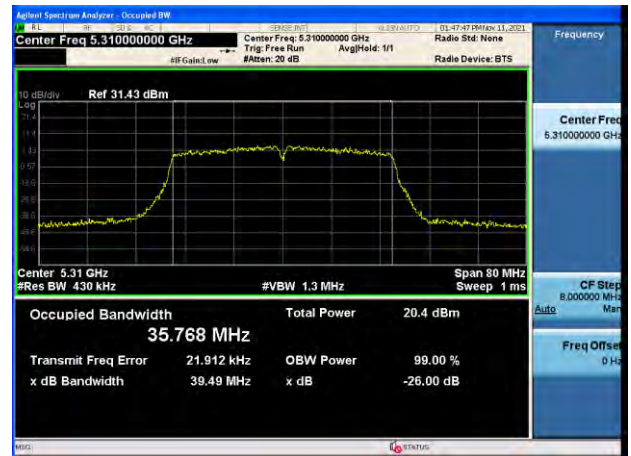
802.11ac_VHT40 UNII 3 BAND 26 dB Bandwidth (CH 159)
