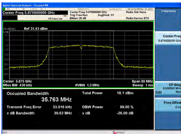
802.11ac_VHT40 UNII 4 BAND 26 dB Bandwidth (CH 175)
