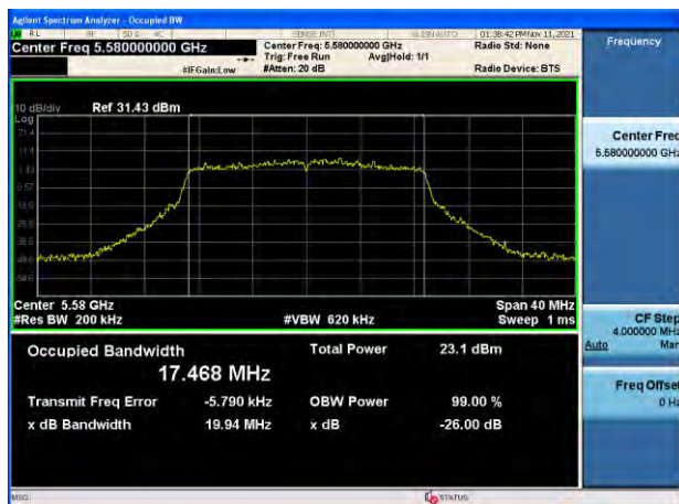
802.11n_HT20 UNII 4 BAND 26 dB Bandwidth(CH 173)
