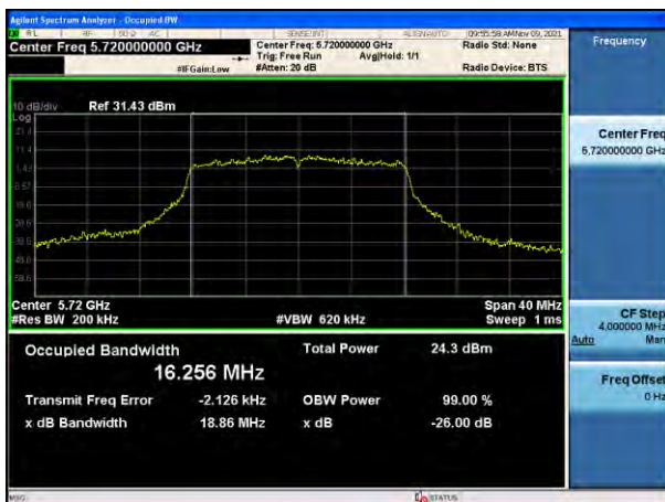
802.11a UNII 4 BAND 26 dB Bandwidth (CH 177)
