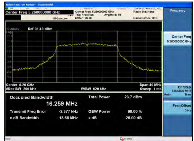
802.11a UNII 3 BAND 26 dB Bandwidth (CH 149)
