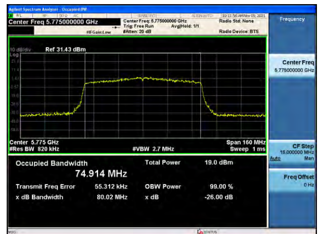
802.11ac_VHT80 UNII 3 BAND 26 dB Bandwidth (CH 155)
