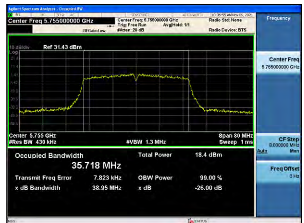
802.11n_HT40 UNII 3 BAND 26 dB Bandwidth (CH 151)
