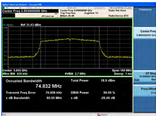
802.11ac_VHT80 UNII 4 BAND 26 dB Bandwidth (CH 171)
