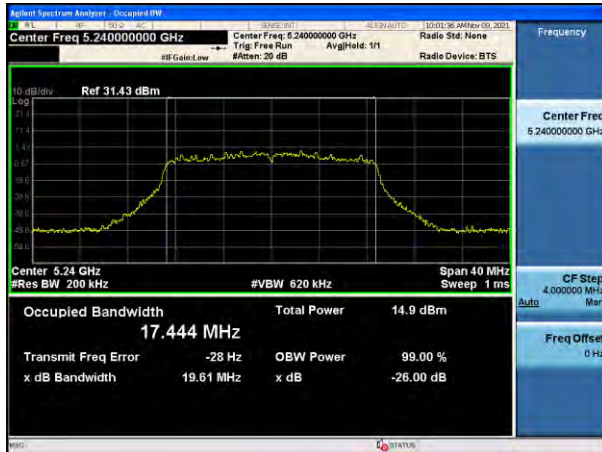
802.11ac_VHT20 UNII 2C BAND 26 dB Bandwidth(CH 100)
