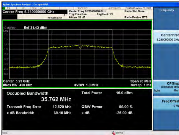
802.11n_HT40 UNII 2C BAND 26 dB Bandwidth(CH 142)
