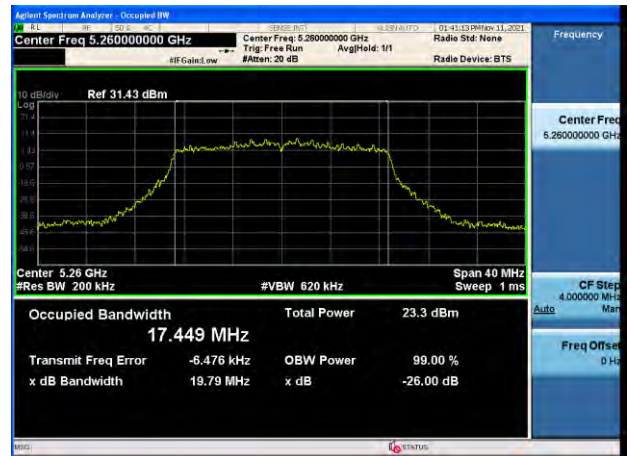
802.11ac_VHT20 UNII 3 BAND 26 dB Bandwidth(CH 165)
