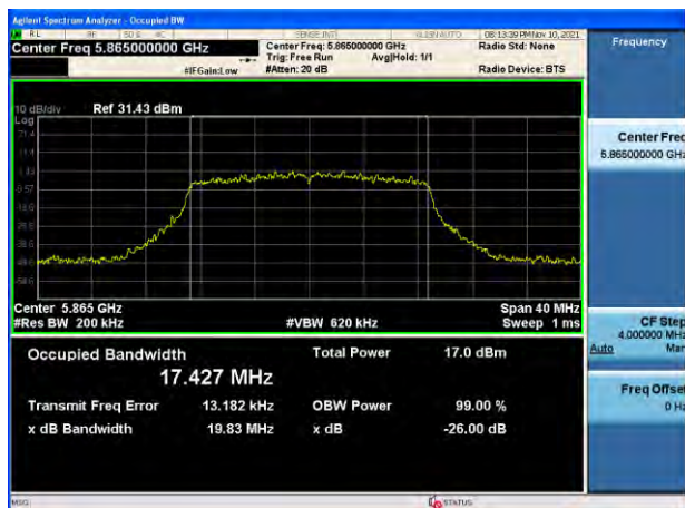
802.11n_HT20 UNII 4 BAND 26 dB Bandwidth(CH 173)
