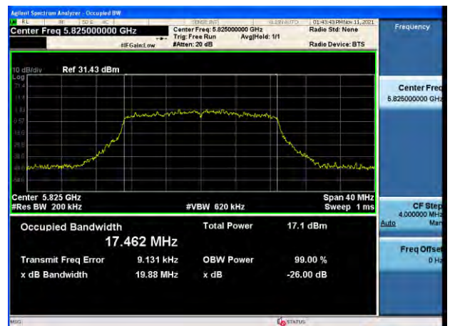
802.11ac_VHT20 UNII 3 BAND 26 dB Bandwidth(CH 165)
