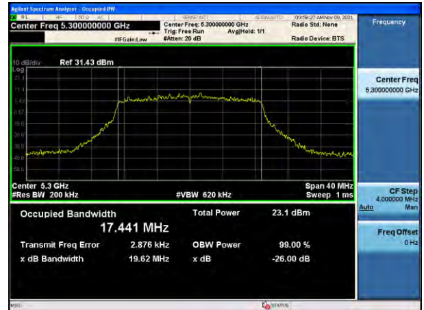
802.11n_HT20 UNII 3 BAND 26 dB Bandwidth(CH 165)
