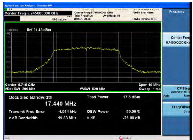
802.11n_HT20 UNII 3 BAND 26 dB Bandwidth(CH 149)
