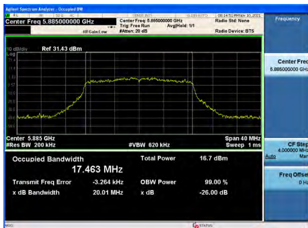
802.11ac_VHT20 UNII 4 BAND 26 dB Bandwidth(CH 177)
