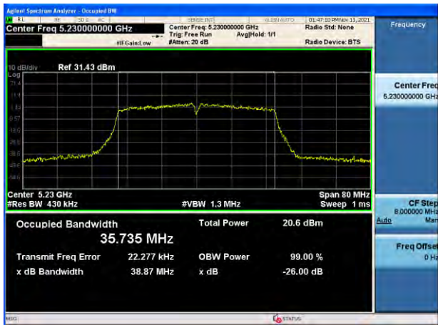
802.11ac_VHT40 UNII 2C BAND 26 dB Bandwidth(CH 142)
