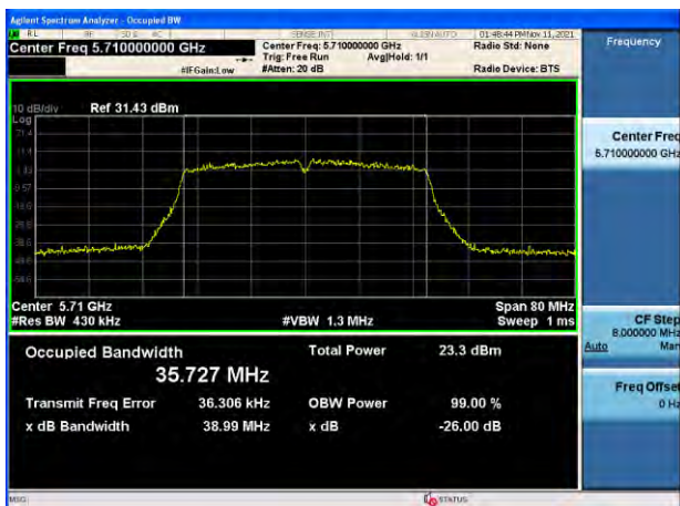
802.11ac_VHT40 UNII 4 BAND 26 dB Bandwidth (CH 175)
