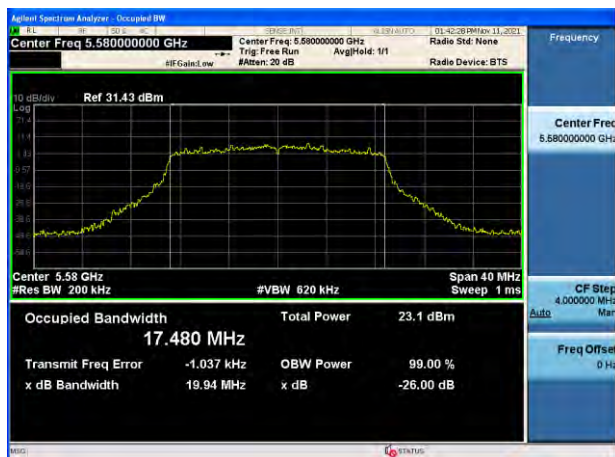
802.11ac_VHT20 UNII 4 BAND 26 dB Bandwidth(CH 177)
