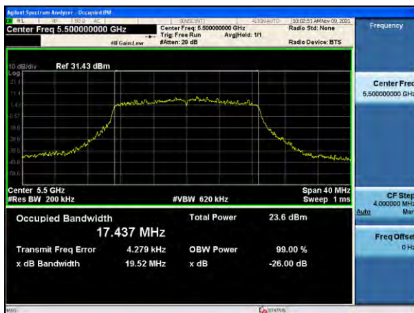
802.11ac_VHT20 UNII 4 BAND 26 dB Bandwidth(CH 173)
