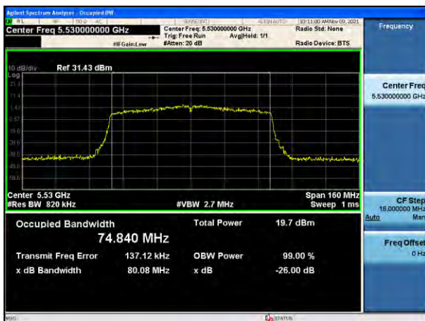
802.11ac_VHT80 UNII 4 BAND 26 dB Bandwidth (CH 171)
