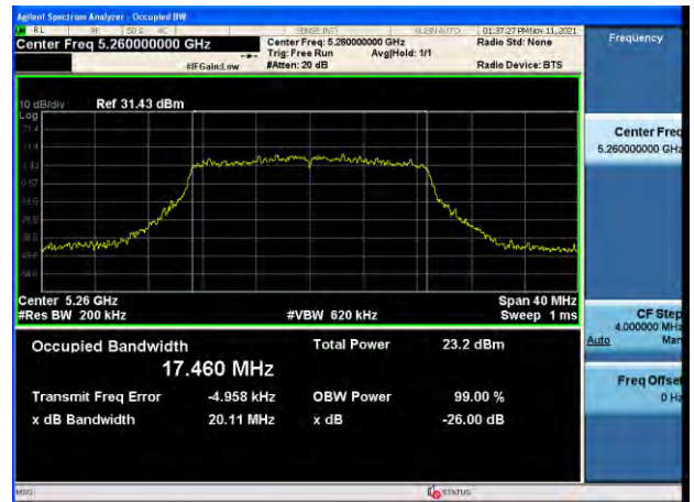
802.11n_HT20 UNII 3 BAND 26 dB Bandwidth(CH 149)
