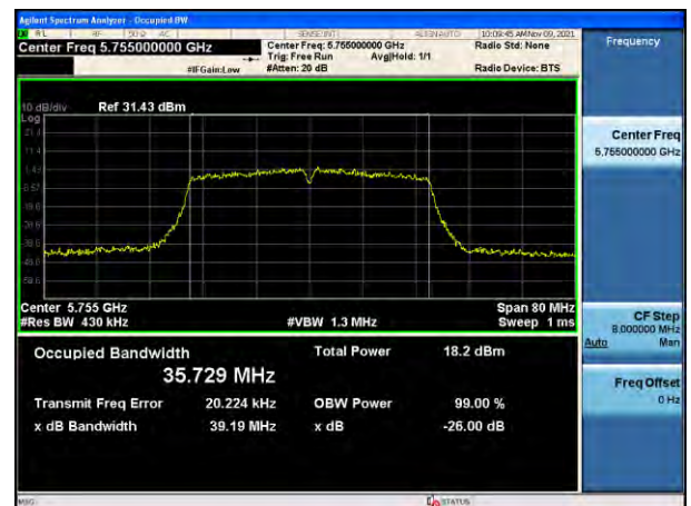
802.11ac_VHT40 UNII 3 BAND 26 dB Bandwidth (CH 151)
