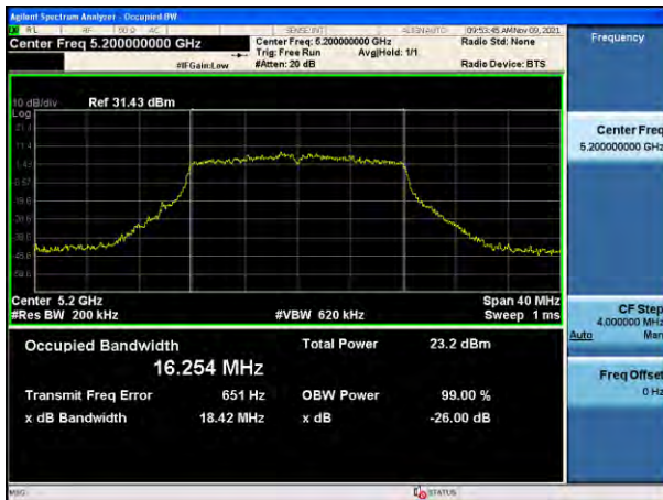
802.11a UNII 2C BAND 26 dB Bandwidth (CH 144)
