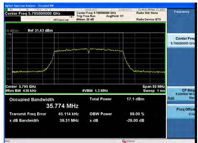
802.11ac_VHT40 UNII 3 BAND 26 dB Bandwidth (CH 159)
