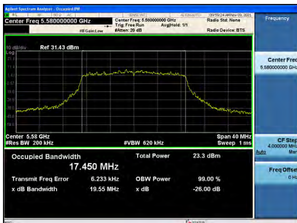
802.11n_HT20 UNII 4 BAND 26 dB Bandwidth(CH 173)
