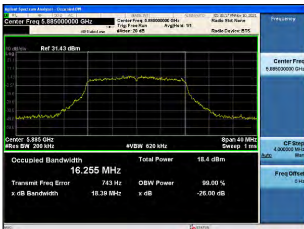
802.11a UNII 4 BAND 26 dB Bandwidth (CH 177)
