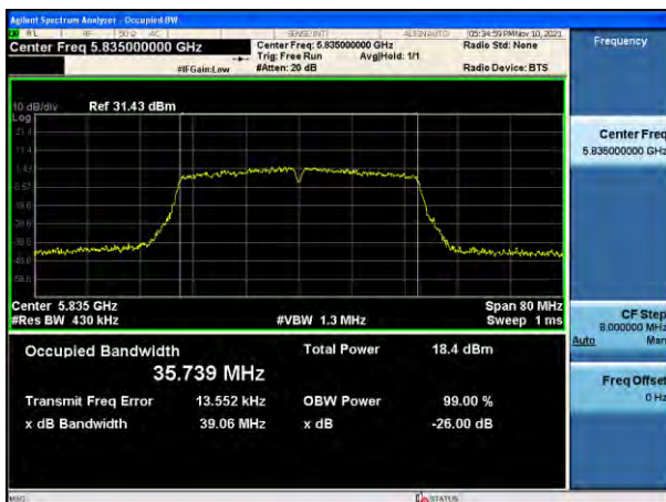
802.11ac_VHT40 UNII 4 BAND 26 dB Bandwidth (CH 167)
