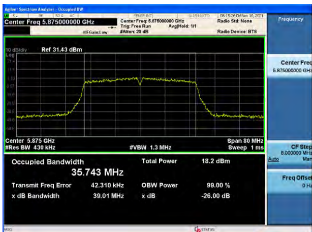
802.11n_HT40 UNII 4 BAND 26 dB Bandwidth (CH 175)
