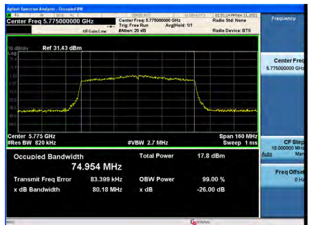
802.11ac_VHT80 UNII 3 BAND 26 dB Bandwidth (CH 155)
