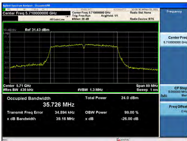
802.11n_HT40 UNII 4 BAND 26 dB Bandwidth (CH 167)
