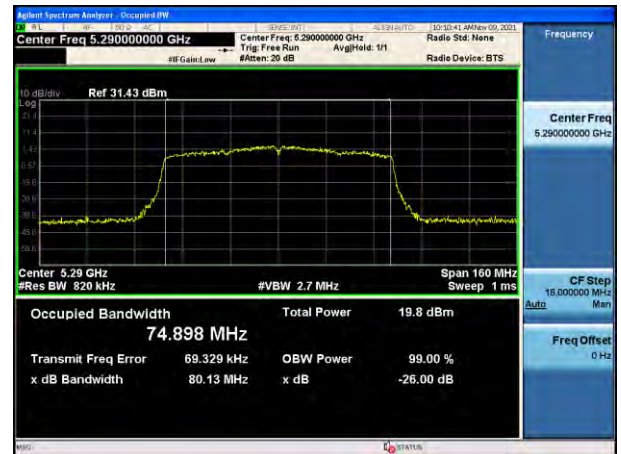
802.11ac_VHT80 UNII 3 BAND 26 dB Bandwidth (CH 155)
