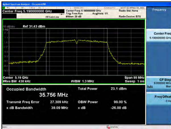
802.11ac_VHT40 UNII 2C BAND 26 dB Bandwidth(CH 142)
