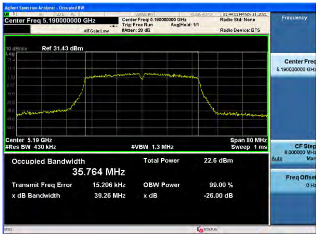
802.11n_HT40 UNII 2C BAND 26 dB Bandwidth(CH 142)
