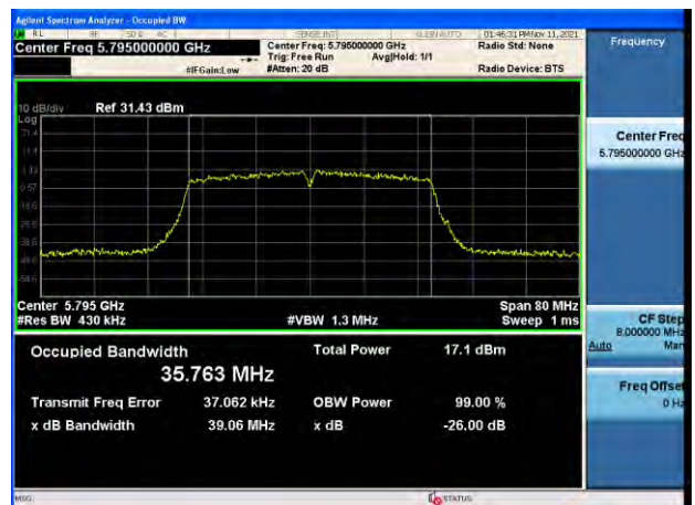
802.11n_HT40 UNII 3 BAND 26 dB Bandwidth (CH 159)
