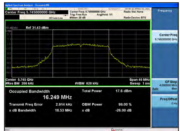
802.11a UNII 3 BAND 26 dB Bandwidth (CH 149)
