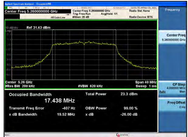
802.11ac_VHT20 UNII 3 BAND 26 dB Bandwidth(CH 157)
