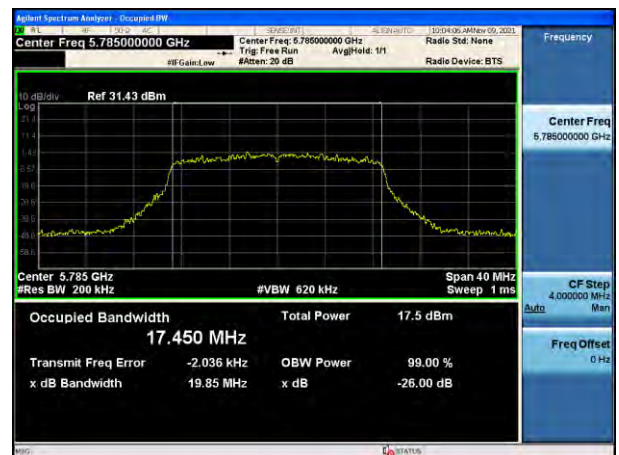
802.11ac_VHT20 UNII 3 BAND 26 dB Bandwidth(CH 157)
