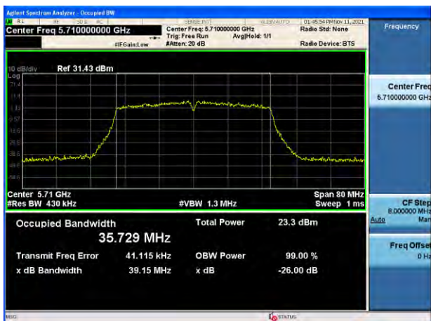
802.11n_HT40 UNII 4 BAND 26 dB Bandwidth (CH 175)
