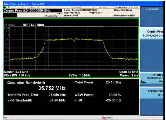
802.11n_HT40 UNII 3 BAND 26 dB Bandwidth (CH 159)
