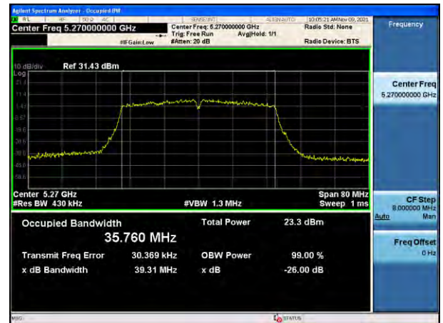
802.11n_HT40 UNII 3 BAND 26 dB Bandwidth (CH 151)
