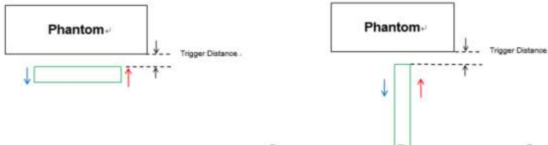
Proximity Sensor Trigger Distance Assessment KDB 616217 D04 §6.2 (Rear / Top / Right side)
