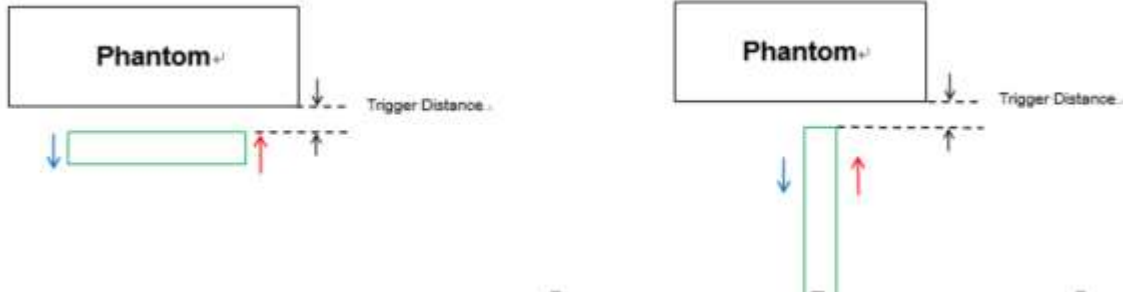
Proximity Sensor Trigger Distance Assessment KDB 616217 D04 §6.2 (Rear / Bottom / Right side)
