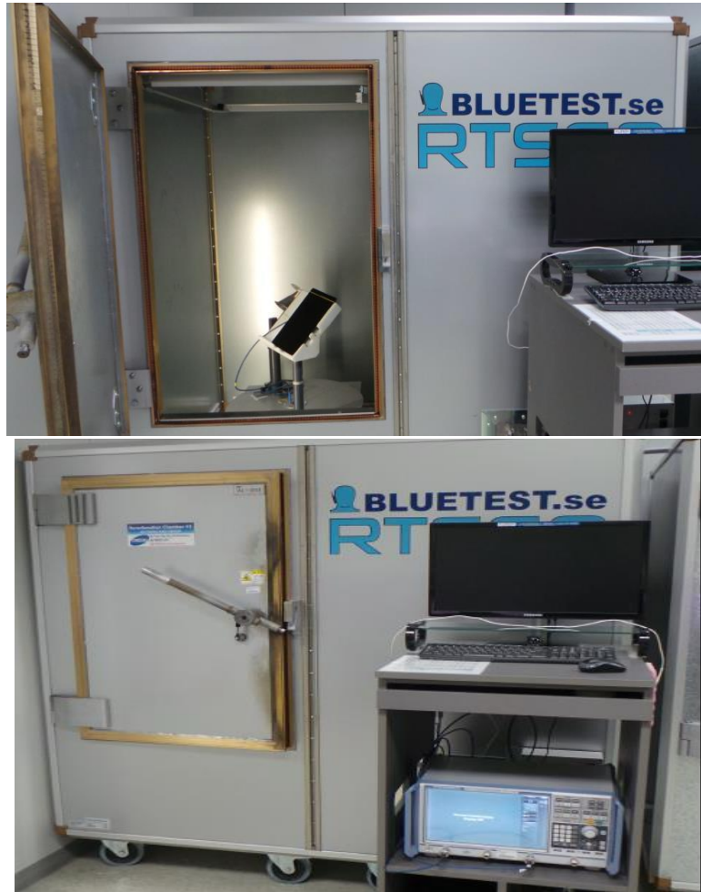
Testing with network analyzer
