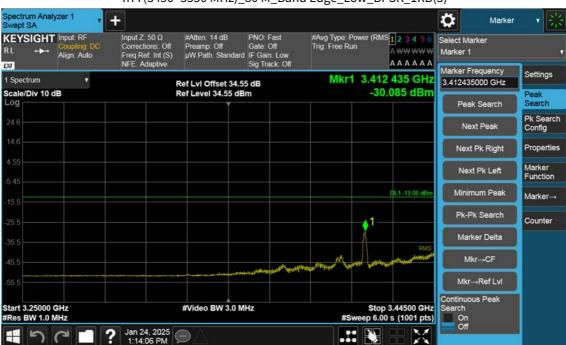
n77(3450~3550 MHz)\_80 M\_Band Edge\_Low\_BPSK\_1RB(3)
