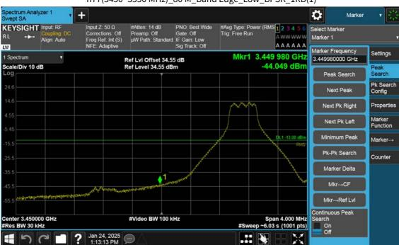
n77(3450~3550 MHz)\_80 M\_Band Edge\_Low\_BPSK\_1RB(1)
