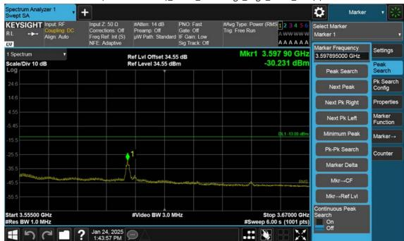
n77(3450~3550 MHz)\_100 M\_Band Edge\_High\_BPSK\_1RB(3)
