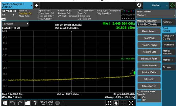
n77(3450~3550 MHz)\_70 M\_Band Edge\_Low\_BPSK\_1RB(2)
