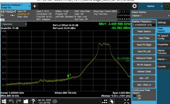
n77(3450~3550 MHz)\_70 M\_Band Edge\_Low\_BPSK\_1RB(1)
