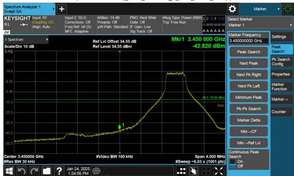
n77(3450~3550 MHz)\_90 M\_Band Edge\_Low\_BPSK\_1RB(1)
