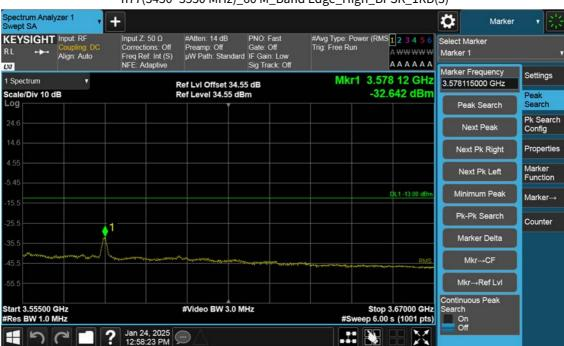
n77(3450~3550 MHz)\_60 M\_Band Edge\_High\_BPSK\_1RB(3)
