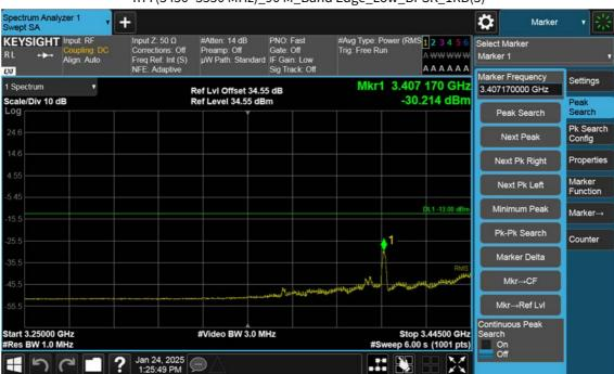
n77(3450~3550 MHz)\_90 M\_Band Edge\_Low\_BPSK\_1RB(3)
