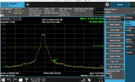
n77(3450~3550 MHz)\_80 M\_Band Edge\_High\_BPSK\_1RB(1)
