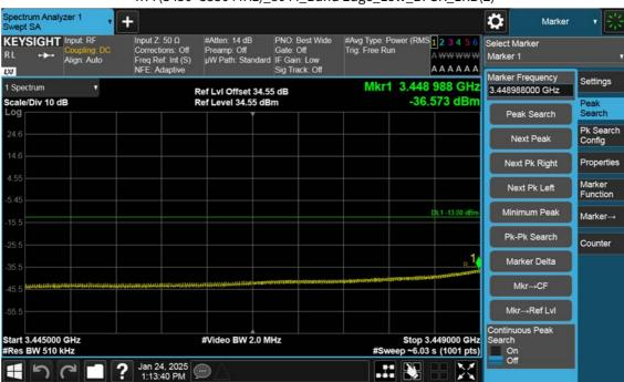
n77(3450~3550 MHz)\_80 M\_Band Edge\_Low\_BPSK\_1RB(2)
