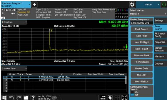
n77(3450~3550 MHz)\_30 M\_Conducted Spurious(30 M-10 G)\_High\_BPSK\_1RB
