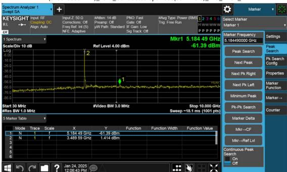
n77(3450~3550 MHz)\_20 M\_Conducted Spurious(30 M-10 G)\_Mid\_BPSK\_1RB
