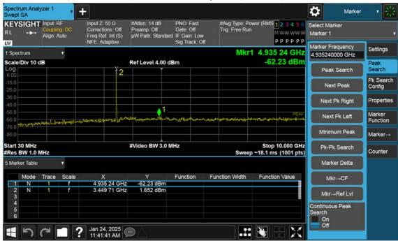
n77(3450~3550 MHz)\_10 M\_Conducted Spurious(30 M-10 G)\_Low\_BPSK\_1RB
