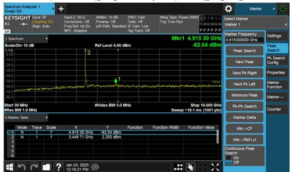
n77(3450~3550 MHz)\_30 M\_Conducted Spurious(30 M-10 G)\_Low\_BPSK\_1RB
