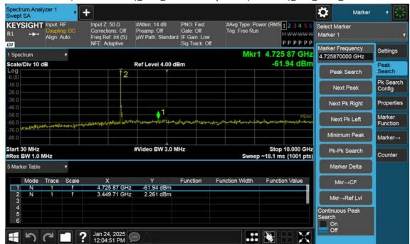
n77(3450~3550 MHz)\_20 M\_Conducted Spurious(30 M-10 G)\_Low\_BPSK\_1RB
