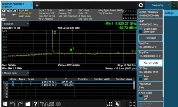
n77(3450~3550 MHz)\_25 M\_Conducted Spurious(30 M-10 G)\_Mid\_BPSK\_1RB
