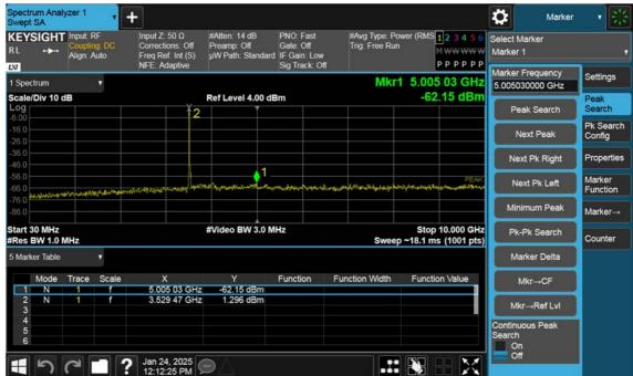
n77(3450~3550 MHz)\_20 M\_Conducted Spurious(30 M-10 G)\_High\_BPSK\_1RB
