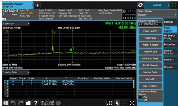
n77(3450~3550 MHz)\_40 M\_Conducted Spurious(30 M-10 G)\_Low\_BPSK\_1RB
