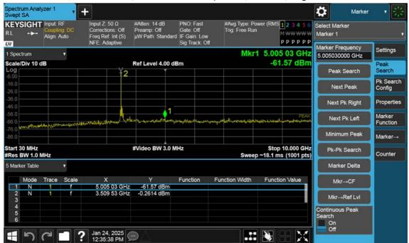
n77(3450~3550 MHz)\_40 M\_Conducted Spurious(30 M-10 G)\_High\_BPSK\_1RB
