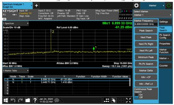
n77(3450~3550 MHz)\_15 M\_Conducted Spurious(30 M-10 G)\_Low\_BPSK\_1RB
