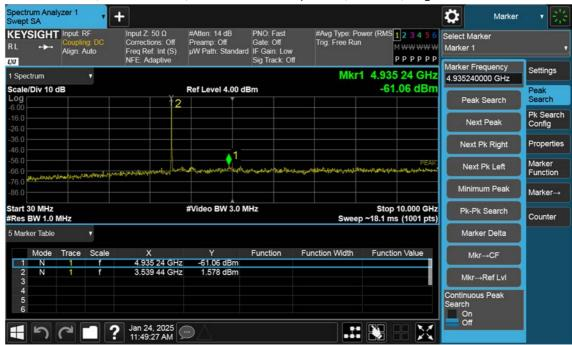
n77(3450~3550 MHz)\_10 M\_Conducted Spurious(30 M-10 G)\_High\_BPSK\_1RB
