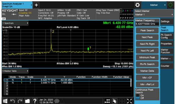
n77(3450~3550 MHz)\_50 M\_Conducted Spurious(30 M-10 G)\_Low\_BPSK\_1RB
