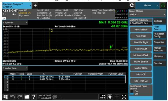
n77(3450~3550 MHz)\_10 M\_Conducted Spurious(30 M-10 G)\_Mid\_BPSK\_1RB
