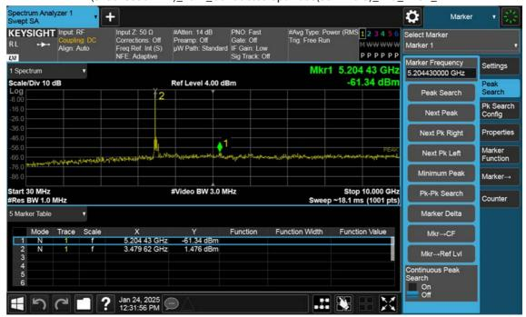
n77(3450~3550 MHz)\_40 M\_Conducted Spurious(30 M-10 G)\_Mid\_BPSK\_1RB
