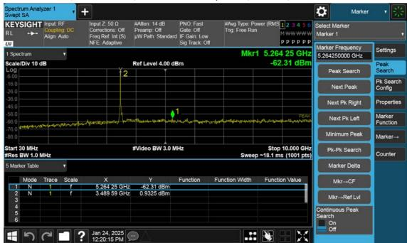
n77(3450~3550 MHz)\_30 M\_Conducted Spurious(30 M-10 G)\_Mid\_BPSK\_1RB
