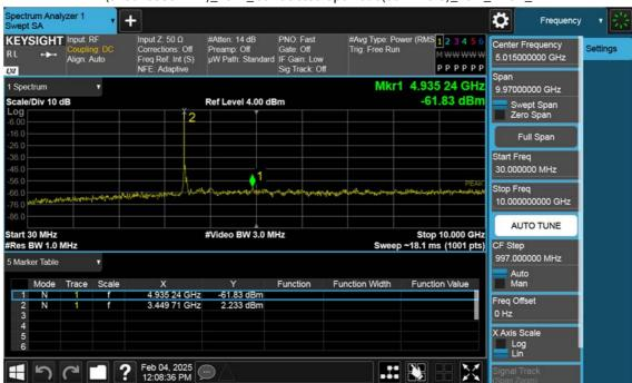
n77(3450~3550 MHz)\_25 M\_Conducted Spurious(30 M-10 G)\_Low\_BPSK\_1RB
