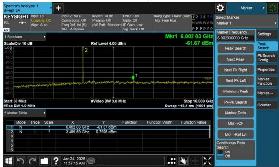
n77(3450~3550 MHz)\_15 M\_Conducted Spurious(30 M-10 G)\_Mid\_BPSK\_1RB
