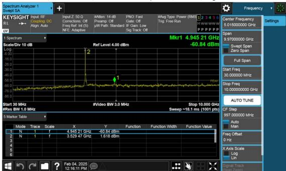
n77(3450~3550 MHz)\_25 M\_Conducted Spurious(30 M-10 G)\_High\_BPSK\_1RB
