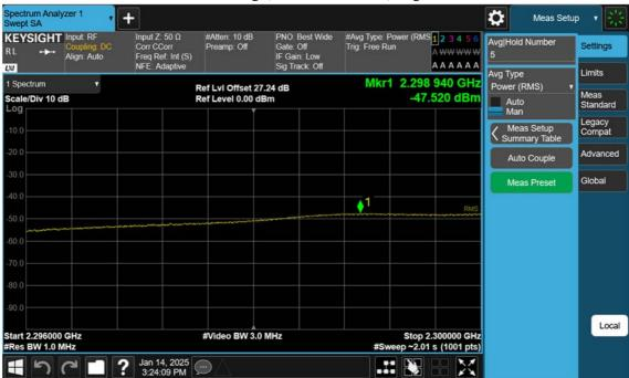
NR30\_5 M\_Band Edge(2296MHz-2300MHz)\_High\_BPSK\_1RB
