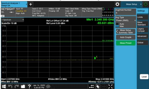
NR30\_5 M\_Band Edge(2337MHz-2341MHz)\_High\_BPSK\_1RB
