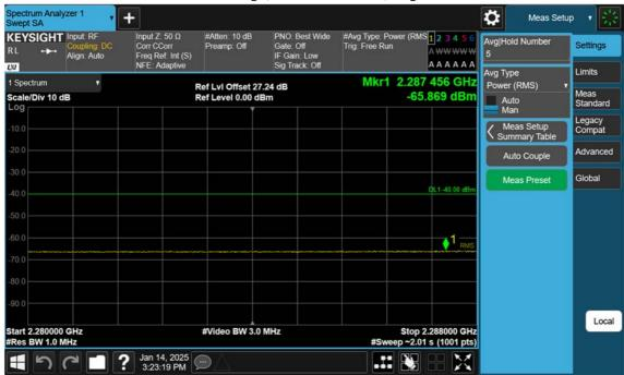
NR30\_5 M\_Band Edge(2280MHz-2288MHz)\_High\_BPSK\_1RB
