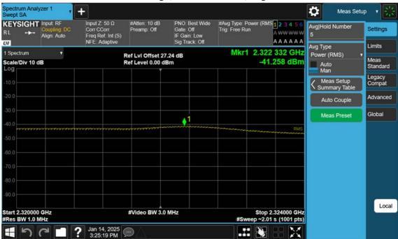
NR30\_5 M\_Band Edge(2320MHz-2324MHz)\_High\_BPSK\_1RB
