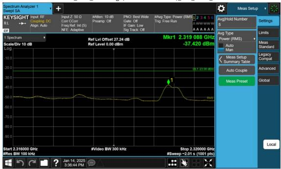
NR30\_10 M\_Band Edge(2316MHz-2320MHz)\_Mid\_BPSK\_1RB
