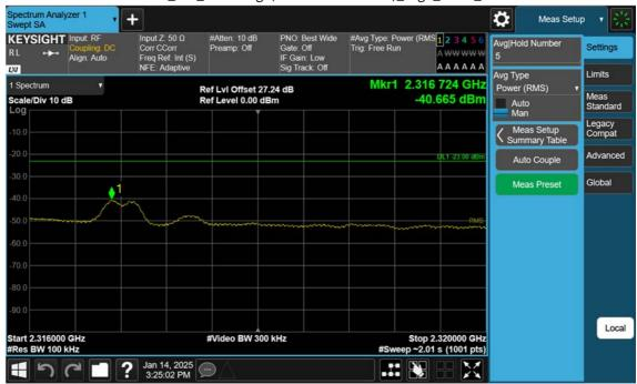
NR30\_5 M\_Band Edge(2316MHz-2320MHz)\_High\_BPSK\_1RB
