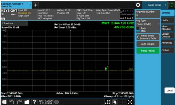
NR30\_5 M\_Band Edge(2341MHz-2345MHz)\_High\_BPSK\_1RB
