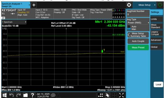
NR30\_5 M\_Band Edge(2300MHz-2305MHz)\_High\_BPSK\_1RB
