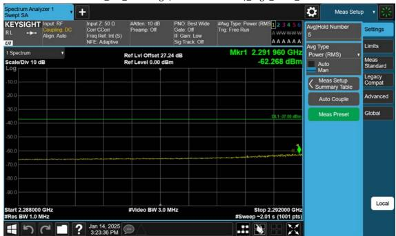
NR30\_5 M\_Band Edge(2288MHz-2292MHz)\_High\_BPSK\_1RB
