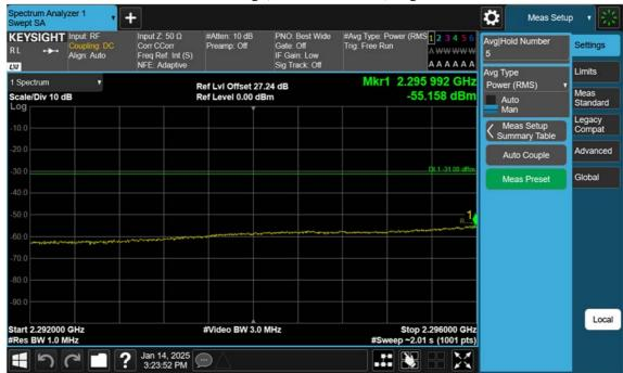
NR30\_5 M\_Band Edge(2292MHz-2296MHz)\_High\_BPSK\_1RB
