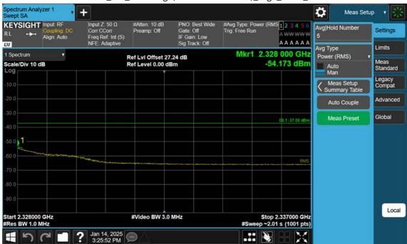
NR30\_5 M\_Band Edge(2328MHz-2337MHz)\_High\_BPSK\_1RB
