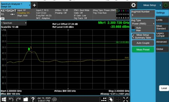
NR30\_10 M\_Band Edge(2300MHz-2304MHz)\_Mid\_BPSK\_1RB
