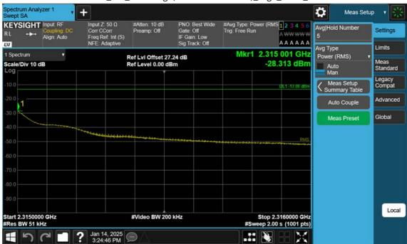
NR30\_5 M\_Band Edge(2315MHz-2316MHz)\_High\_BPSK\_1RB
