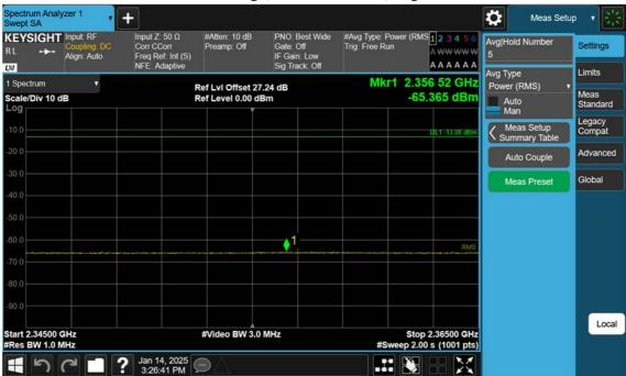
NR30\_5 M\_Band Edge(2345MHz-2365MHz)\_High\_BPSK\_1RB
