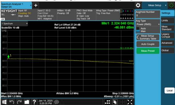
NR30\_5 M\_Band Edge(2324MHz-2328MHz)\_High\_BPSK\_1RB
