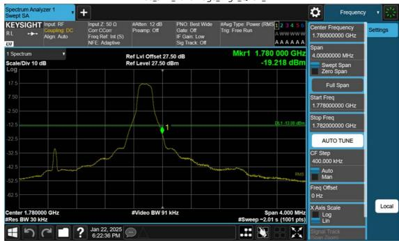
LTE B66\_3 M\_Band Edge\_High\_QPSK\_1RB
