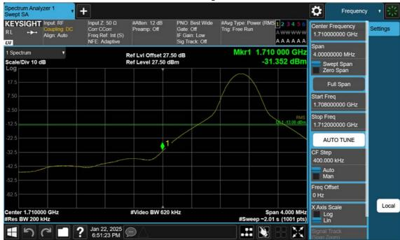
LTE B66\_20 M\_Band Edge\_Low\_QPSK\_1RB
