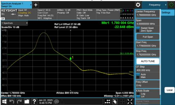
LTE B66\_15 M\_Band Edge\_High\_QPSK\_1RB
