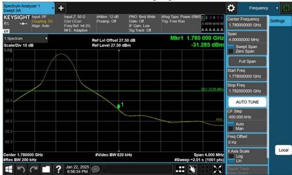
LTE B66\_20 M\_Band Edge\_High\_QPSK\_1RB
