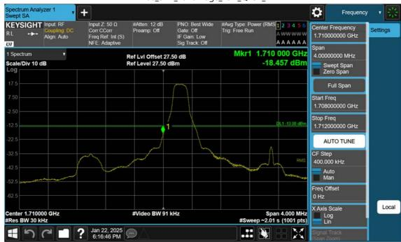
LTE B66\_3 M\_Band Edge\_Low\_QPSK\_1RB
