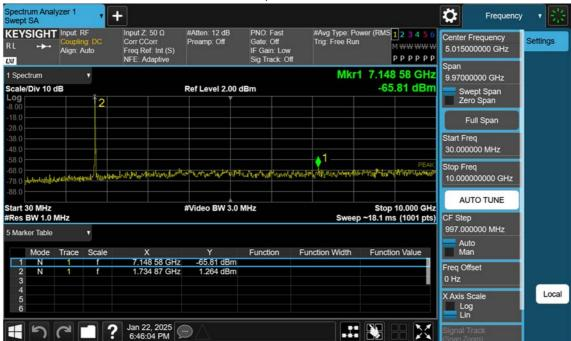
LTE B66\_15 M\_Conducted Spurious(30 M-10 G)\_Mid\_QPSK\_1RB
