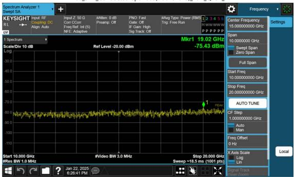
LTE B66\_5 M\_Conducted Spurious(Above10 G)\_Low\_QPSK\_1RB
