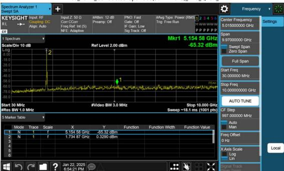
LTE B66\_20 M\_Conducted Spurious(30 M-10 G)\_Mid\_QPSK\_1RB
