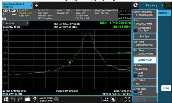
LTE B66\_10 M\_Band Edge\_Low\_QPSK\_1RB
