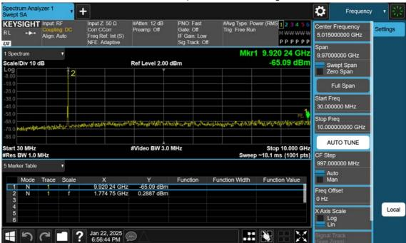
LTE B66\_20 M\_Conducted Spurious(30 M-10 G)\_High\_QPSK\_1RB
