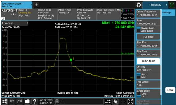
LTE B66\_1.4M\_Band Edge\_High\_QPSK\_1RB
