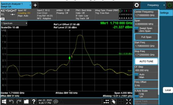
LTE B66\_5 M\_Band Edge\_Low\_QPSK\_1RB
