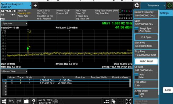
LTE B66\_15 M\_Conducted Spurious(30 M-10 G)\_Low\_QPSK\_1RB
