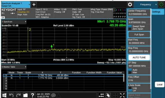
LTE B66\_15 M\_Conducted Spurious(30 M-10 G)\_High\_QPSK\_1RB
