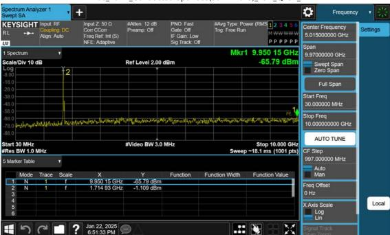
LTE B66\_20 M\_Conducted Spurious(30 M-10 G)\_Low\_QPSK\_1RB
