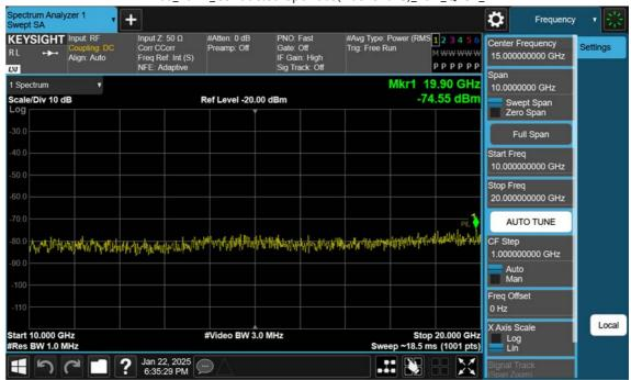
LTE B66\_10 M\_Conducted Spurious(Above10 G)\_Low\_QPSK\_1RB
