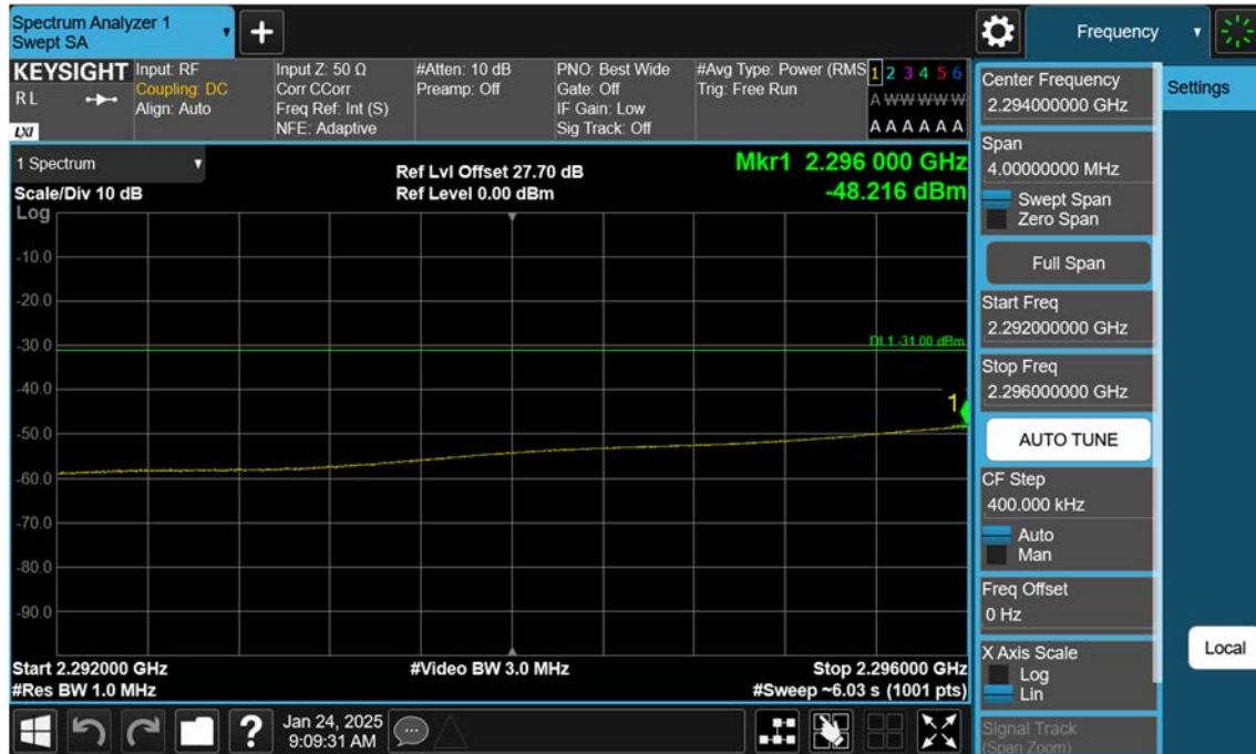
LTE B30_5 M_Band Edge(2292MHz-2296MHz)_Mid_QPSK_FullIRB
