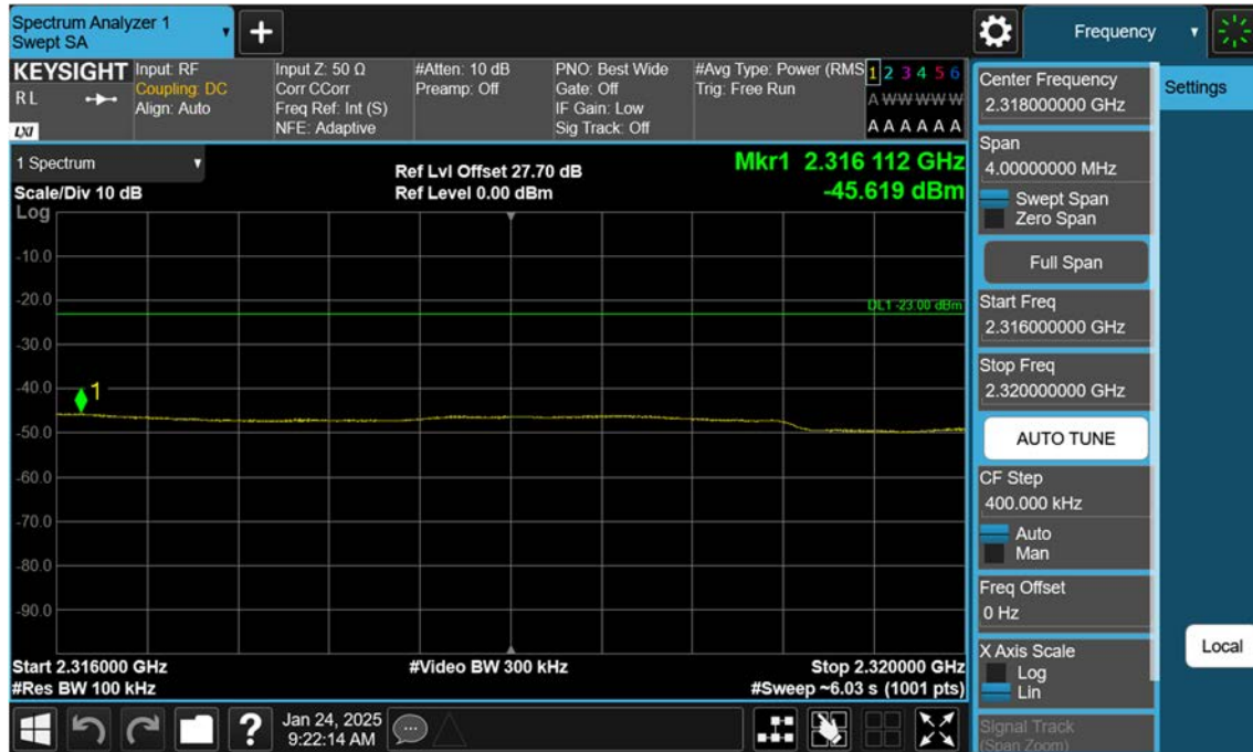
LTE B30_5 M_Band Edge(2316MHz-2320MHz)_High_QPSK_FullIRB
