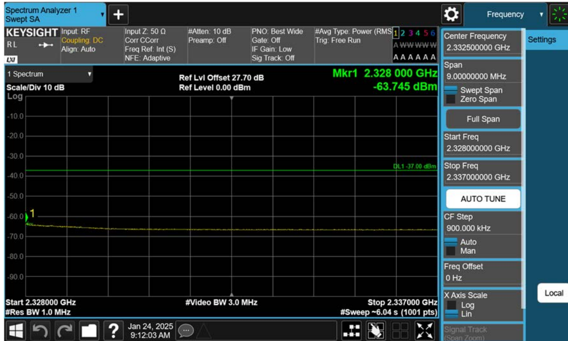
LTE B30_5 M_Band Edge(2328MHz-2337MHz)_Mid_QPSK_FullIRB
