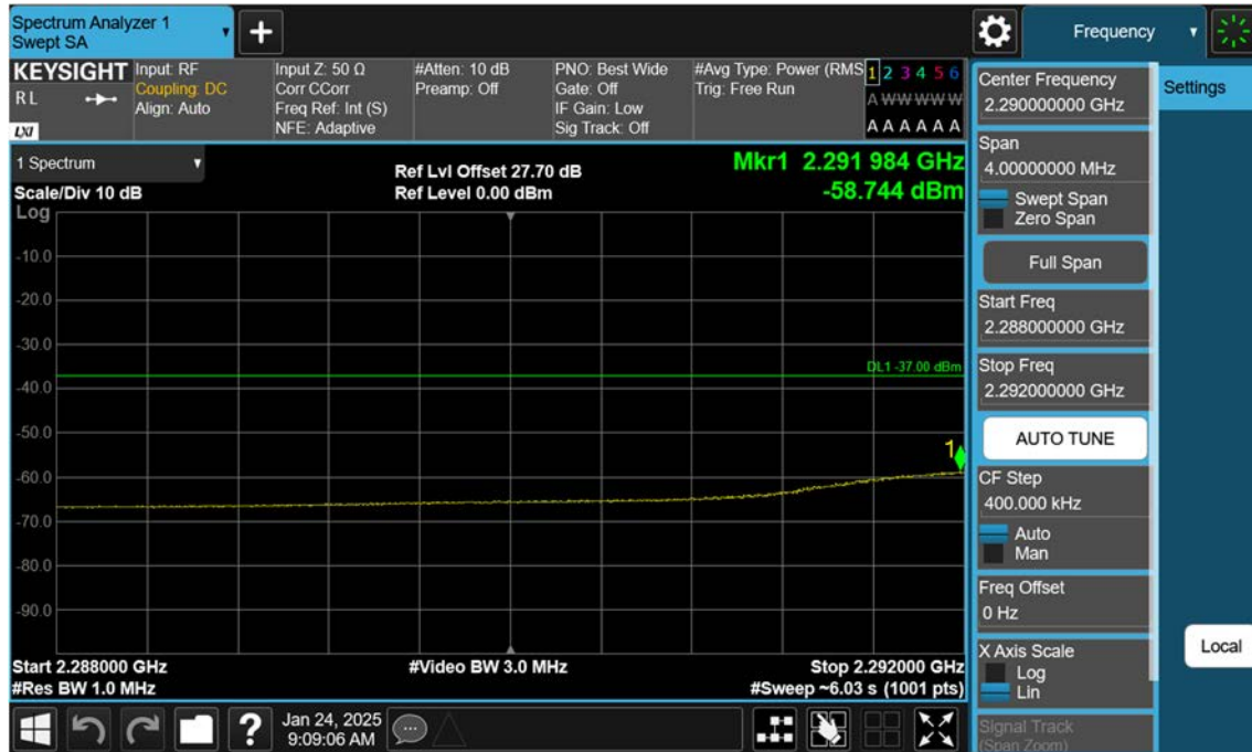
LTE B30_5 M_Band Edge(2288MHz-2292MHz)_Mid_QPSK_FullIRB
