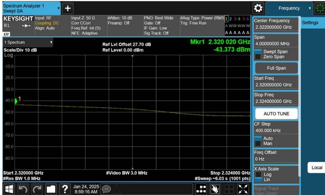
LTE B30_5 M_Band Edge(2320MHz-2324MHz)_Low_QPSK_FullIRB
