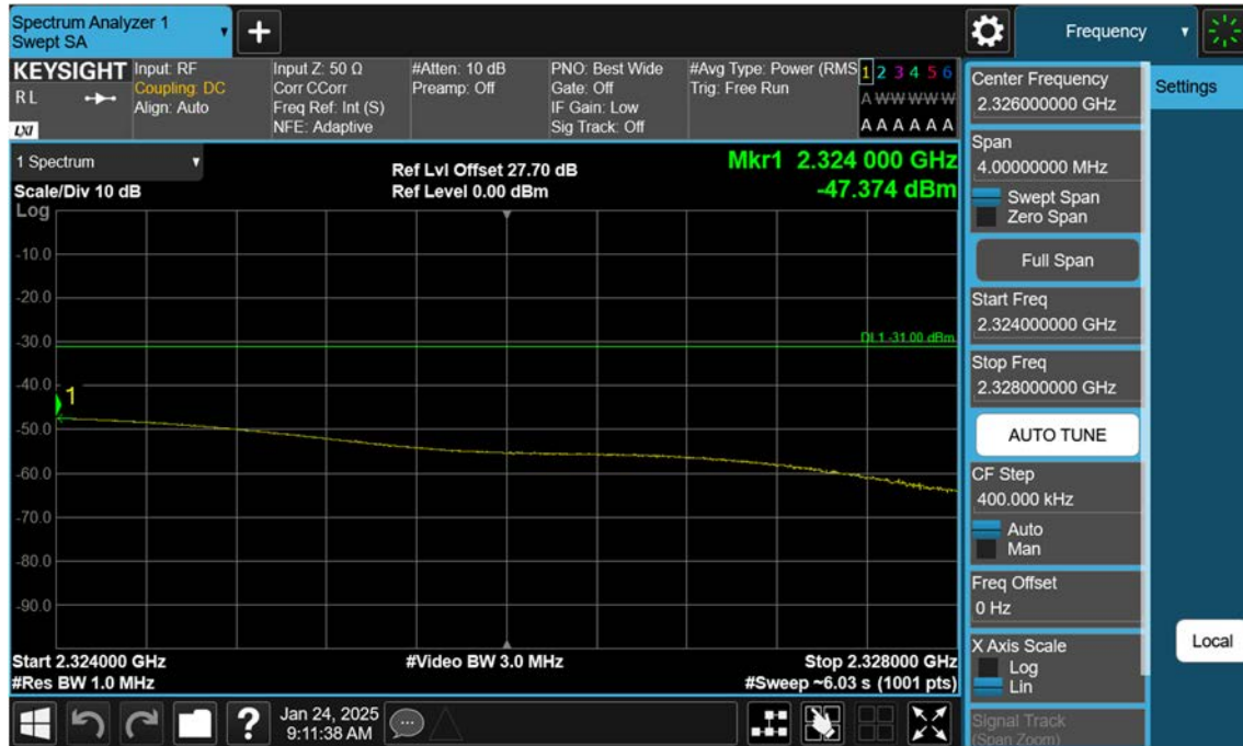
LTE B30_5 M_Band Edge(2324MHz-2328MHz)_Mid_QPSK_FullIRB
