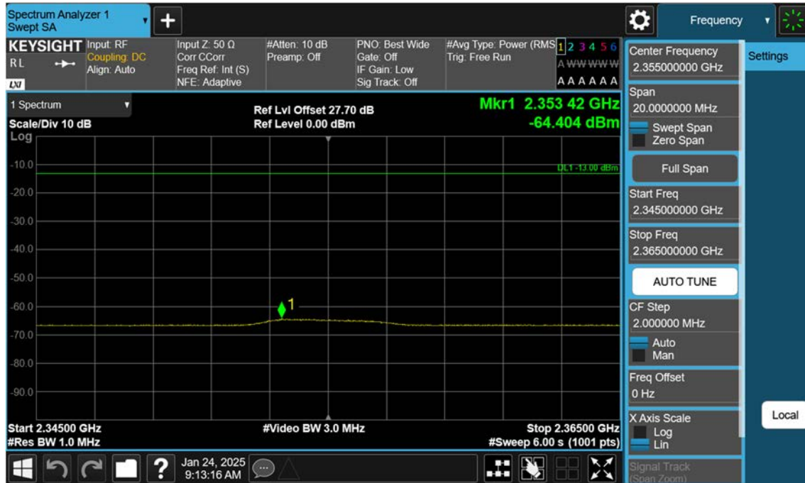
LTE B30_5 M_Band Edge(2345MHz-2365MHz)_Mid_QPSK_FullRB
