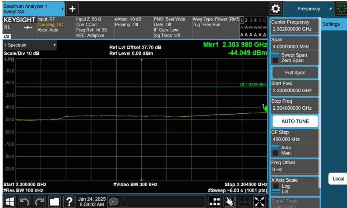
LTE B30_5 M_Band Edge(2300MHz-2304MHz)_Low_QPSK_FullIRB
