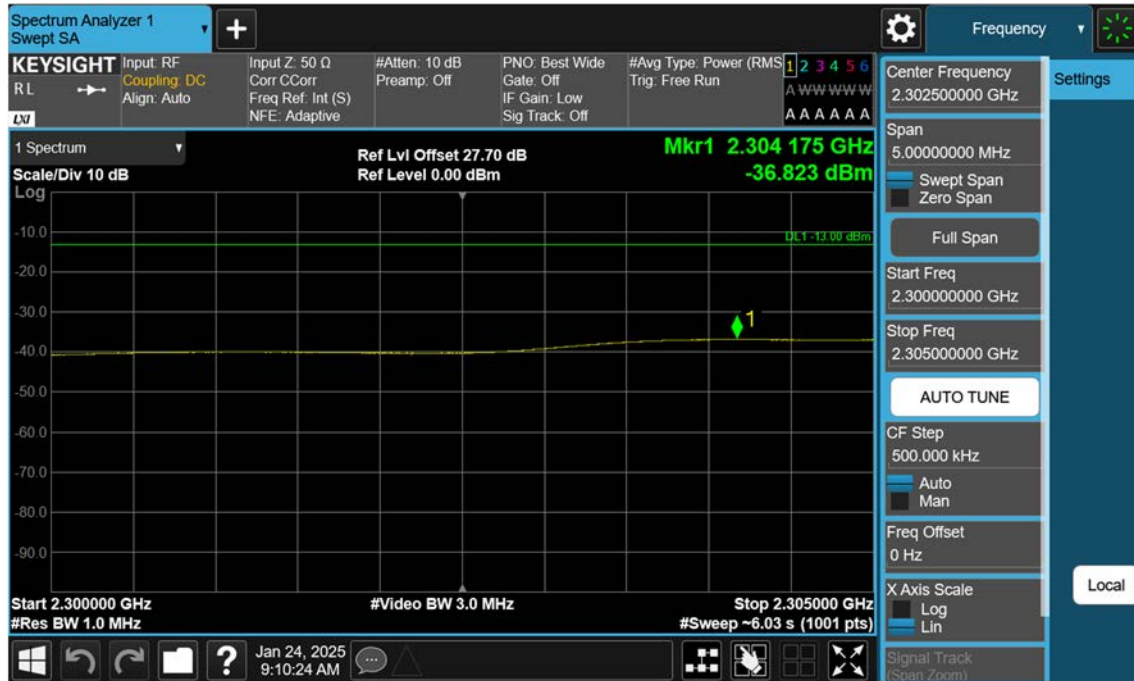
LTE B30_5 M_Band Edge(2300MHz-2305MHz)_Mid_QPSK_FullIRB
