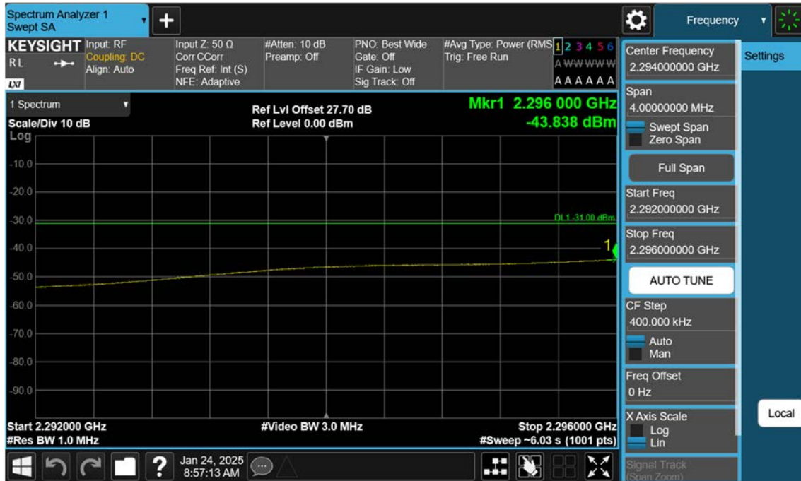
LTE B30_5 M_Band Edge(2292MHz-2296MHz)_Low_QPSK_FullIRB
