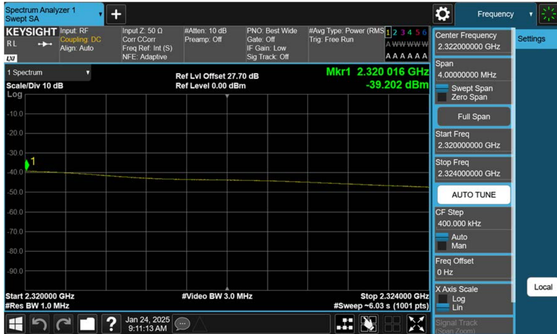
LTE B30_5 M_Band Edge(2320MHz-2324MHz)_Mid_QPSK_FullIRB
