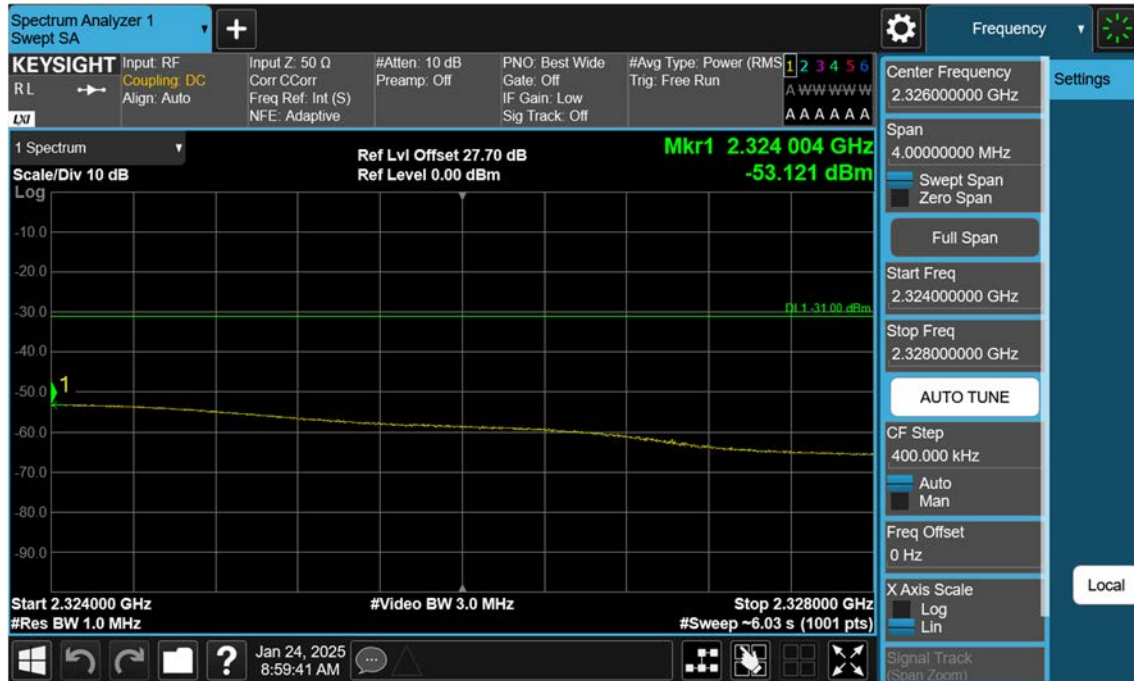
LTE B30_5 M_Band Edge(2324MHz-2328MHz)_Low_QPSK_FullIRB
