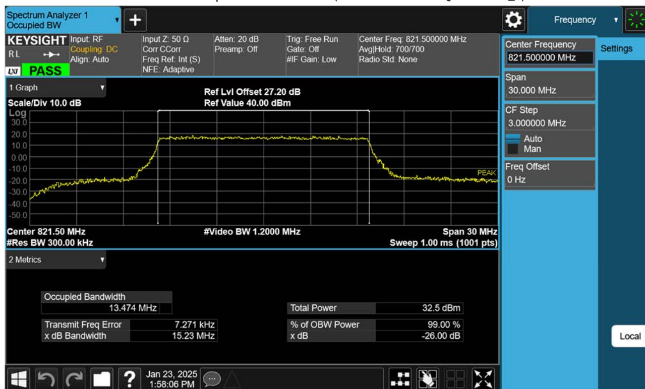
BAND 26. Occupied Bandwidth Plot (15 M BW Ch.26765 QPSK RB 75_0)
