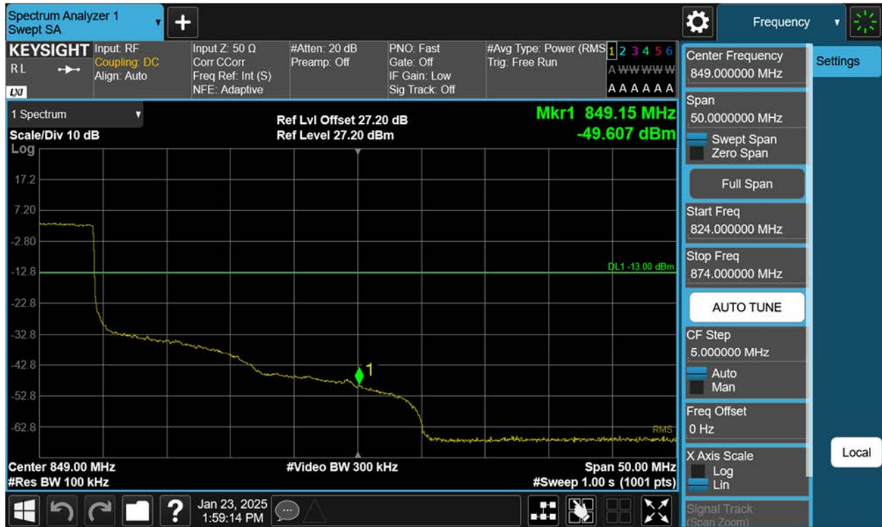
BAND 26. Mid Band Edge Plot (15 M BW Ch.26765 QPSK_RB75_Offset 0)
