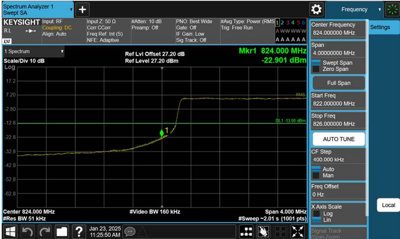
BAND 26. Lower Band Edge Plot (5 M BW Ch.26815 QPSK_RB25_Offset 0)
