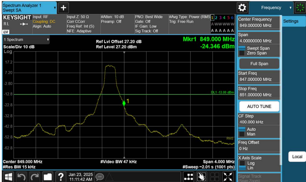
BAND 26. Upper Band Edge Plot (1.4 M BW Ch.27033 QPSK_RB1_Offset 5)
