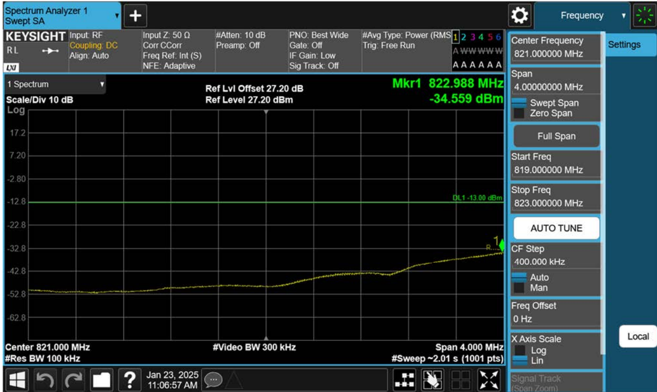
BAND 26. Lower Extended Band Edge Plot (1.4 M BW Ch.26797 QPSK_RB6_0)
