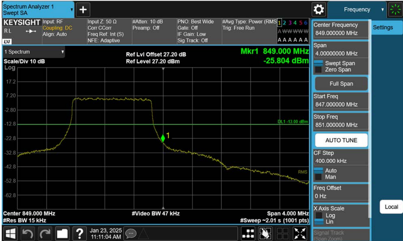
BAND 26. Upper Band Edge Plot (1.4 M BW Ch.27033 QPSK_RB6_Offset 0)
