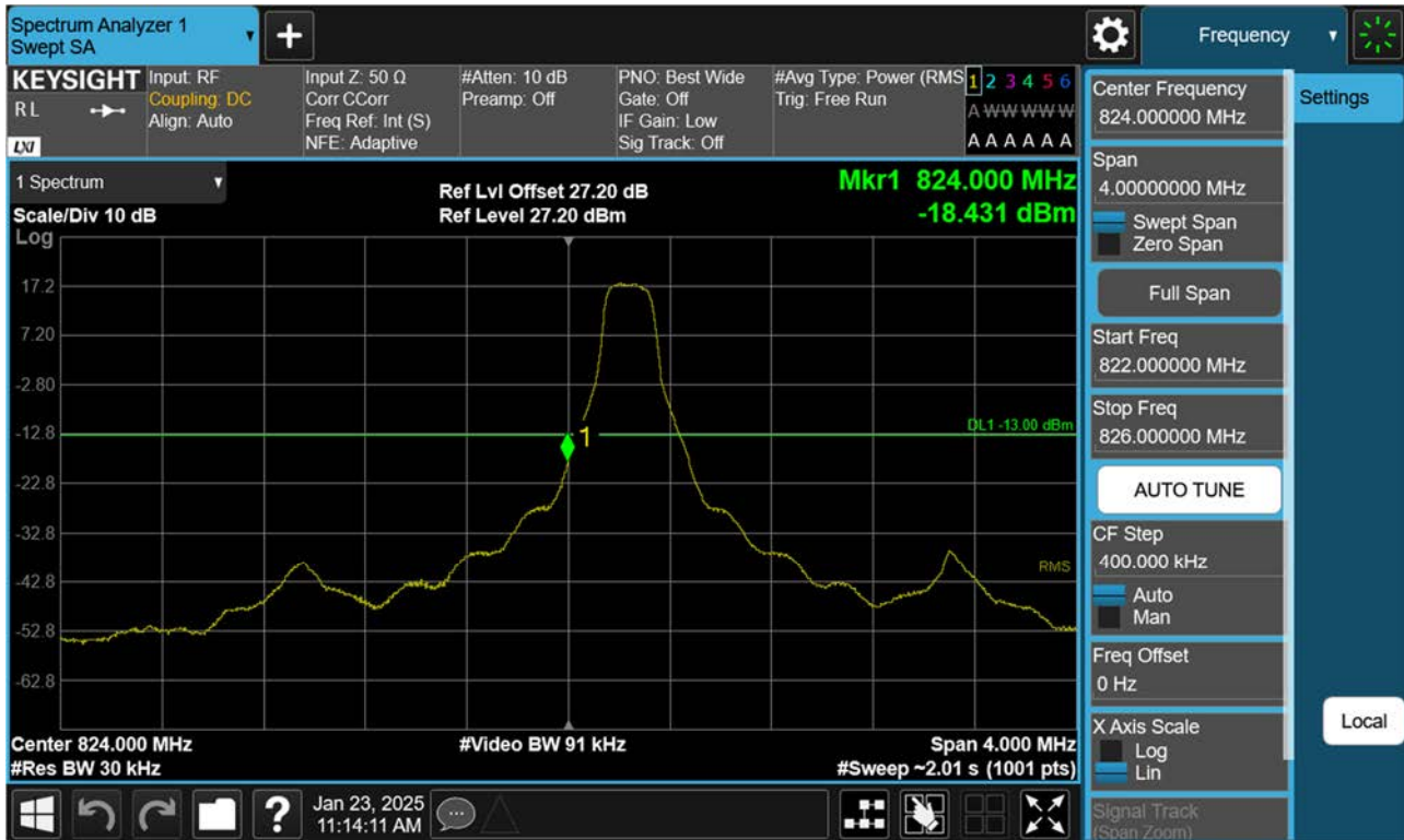
BAND 26. Lower Band Edge Plot (3 M BW Ch.26805 QPSK_RB1_Offset 0)
