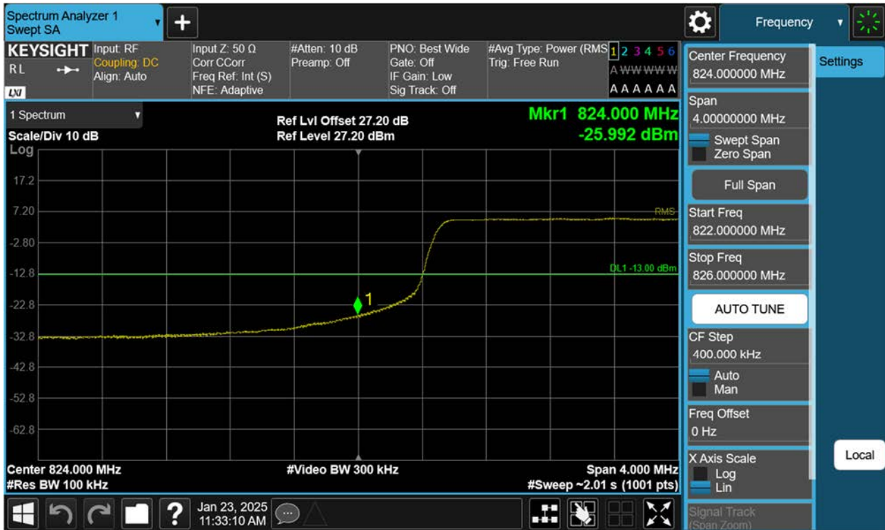
BAND 26. Lower Band Edge Plot (10 M BW Ch.26840 QPSK_RB50_Offset 0)
