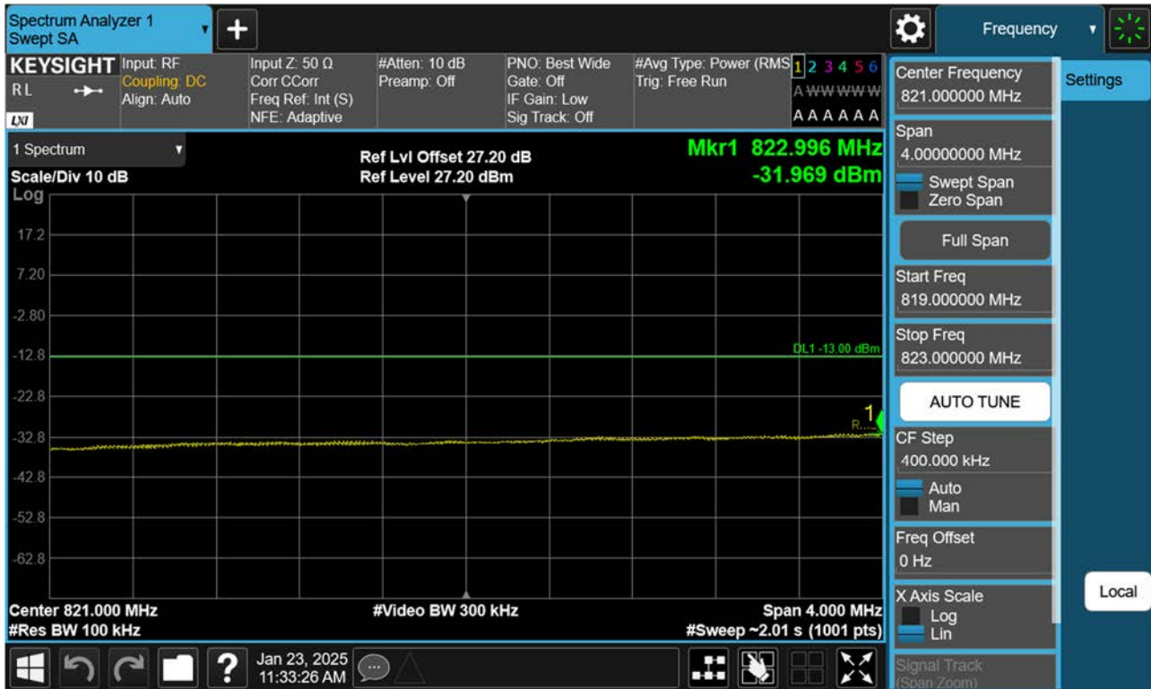
BAND 26. Lower Extended Band Edge Plot (10 M BW Ch.26840 QPSK_RB50_0)
