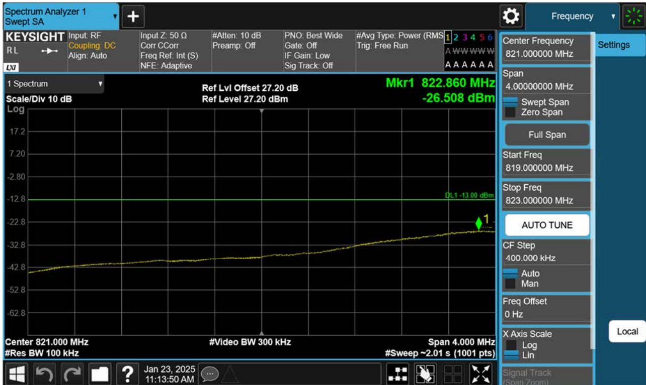
BAND 26. Lower Extended Band Edge Plot (3 M BW Ch.26805 QPSK_RB15_0)
