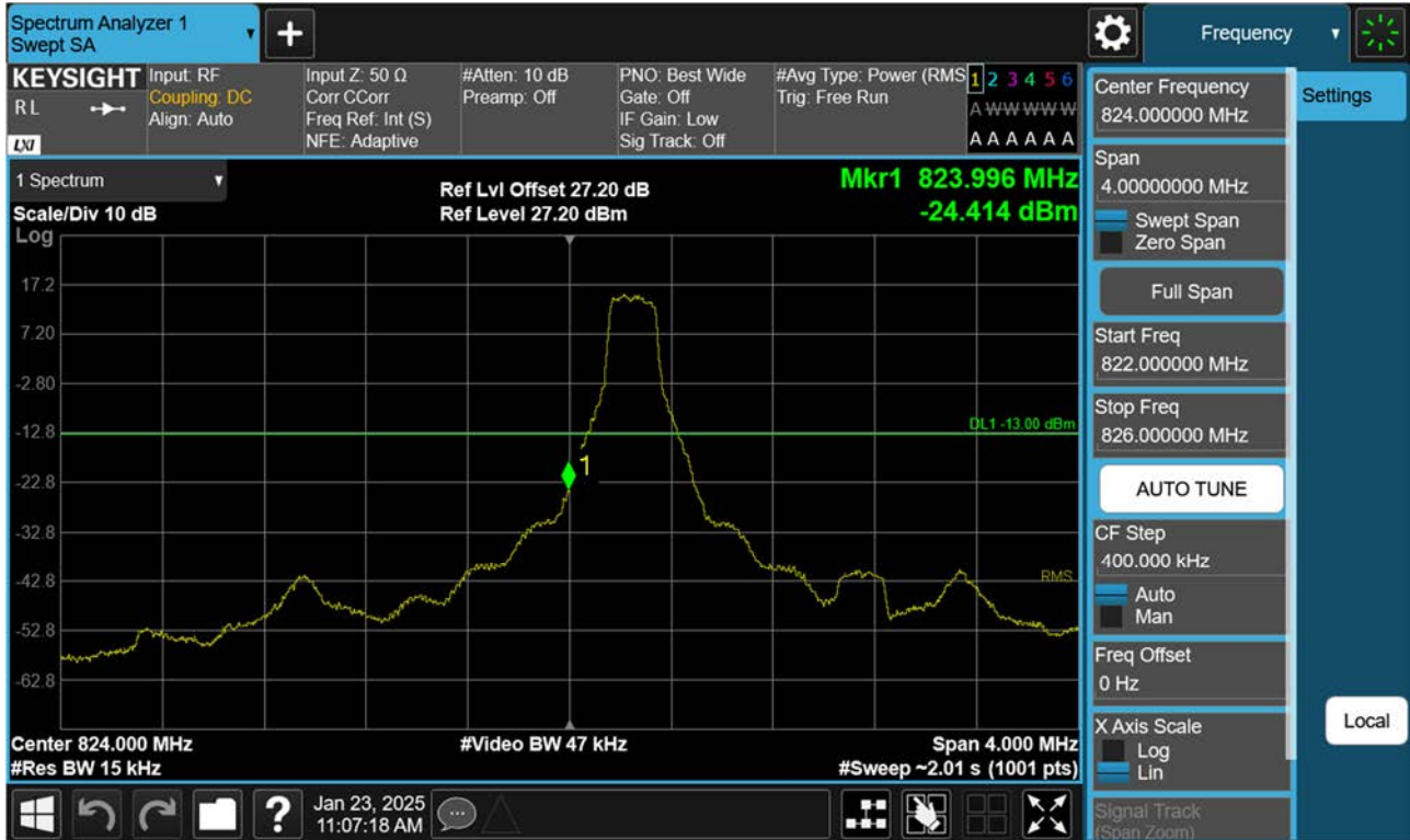
BAND 26. Lower Band Edge Plot (1.4 M BW Ch.26797 QPSK_RB1_Offset 0)
