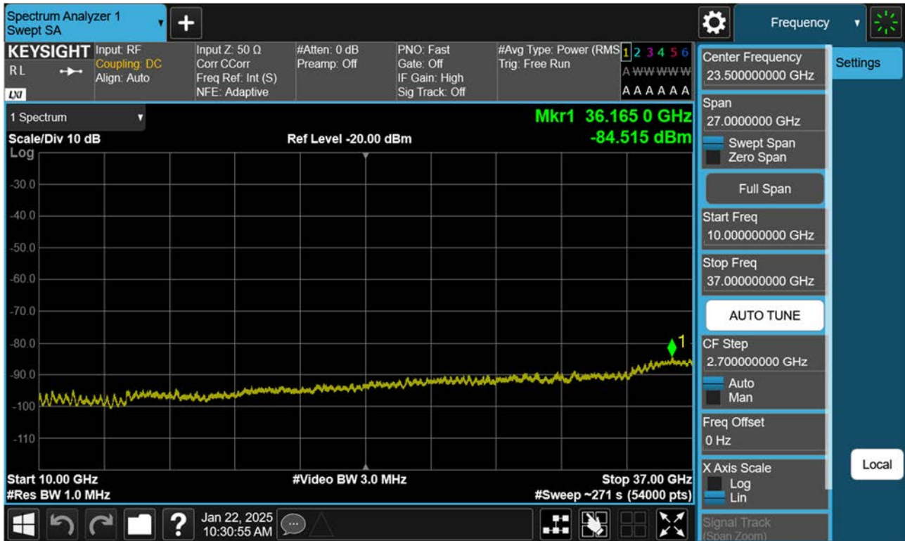
BAND 48. Conducted Spurious Plot 2 (10 MHz Ch. 55990 QPSK RB 1, Offset 0)
