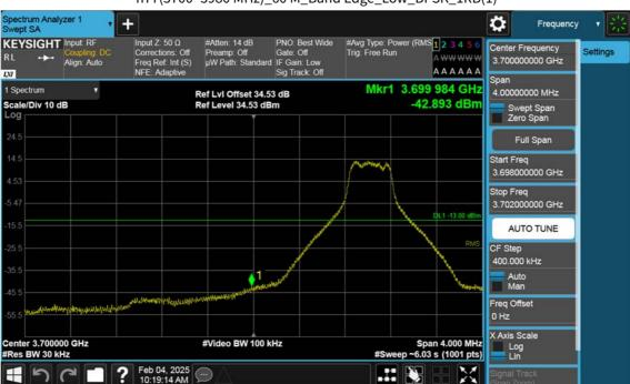
n77(3700~3980 MHz)\_60 M\_Band Edge\_Low\_BPSK\_1RB(1)
