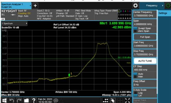
n77(3700~3980 MHz)\_90 M\_Band Edge\_Low\_BPSK\_1RB(1)
