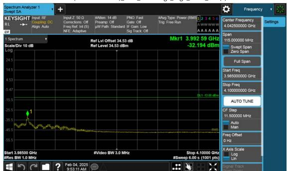
n77(3700~3980 MHz)\_30 M\_Band Edge\_High\_BPSK\_1RB(3)
