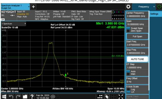
n77(3700~3980 MHz)\_50 M\_Band Edge\_High\_BPSK\_1RB(1)
