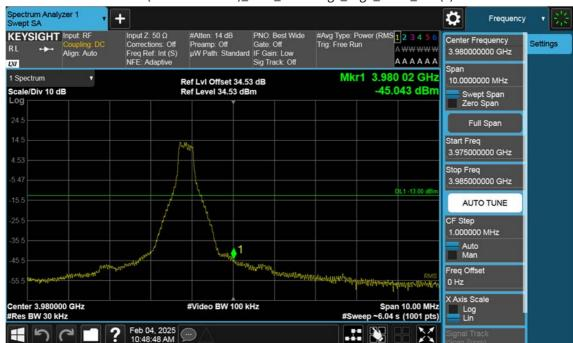
n77(3700~3980 MHz)\_80 M\_Band Edge\_High\_BPSK\_1RB(1)
