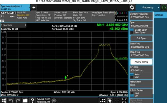
n77(3700~3980 MHz)\_50 M\_Band Edge\_Low\_BPSK\_1RB(1)
