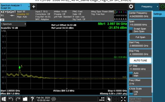
n77(3700~3980 MHz)\_40 M\_Band Edge\_High\_BPSK\_1RB(3)
