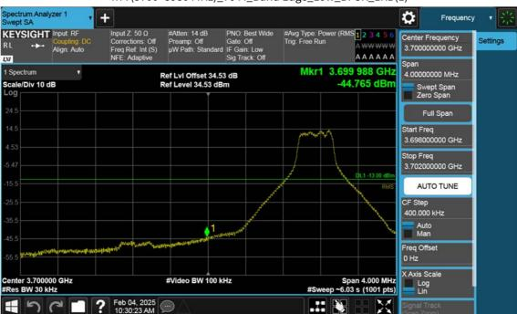
n77(3700~3980 MHz)\_70 M\_Band Edge\_Low\_BPSK\_1RB(1)
