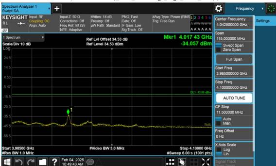
n77(3700~3980 MHz)\_80 M\_Band Edge\_High\_BPSK\_1RB(3)
