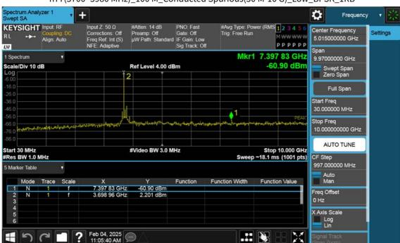
n77(3700~3980 MHz)\_100 M\_Conducted Spurious(30 M-10 G)\_Low\_BPSK\_1RB
