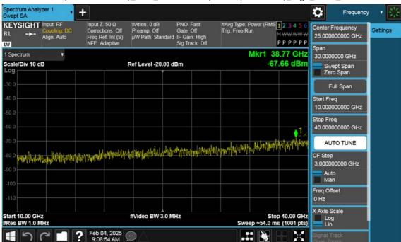
n77(3700~3980 MHz)\_10 M\_Conducted Spurious(Above10 G)\_High\_BPSK\_1RB
