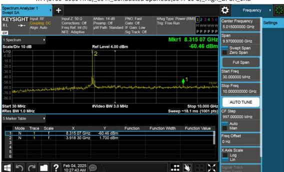
n77(3700~3980 MHz)\_60 M\_Conducted Spurious(30 M-10 G)\_High\_BPSK\_1RB
