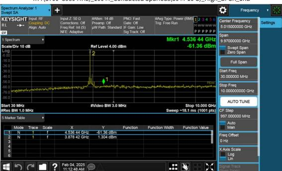
n77(3700~3980 MHz)\_100 M\_Conducted Spurious(30 M-10 G)\_High\_BPSK\_1RB
