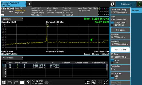
n77(3700~3980 MHz)\_70 M\_Conducted Spurious(30 M-10 G)\_High\_BPSK\_1RB
