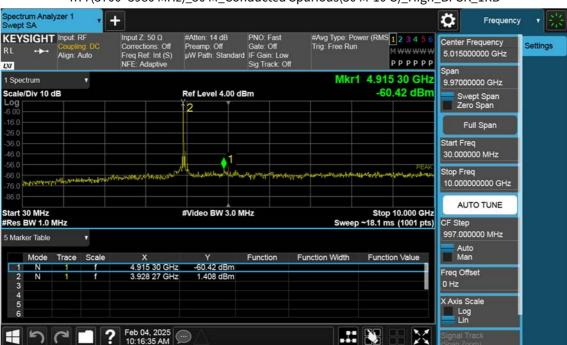
n77(3700~3980 MHz)\_50 M\_Conducted Spurious(30 M-10 G)\_High\_BPSK\_1RB
