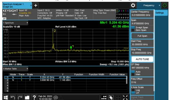
n77(3700~3980 MHz)\_80 M\_Conducted Spurious(30 M-10 G)\_Low\_BPSK\_1RB
