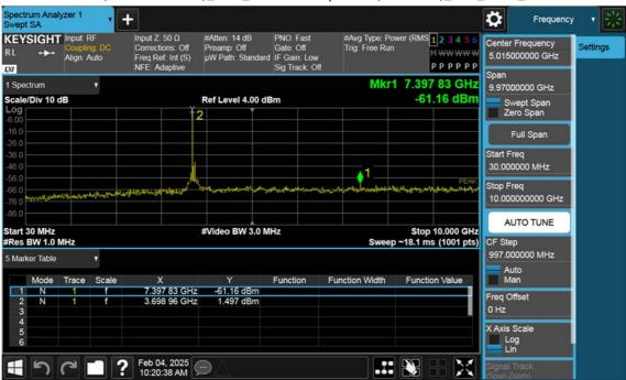
n77(3700~3980 MHz)\_60 M\_Conducted Spurious(30 M-10 G)\_Low\_BPSK\_1RB
