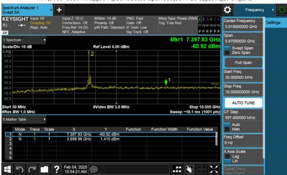
n77(3700~3980 MHz)\_90 M\_Conducted Spurious(30 M-10 G)\_Low\_BPSK\_1RB
