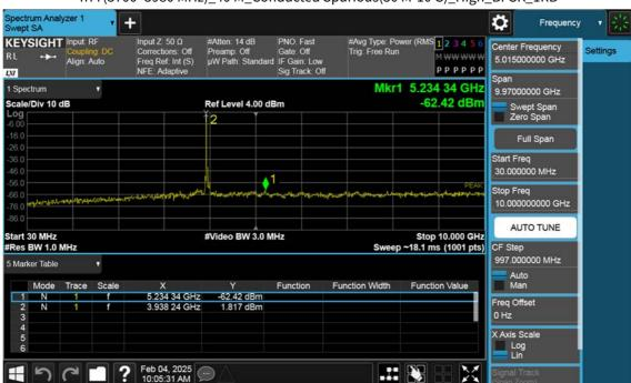
n77(3700~3980 MHz)\_40 M\_Conducted Spurious(30 M-10 G)\_High\_BPSK\_1RB
