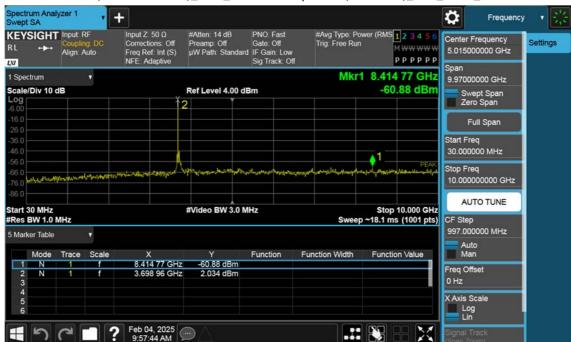
n77(3700~3980 MHz)\_40 M\_Conducted Spurious(30 M-10 G)\_Low\_BPSK\_1RB
