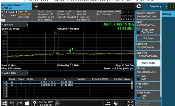
n77(3700~3980 MHz)\_25 M\_Conducted Spurious(30 M-10 G)\_Low\_BPSK\_1RB
