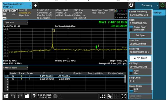
n77(3700~3980 MHz)\_50 M\_Conducted Spurious(30 M-10 G)\_Low\_BPSK\_1RB
