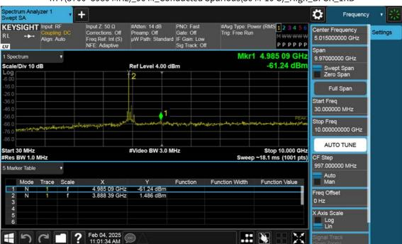
n77(3700~3980 MHz)\_90 M\_Conducted Spurious(30 M-10 G)\_High\_BPSK\_1RB
