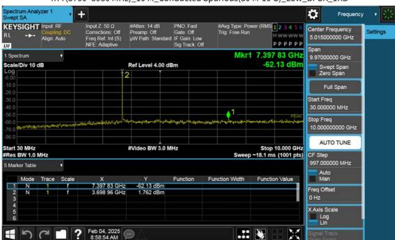
n77(3700~3980 MHz)\_10 M\_Conducted Spurious(30 M-10 G)\_Low\_BPSK\_1RB
