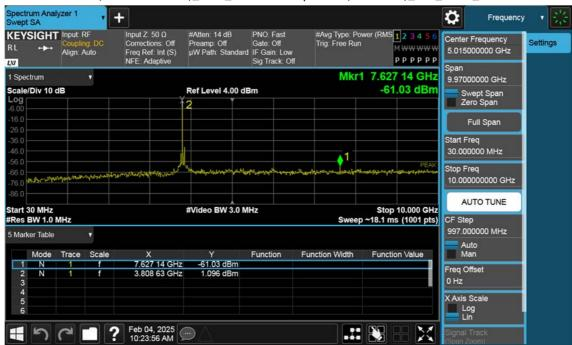
n77(3700~3980 MHz)\_60 M\_Conducted Spurious(30 M-10 G)\_Mid\_BPSK\_1RB
