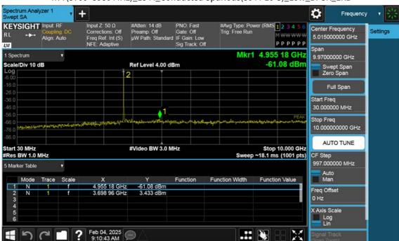
n77(3700~3980 MHz)\_15 M\_Conducted Spurious(30 M-10 G)\_Low\_BPSK\_1RB
