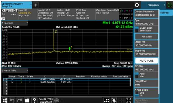
n77(3700~3980 MHz)\_20 M\_Conducted Spurious(30 M-10 G)\_Low\_BPSK\_1RB
