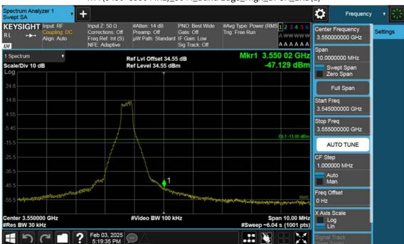
n77(3450~3550 MHz)\_50 M\_Band Edge\_High\_BPSK\_1RB(1)
