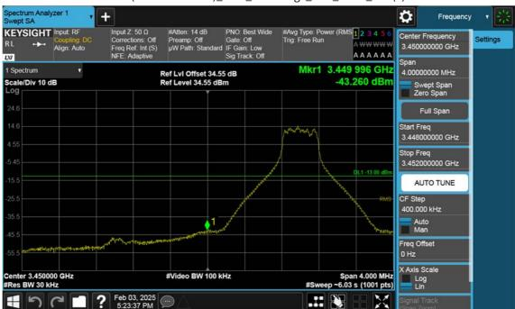
n77(3450~3550 MHz)\_60 M\_Band Edge\_Low\_BPSK\_1RB(1)
