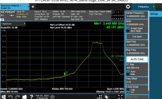
n77(3450~3550 MHz)\_40 M\_Band Edge\_Low\_BPSK\_1RB(1)
