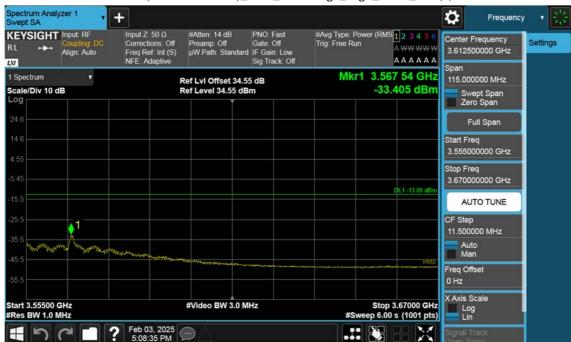
n77(3450~3550 MHz)\_40 M\_Band Edge\_High\_BPSK\_1RB(3)
