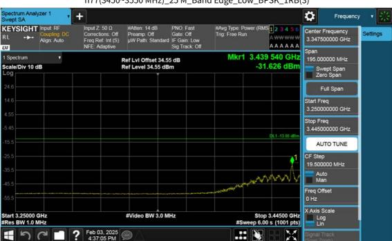
n77(3450~3550 MHz)\_25 M\_Band Edge\_Low\_BPSK\_1RB(3)
