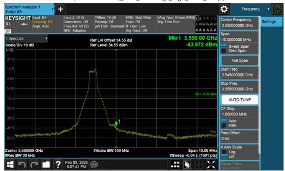
n77(3450~3550 MHz)\_40 M\_Band Edge\_High\_BPSK\_1RB(1)
