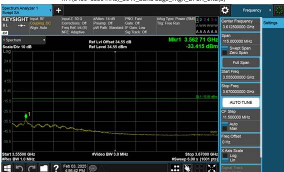
n77(3450~3550 MHz)\_30 M\_Band Edge\_High\_BPSK\_1RB(3)
