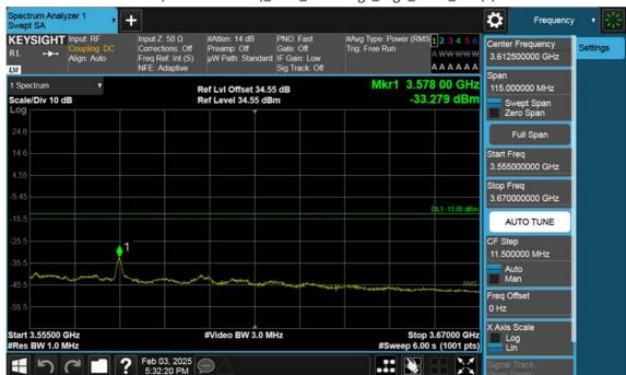
n77(3450~3550 MHz)\_60 M\_Band Edge\_High\_BPSK\_1RB(3)
