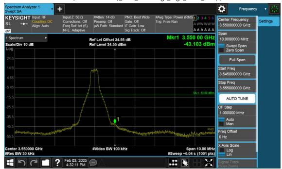
n77(3450~3550 MHz)\_20 M\_Band Edge\_High\_BPSK\_1RB(1)
