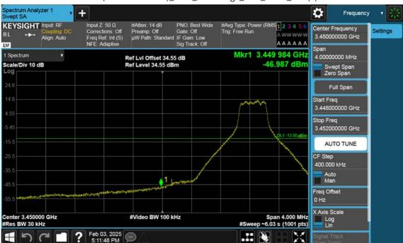
n77(3450~3550 MHz)\_50 M\_Band Edge\_Low\_BPSK\_1RB(1)
