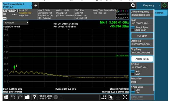
n77(3450~3550 MHz)\_25 M\_Band Edge\_High\_BPSK\_1RB(3)
