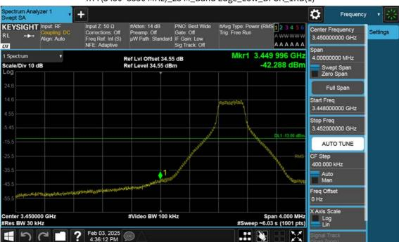
n77(3450~3550 MHz)\_25 M\_Band Edge\_Low\_BPSK\_1RB(1)
